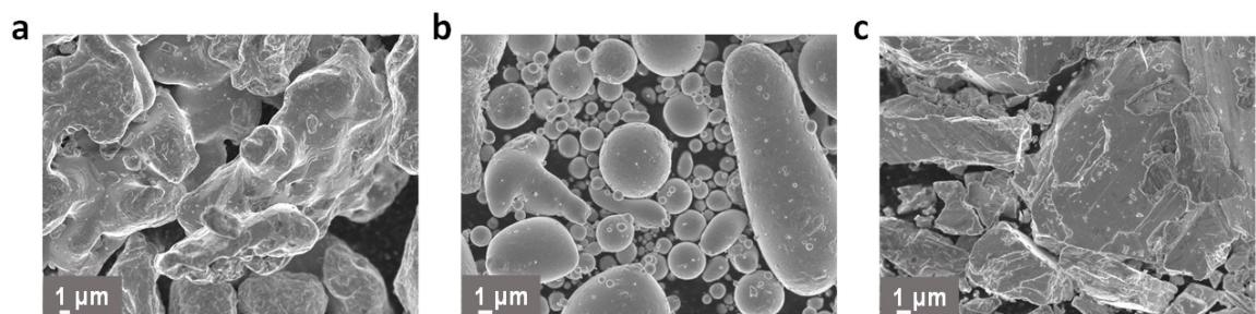
**Figure S1.** Metal powders used as precursor for the rapid solidification process. a) Fe powder. b) Sn powder. c) Sb powder.
