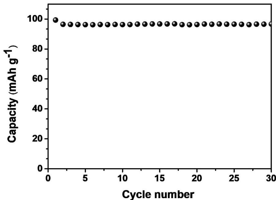
**Figure S12.** Galvanostatic cycling performance of  $\text{NaVPO}_4\text{F}/\text{Na}$  half-cell at a specific current of  $50 \text{ mA g}^{-1}$  in the potential window 2-3.8 vs.  $\text{Na}^+/\text{Na}$ .
