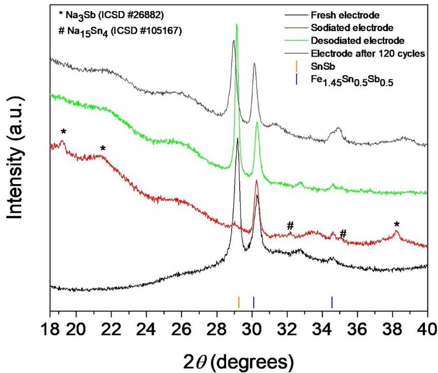
**Figure S11.** *Ex situ* XRD of  $\text{Fe}_{1.0}\text{-SnSb}$  anode at various stages of cycling.
