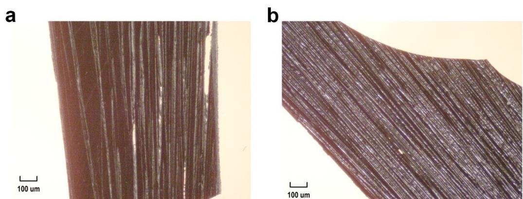
**Figure S2.** Optical microscopy images of the rapidly solidified ribbons of a) SnSb and b)  $\text{Fe}_{1.0}\text{-SnSb}$ .
