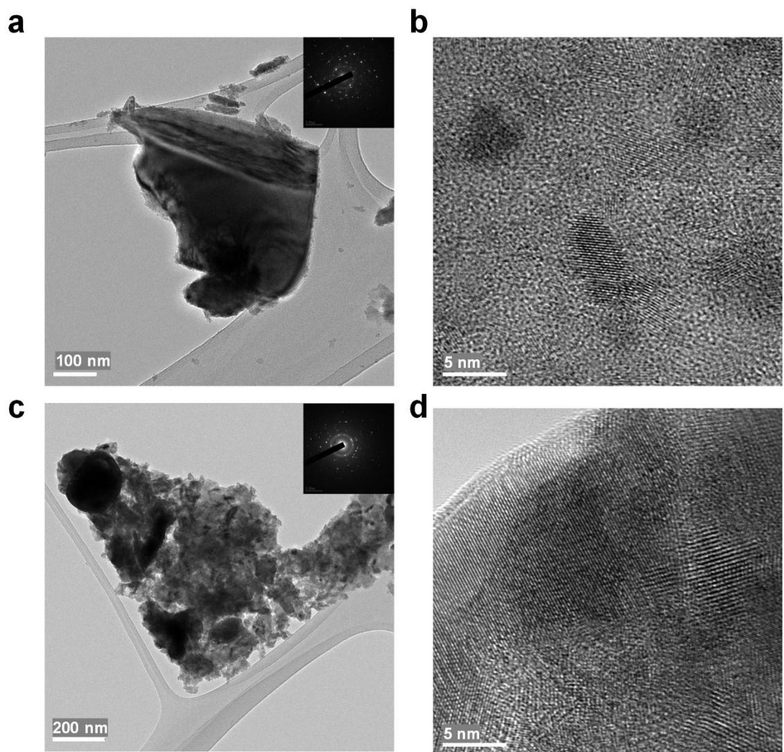
**Figure S9.** HRTEM images of (a, b)  $\text{Fe}_{0.25}\text{-SnSb}$  and (c, d)  $\text{Fe}_{0.5}\text{-SnSb}$  alloys
