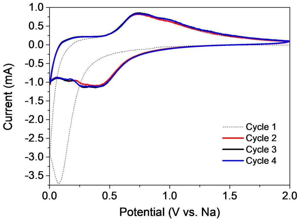
**Figure S6.** Cyclic voltammogram of  $\text{Fe}_{1.0}\text{-SnSb}$  alloy anode.
