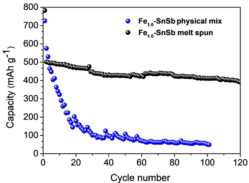
**Figure S8.** Enhanced cycling stability of the rapidly solidified  $\text{Fe}_{1.0}\text{-SnSb}$  alloy against the control sample which is a physical mix of the Fe, Sn and Sb metal powders in the same ratio.
