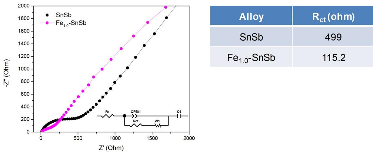
**Figure S7.** Impedance spectra of SnSb and  $\text{Fe}_{1.0}\text{-SnSb}$  anodes.
