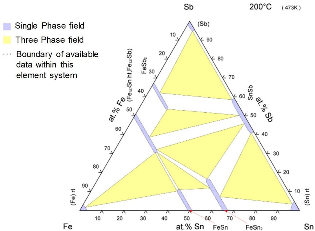
**Figure S4.** Fe-Sb-Sn isothermal section of ternary phase diagram.<sup>1</sup> ©Springer & Material Phases Data System (MPDS), Switzerland & National Institute for Materials Science (NIMS), Japan, 2016.
