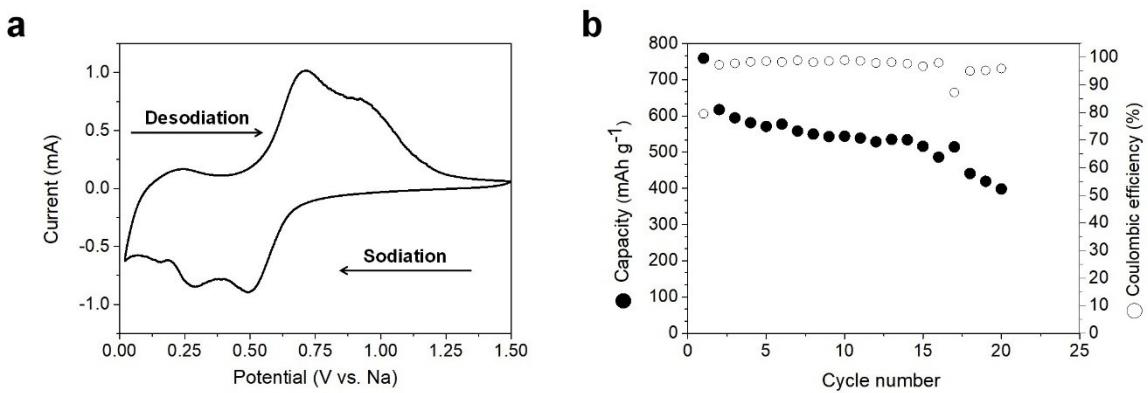
**Figure S3.** Electrochemical performance of SnSb anode. a) Cyclic voltammogram at  $0.1 \text{ mV s}^{-1}$  and b) Galvanostatic charge-discharge test at  $50 \text{ mA g}^{-1}$  in the potential window  $0.005 - 2 \text{ V}$  vs. Na.
