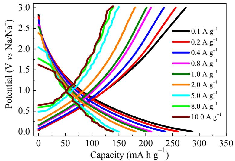
**Figure S13.** Discharge and charge profiles of the 5th cycle at various current densities for well-ordered 3D porous PC.
