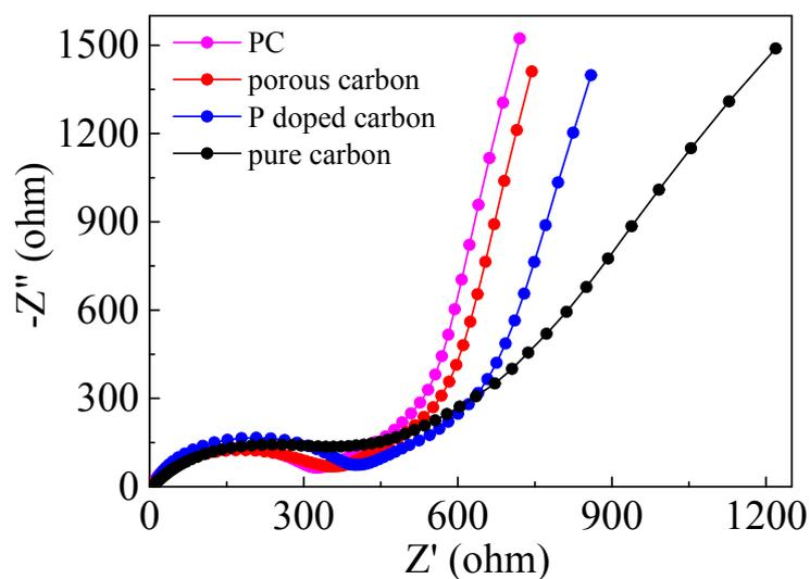
**Figure S6.** Electrochemical impedance spectra of PC, porous carbon, P doped carbon, and pure carbon as electrodes after first cycle in the frequency range from 1 MHz to 100 mHz, respectively.
