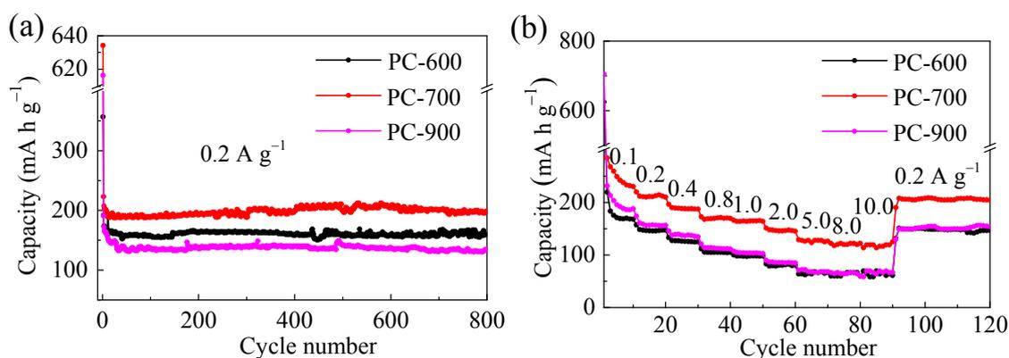
**Figure S14.** (a) Cycle performance at the current density of 0.2 A g<sup>-1</sup> (b) Rate performance in the potential range of 0–3.0 V for PC-600, PC-700 and PC-900.
