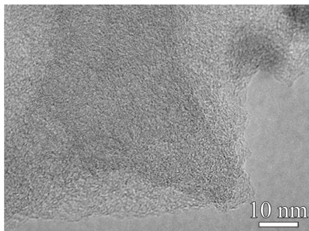
**Figure S5.** HRTEM image of the well-ordered 3D porous PC.
