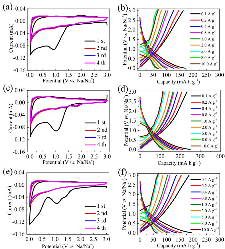
**Figure S12.** First four cyclic voltammetry (CV) curves of (a) PC-600 (c) PC-700 and (e) PC-900 for the first four cycles in the potential range of 0.0–3.0 V vs. Na<sup>+</sup>/Na at a scan rate of 0.2 mV s<sup>-1</sup>; galvanostatic charge and discharge profiles of (b) PC-600 (d) PC-700 and (f) PC-900 at 0.2 A g<sup>-1</sup>.
