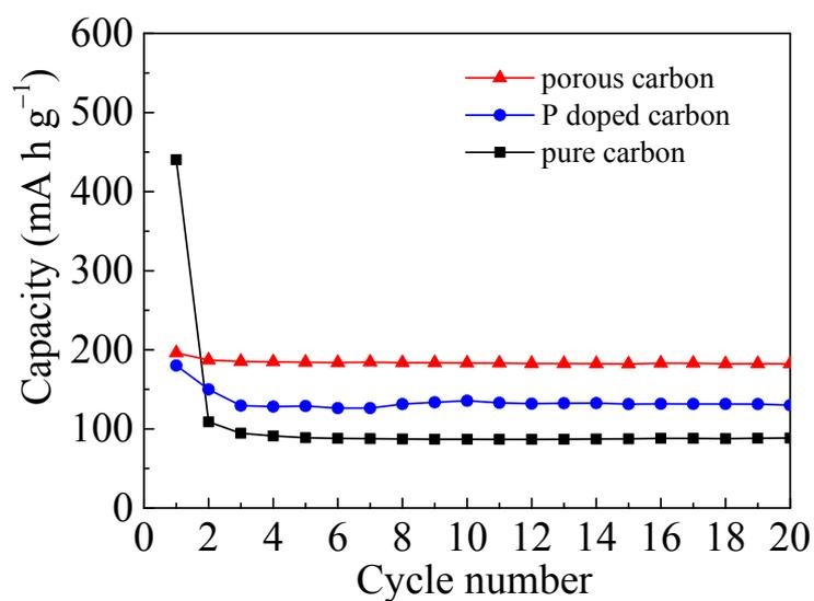
**Figure S7.** Cycling performance of porous carbon, P doped carbon and pure carbon at a current density of  $0.2 \text{ A g}^{-1}$ .
