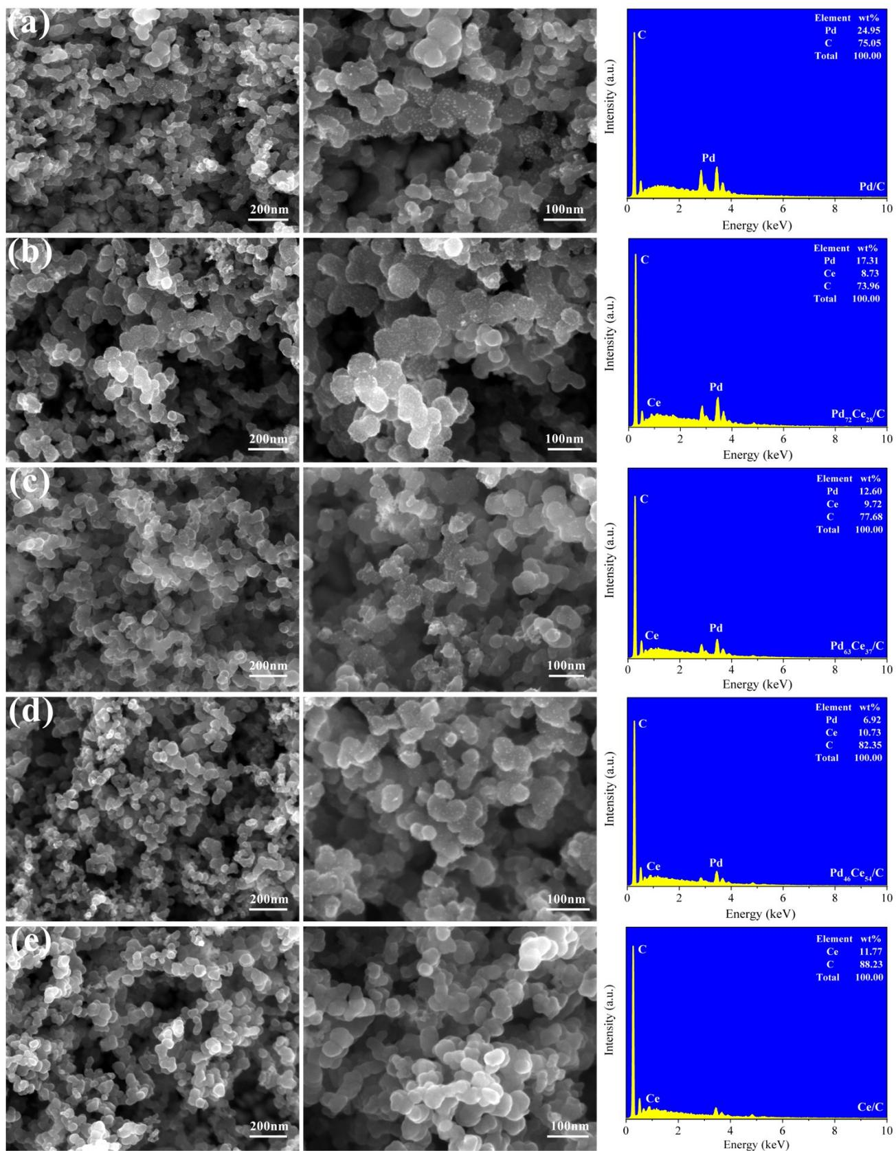
**Figure S1.** SEM images with different magnifications and the corresponding EDS of the various PdCe/C catalysts. (a) Pd/C, (b) Pd<sub>72</sub>Ce<sub>28</sub>/C, (c) Pd<sub>63</sub>Ce<sub>37</sub>/C, (d) Pd<sub>46</sub>Ce<sub>54</sub>/C and (e) Ce/C.
