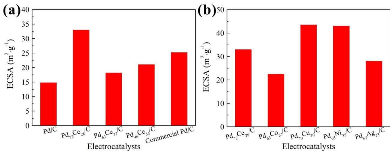
**Figure S5.** (a) ECSA of  $\text{Pd}_{72}\text{Ce}_{28}/\text{C}$  catalyst compared to other PdCe/C catalysts and commercial Pd/C catalyst. (b) ECSA of PdM/C (M = Co, Cu, Ni, Ag) catalysts and  $\text{Pd}_{72}\text{Ce}_{28}/\text{C}$  catalyst. All ECSAs are obtained by integrating the reduction peak area of Pd in the CV curves.
