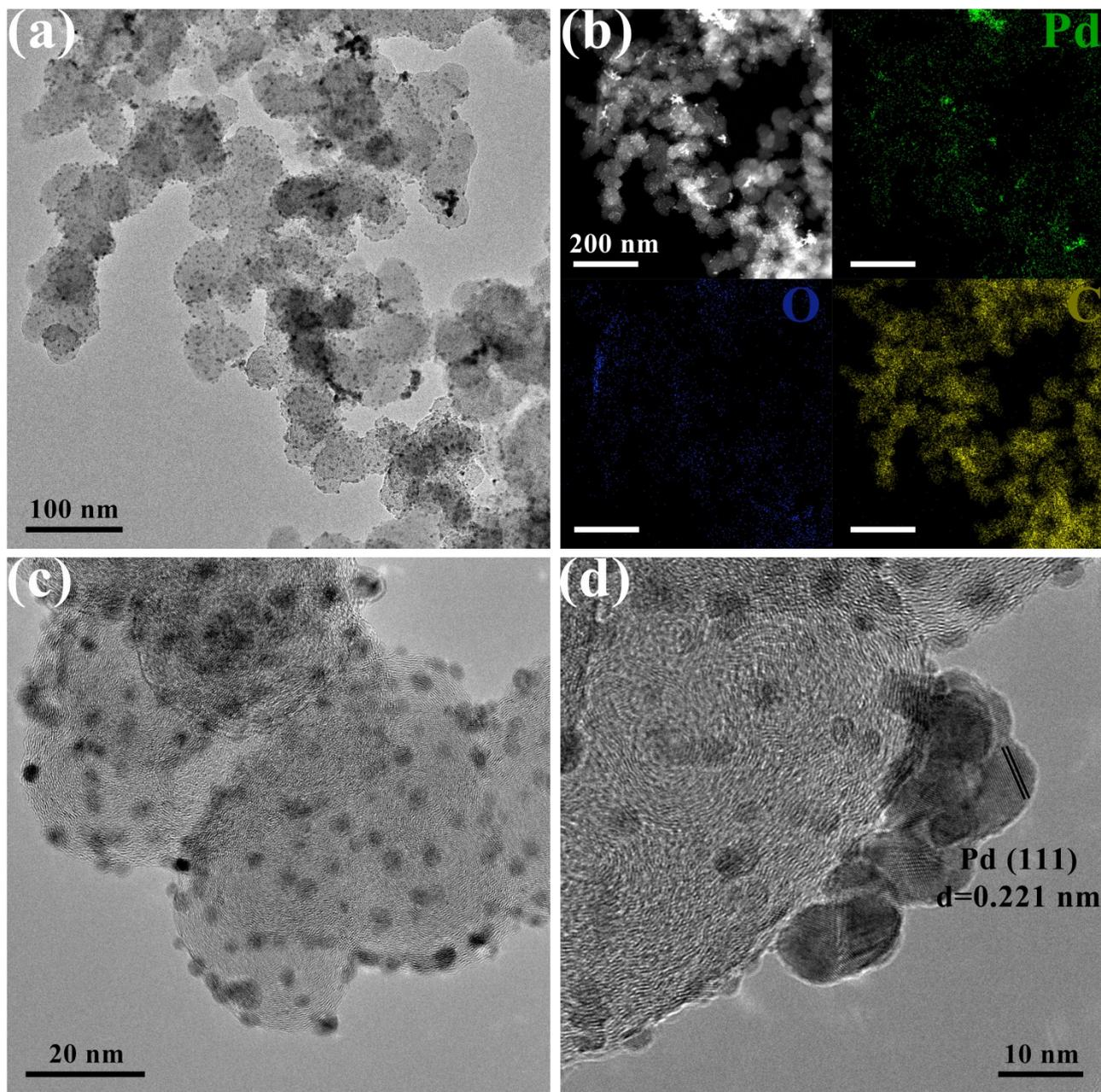
**Figure S2.** TEM images with different magnifications and the corresponding EDX of Pd/C catalyst. (a) TEM image of Pd/C catalyst. (b) HAADF image and EDX elemental mapping of Pd/C catalyst. (c) TEM image of the carbon supported Pd nanoparticles. (d) The high-resolution TEM image of the carbon supported Pd nanoparticles. The interplanar spacing of the carbon supported Pd nanoparticles could be marked in the image.
