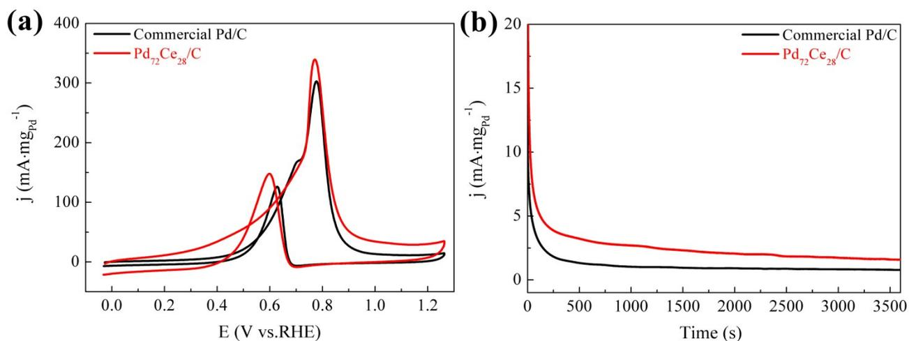
**Figure S3.** Electrochemical performance of Pd<sub>72</sub>Ce<sub>28</sub>/C catalysts for the methanol oxidation reaction. (a) CV curves of Pd<sub>72</sub>Ce<sub>28</sub>/C and the commercial Pd/C catalysts at the scan rate of 50 mV·s<sup>-1</sup> in N<sub>2</sub>-saturated 1 M KOH with 1 M CH<sub>3</sub>OH solution normalized by the mass of Pd. (b) CA curves at 0.45 V in N<sub>2</sub>-saturated 1 M KOH with 1 M CH<sub>3</sub>OH solution.
