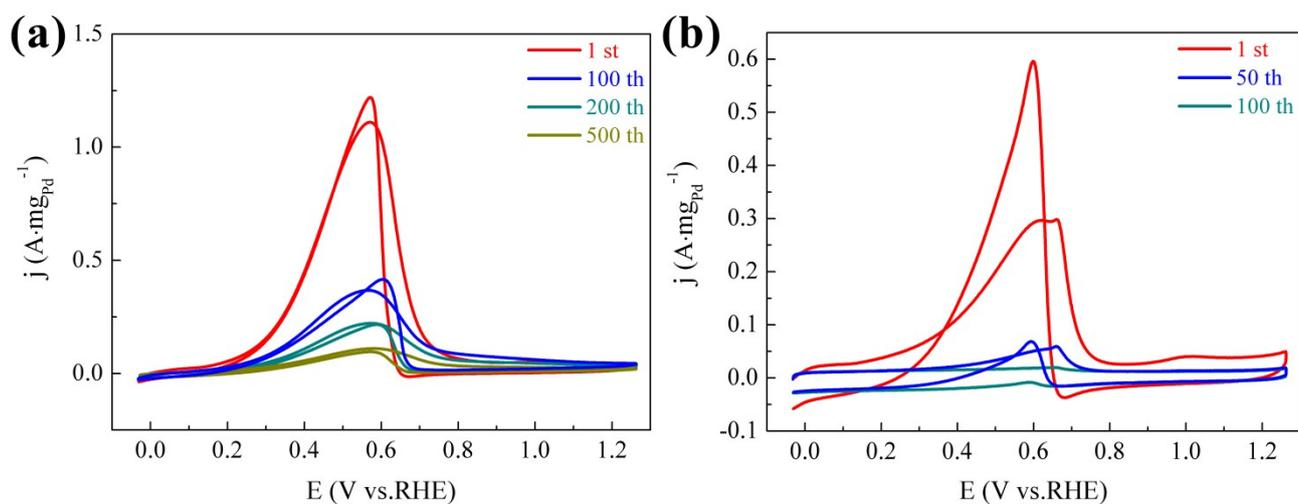
**Figure S4.** Cycle stability of Pd<sub>72</sub>Ce<sub>28</sub>/C catalysts for the formate oxidation reaction. CV curves at different cycle times of (a) Pd<sub>72</sub>Ce<sub>28</sub>/C catalyst and (b) the commercial Pd/C catalyst at the scan rate of 50 mV·s<sup>-1</sup> in N<sub>2</sub>-saturated 1 M KOH with 1 M CH<sub>3</sub>OH solution normalized by the mass of Pd.
