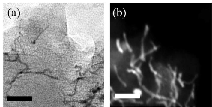
Figure S2. (a)TEM image and (b) HAADF-STEM image of PtNi NWs. The scale bar is 20 nm.
