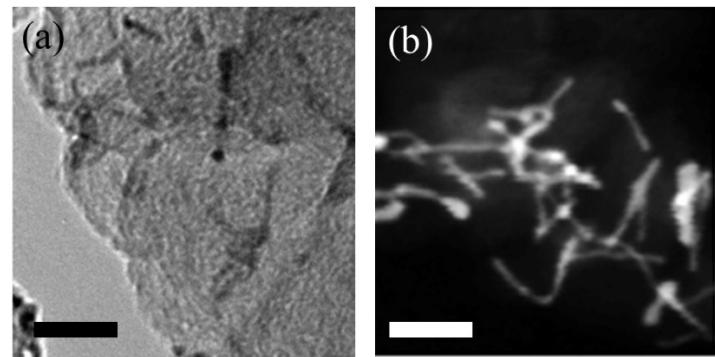
Figure S4. (a)TEM image and (b) HAADF-STEM image of D-Ar-Pt NWs. The scale bar is 20 nm
