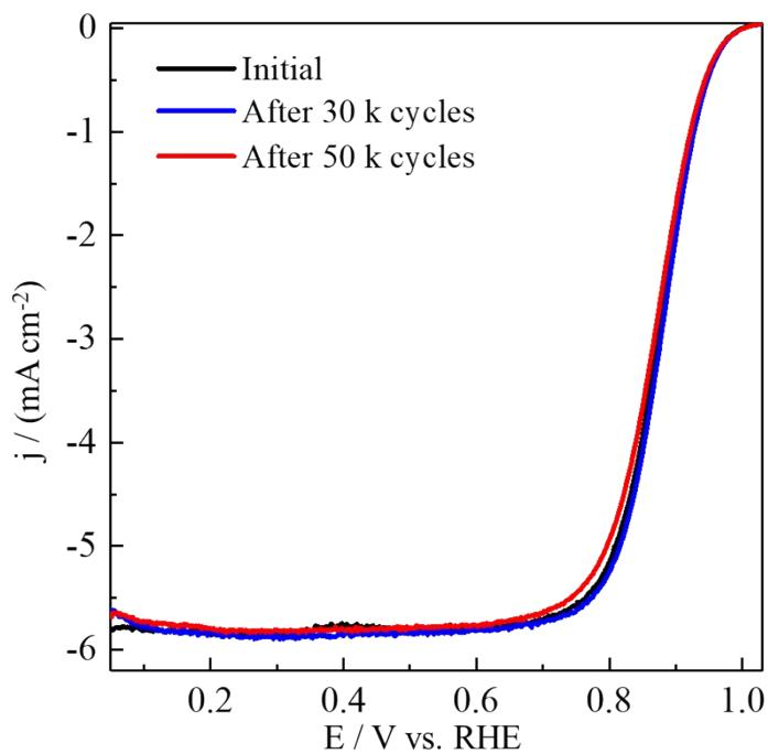
Figure S8. Polarization curves of Pt NWs in oxygen saturated 0.1 HClO<sub>4</sub> before and after 30 000 and 50 000 potential cycles between 0.6 and 1.0 V versus RHE.
