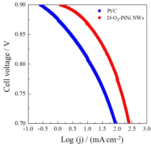
Figure S7. Tafel plots of Pt/C and D-O<sub>2</sub>-Pt NWs of MEA for H<sub>2</sub>-air fuel cells.
