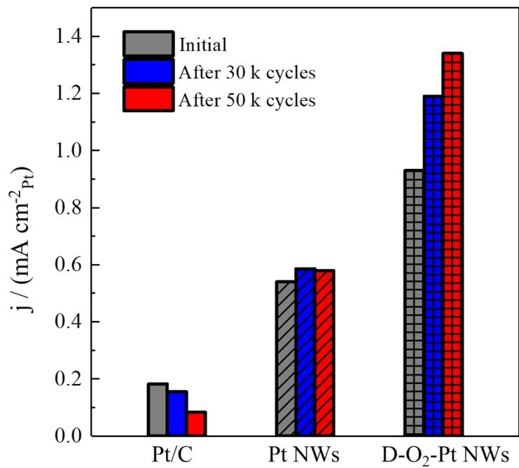
Figure S11. Bar chart of specific activity of Pt/C, Pt NWs and D-O<sub>2</sub>-Pt NWs before and after stability test.
