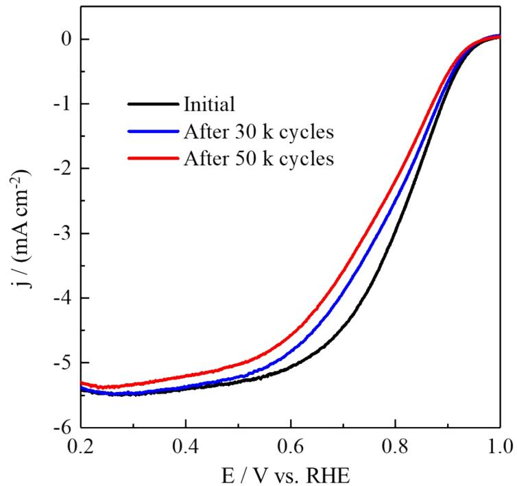
Figure S9. Polarization curves of Pt/C in oxygen saturated 0.1 HClO<sub>4</sub> before and after 30 000 and 50 000 potential cycles between 0.6 and 1.0 V versus RHE. The insert image is the HAADF-STEM image of Pt/C after stability test.
