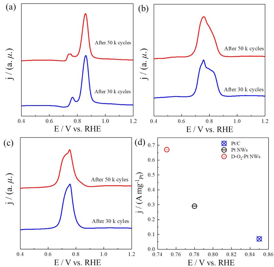
Figure S12. CO stripping curves on Pt/C (a), Pt NWs (b) and D-O<sub>2</sub>-Pt NWs (c) after 30 k and 50 k cycles. (d) The relationship between mass activity at 0.9 V and density of defects, estimated by average CO oxidation potential after 50 k cycles.
