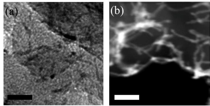
Figure S1. (a)TEM image and (b) HAADF-STEM image of Pt NWs. The scale bar is 20 nm.
