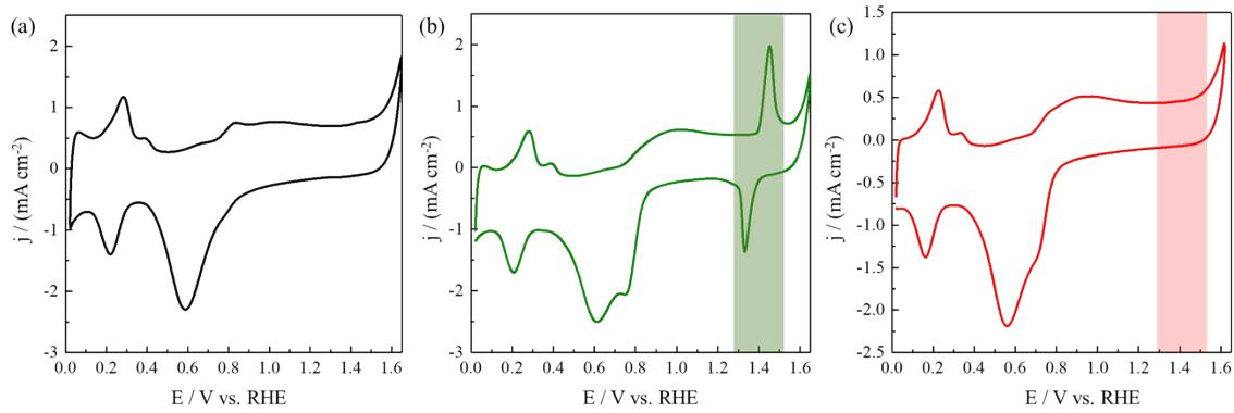
Figure S5. (a) The CV curve of 1<sup>st</sup> cycle of D-Ar-Pt NWs in oxygen saturated 0.1 M NaOH. (b) The CV curve of 50<sup>th</sup> cycle of D-Ar-Pt NWs in oxygen saturated 0.1 M NaOH. (c) The CV curve of 50<sup>th</sup> cycle of D-O<sub>2</sub>-Pt NWs in oxygen saturated 0.1 M NaOH.
