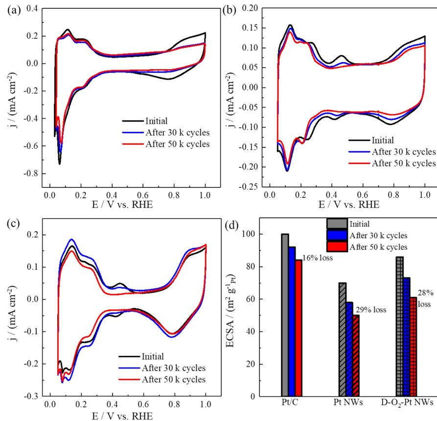
Figure S10. CV of Pt/C (a), Pt NWs (b) and D-O<sub>2</sub>-Pt NWs (c) before and after stability test in Ar saturated 0.1 M HClO<sub>4</sub>. (d) Electrochemical surface area of Pt/C, Pt NWs and D-Pt NWs before and after stability test.
