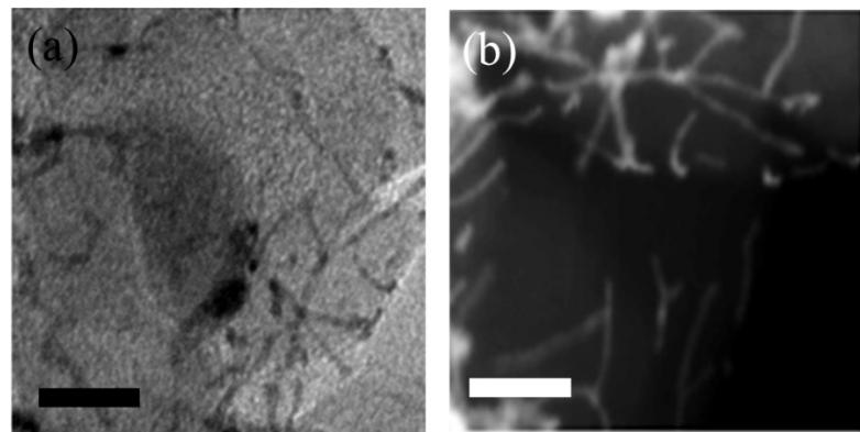
Figure S3. (a)TEM image and (b) HAADF-STEM image of D-O<sub>2</sub>-Pt NWs. The scale bar is 20 nm
