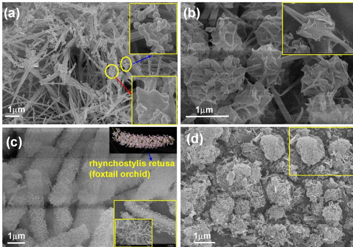
**Fig. S2.** HR-SEM images of  $\alpha$ -NiMoO<sub>4</sub> nanostructures at different amounts of TPAOH (a) 10  $\mu$ l (b) 30  $\mu$ l (c) 50  $\mu$ l (d) 70  $\mu$ l, which clearly shows the influence of TPAOH on the morphologies of  $\alpha$ -NiMoO<sub>4</sub>.
