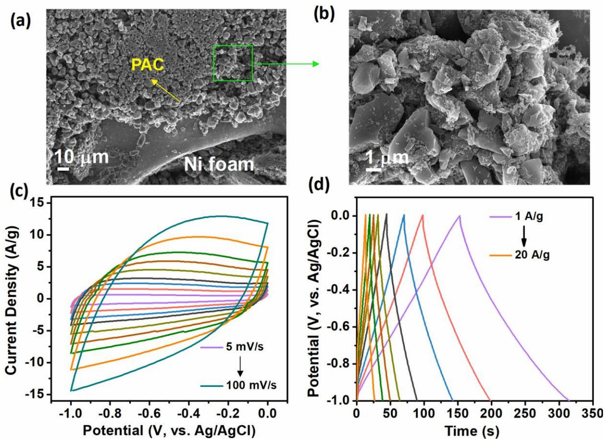
**Fig. S5.** (a) and (b) low and high magnification SEM images of APC, respectively, (c) CV curves of APC at different scan rates and (d) GCD curves of the APC at different current densities.
