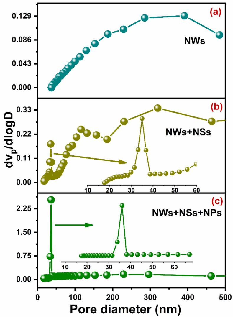
**Fig. S3.** Pore size distribution curves of the  $\alpha$ -NiMoO<sub>4</sub> (a) NWs, (b) NWs+NSs, and (c) NWs+NSs+NPs)
