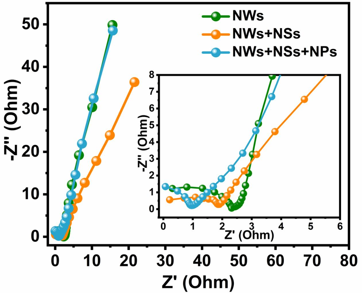
**Fig. S4.** EIS spectra of  $\alpha$ -NiMoO<sub>4</sub> NWs, NWs+NSs, NWS+NSs+NPs samples measured in three-electrode system.
