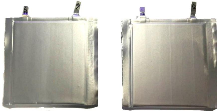
**Fig. S9** The optical photograph of  $\text{LiNi}_{0.5}\text{Co}_{0.2}\text{Mn}_{0.3}\text{O}_2/\text{GSC-graphite}$  full batteries.
