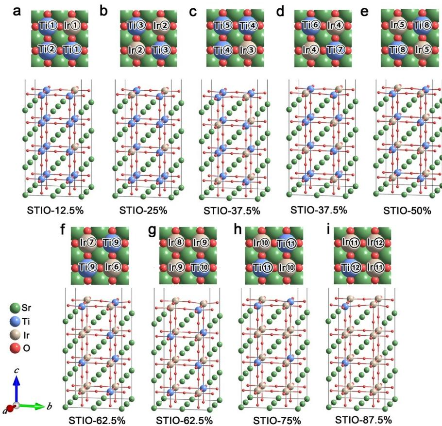
**Fig. S2.** Structural models and the corresponding top views for the (001) planes of **a**, STIO-12.5%, **b**, STIO-25%, **c**, **d**, STIO-37.5%, **e**, STIO-50%, **f**, **g**, STIO-62.5%, **h**, STIO-75%, **i**, STIO-87.5%. The titanium and iridium sites with different atomic environments are marked on the top views, and the corresponding free energy for the intermediates are shown in Table S3 and Table S4, respectively.
