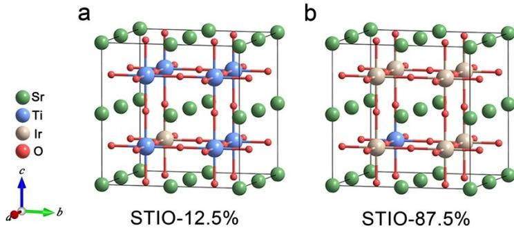
**Fig. S1.** The structural models of **a**, STIO-12.5%, **b**, STIO-87.5%. The models with remain iridium content are shown in Table S1, because of their various possible doping configurations.
