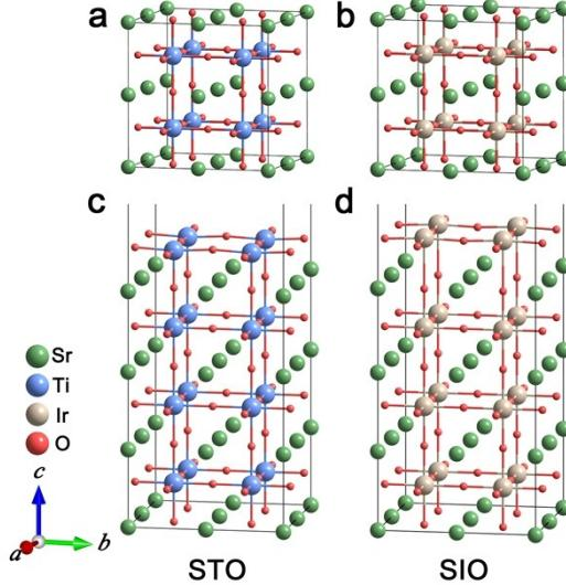
**Fig. S3.** **a, b,**  $\text{SrTiO}_3$  and  $\text{SrIrO}_3$  supercells with the cubic structure. **c,** The slab model for the (001) plane of the STO. **d,** The slab model for the (001) plane of the SIO. The free energy for the intermediates on Ti/Ir sites are shown in Table S3 and Table S4, respectively.
