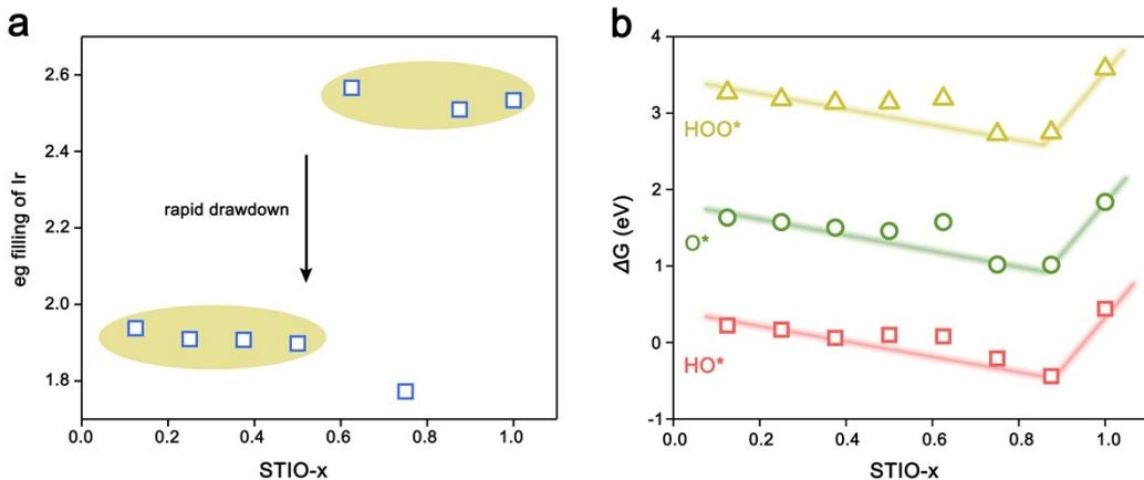
**Fig. S6.** (a) The  $e_g$ -filling and (b) adsorption free energy of HOO\*, O\* and HO\* for the most active iridium sites plotted as a function of the iridium content of STIO.
