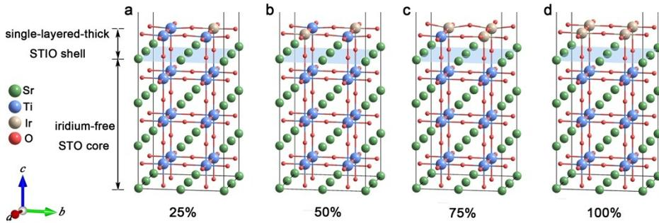
**Fig. S10.** Structural models of the novel core/shell-type models with different iridium content in the STIO shell. The titanium and iridium sites with different atomic environments are marked on the top views in Fig. 5, inset in main text, and the corresponding free energy for the intermediates are shown in Table S8.
