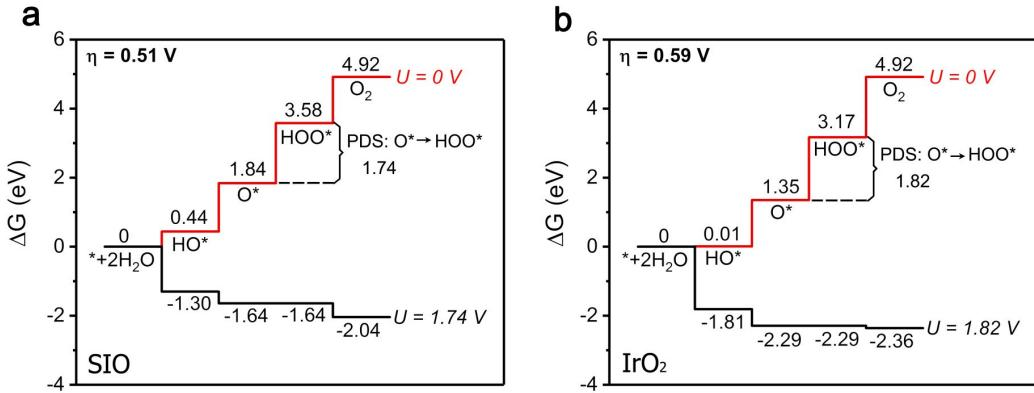
**Fig. S4.** The Gibbs free energy diagram for (a) SIO and (b)  $\text{IrO}_2$ , respectively. The data for  $\text{IrO}_2$  are taken from our previous study. Ref. [1]. The overpotential of perovskite SIO (0.51 V) are lower than that of rutile  $\text{IrO}_2$  (0.59 V) because of the weaker bonding energy of the intermediates on the SIO.
