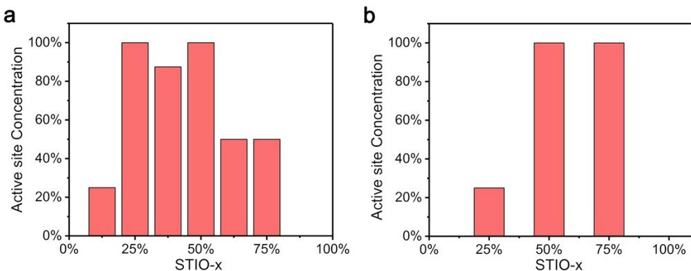
**Fig. S11.** The active site concentration as a function of the iridium content in (a) STIO models and (b) STIO-shell of the core-shell models. The active site concentration is the ratio of the number of the active sites (the overpotential of the site is similar or lower than that on  $\text{IrO}_2$ ) and the number of all catalytic sites.
