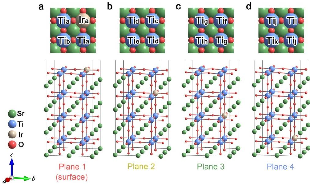
**Fig. S7.** Structural models and the corresponding top views of STO slab models with iridium doped in **a**, Plane 1 (surface), **b**, Plane 2, **c**, Plane 3, **d**, Plane 4. The titanium and iridium sites with different atomic environments are marked on the top views, and the corresponding free energy for the intermediates are shown in Table S6.
