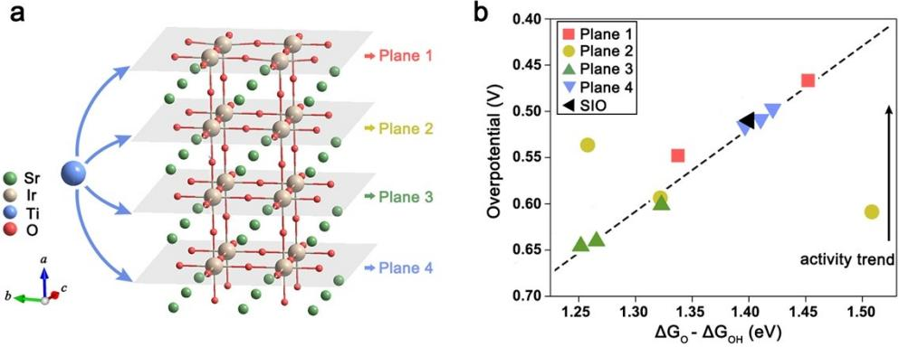
**Fig. S9.** Schematic of an titanium atom substituting iridium atom on different planes of SIO model. The planes 1-4 represent possible doped planes of SIO model. (b) Negative theoretical overpotential as a function of  $\Delta G_O - \Delta G_{OH}$  for the surface iridium sites in the SIO model with iridium doped in plane 1 (red), plane 2 (yellow), plane 3 (green), plane 4 (blue), respectively. The overpotential (black) for the surface titanium site in SIO is also shown.
