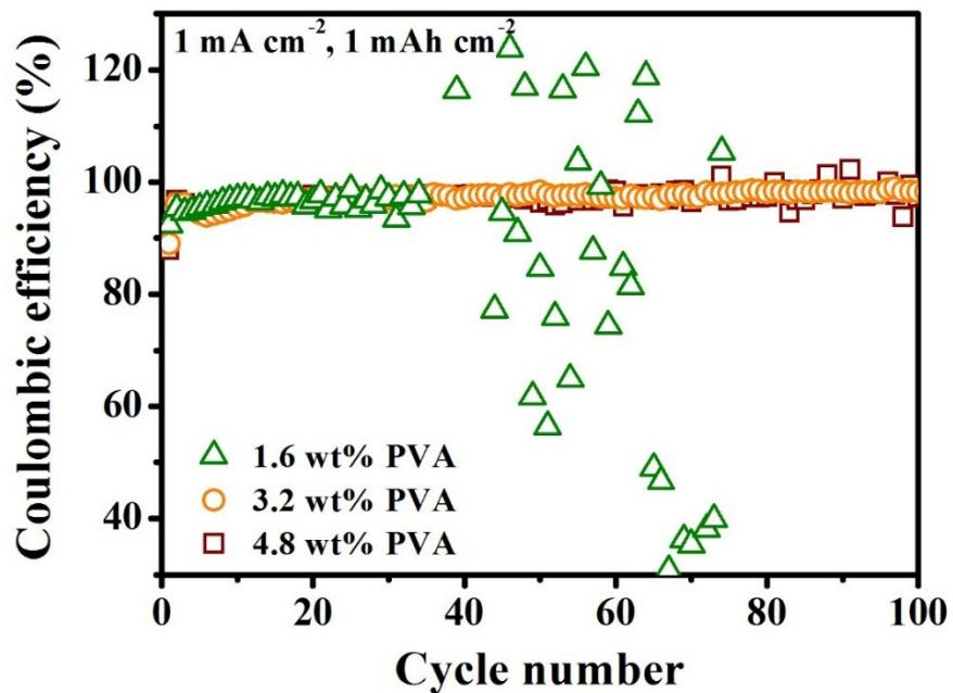
**Fig. S14** Coulombic efficiency of Zn-MOF/PVA films with different PVA content.
