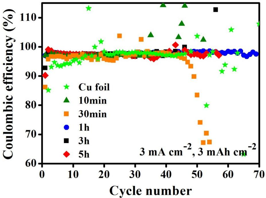
**Fig. S12** The coulombic efficiency of the electrode under the protection of Zn-MOF film obtained at different growth times.
