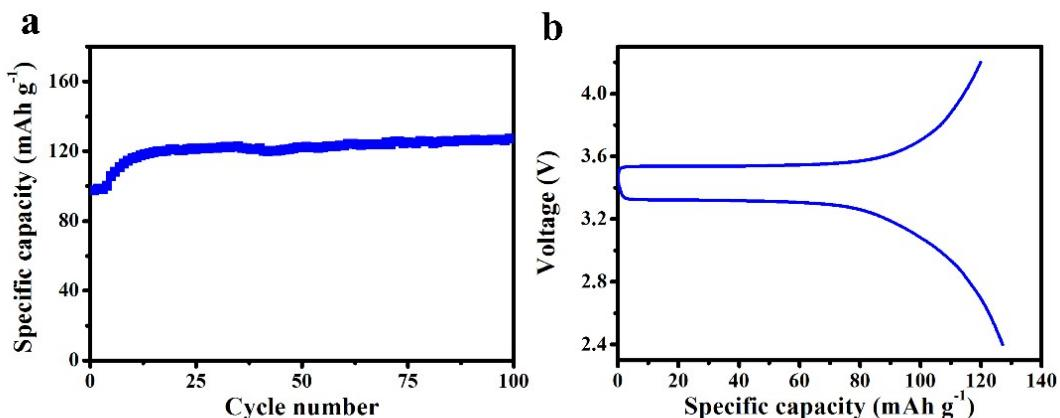
**Fig. S15** LiFePO<sub>4</sub> and Li foil assembly batteries (a)Cycle performance of the battery at 1C; (b) Charge-discharge voltage curve after 100 cycles.
