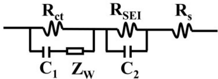
**Fig.S11** Impedance equivalent circuit model.
