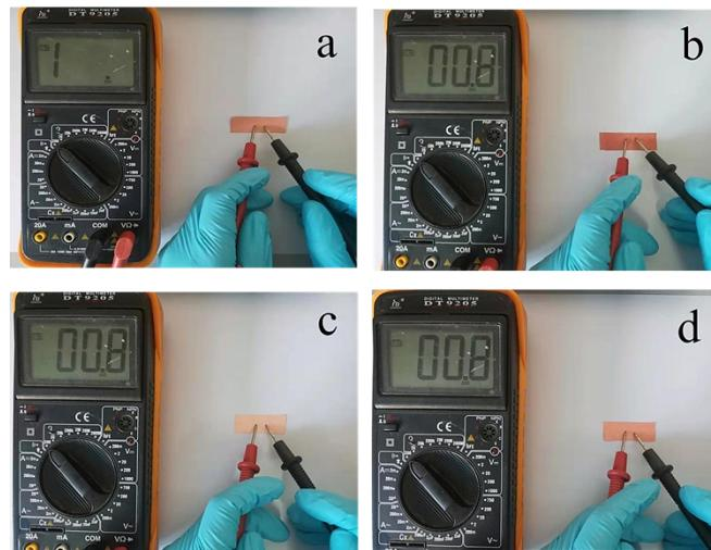
**Fig. S3** Apparent resistance of samples (a)Cu@Zn-MOF side (b) Back of Cu@Zn-MOF; (c) Rough (d) Smooth side of Cu foil.
