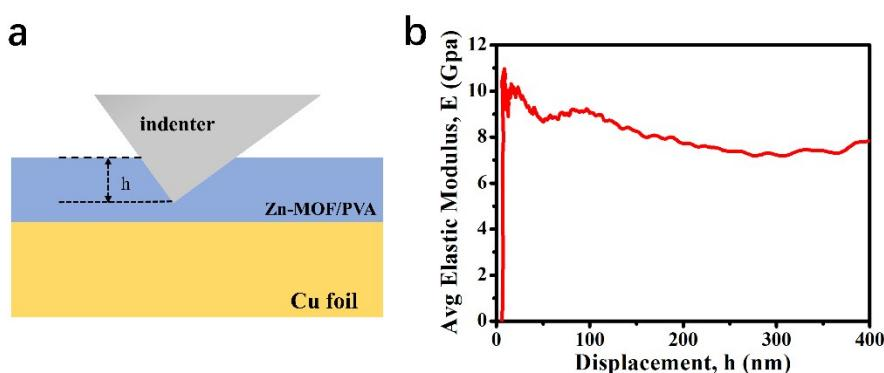
**Fig. S7** (a) schematic diagram of nanoindentation test (b) shows the curve of average elastic modulus
