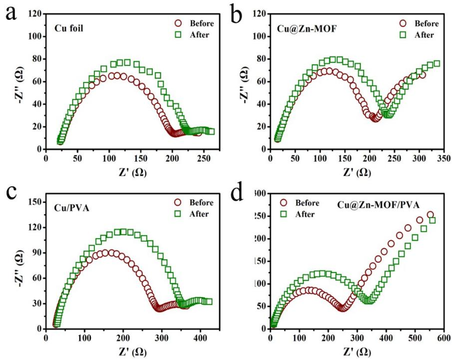
**Fig. S8** Impedance change before and after time-current test (a) Cu foil; (b) Cu@Zn-MOF; (c) Cu/PVA; (d) Cu@Zn-MOF/PVA.
