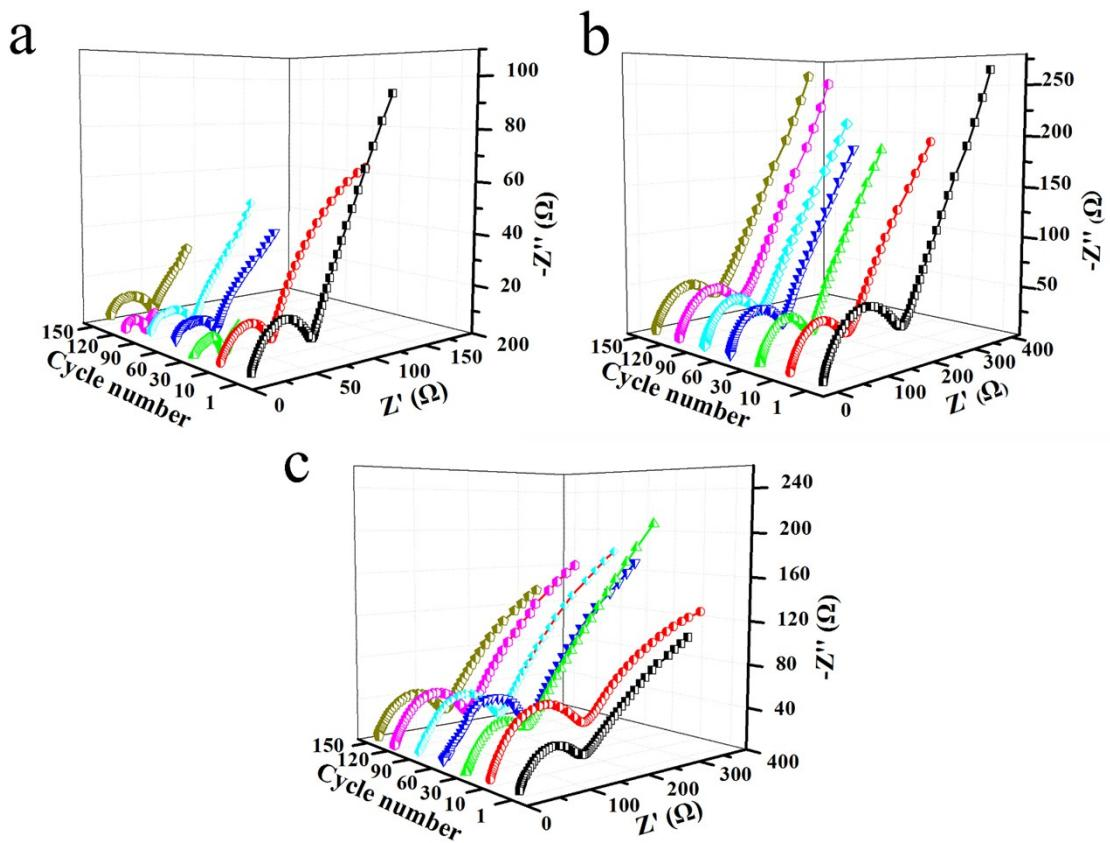
**Fig. S10** The electrochemical impedance at different cycle times (a) Cu foil; (b) Cu@Zn-MOF; (c) Cu/PVA;
