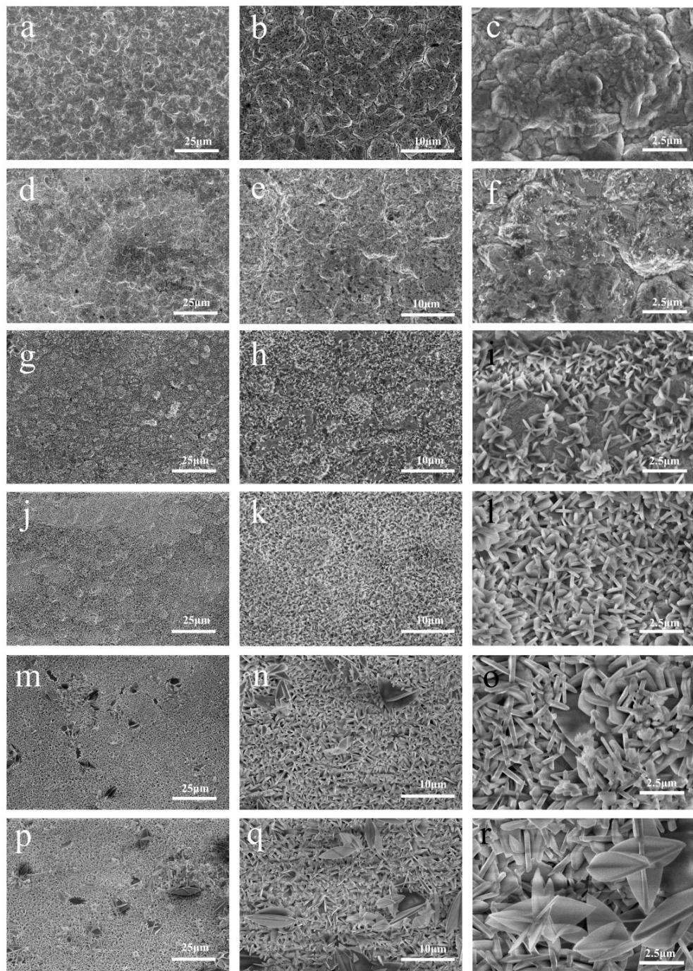
**Fig. S5** Top-view SEM images of the Zn-MOF film on Cu foil with different crystallization time (a) (b) (c) 0min, (d) (e) (f) 10 min, (g) (h) (i) 30 min, (g) (k) (l) 1 h, (m) (n) (o) 3 h, (p) (q) (r) 5 h.
