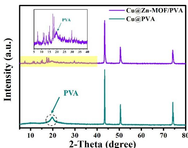
**Fig. S1** The XRD patterns of Cu@Zn-MOF/PVA and Cu@PVA
