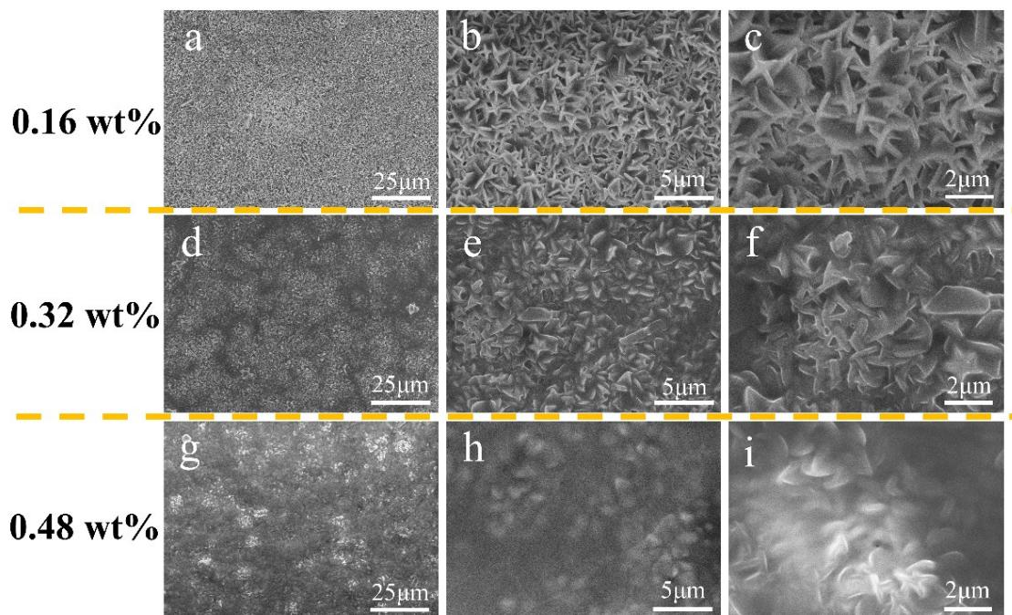
**Fig. S6** Top-view SEM images of the Zn-MOF/PVA film on Cu foil with different content of PVA (a) (b) (c) 0.16%, (d) (e) (f) 0.32%, (g) (h) (i) 0.48% .
