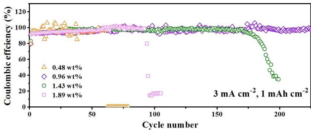
**Fig. S13** Coulombic efficiency of PVA with different lithium salt contents.
