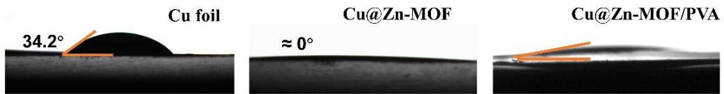
**Fig. S2** Contact angles of LiTFSI-DOL/DME electrolyte on the Cu foil、Cu@Zn-MOF and Cu@Zn-MOF/PVA.
