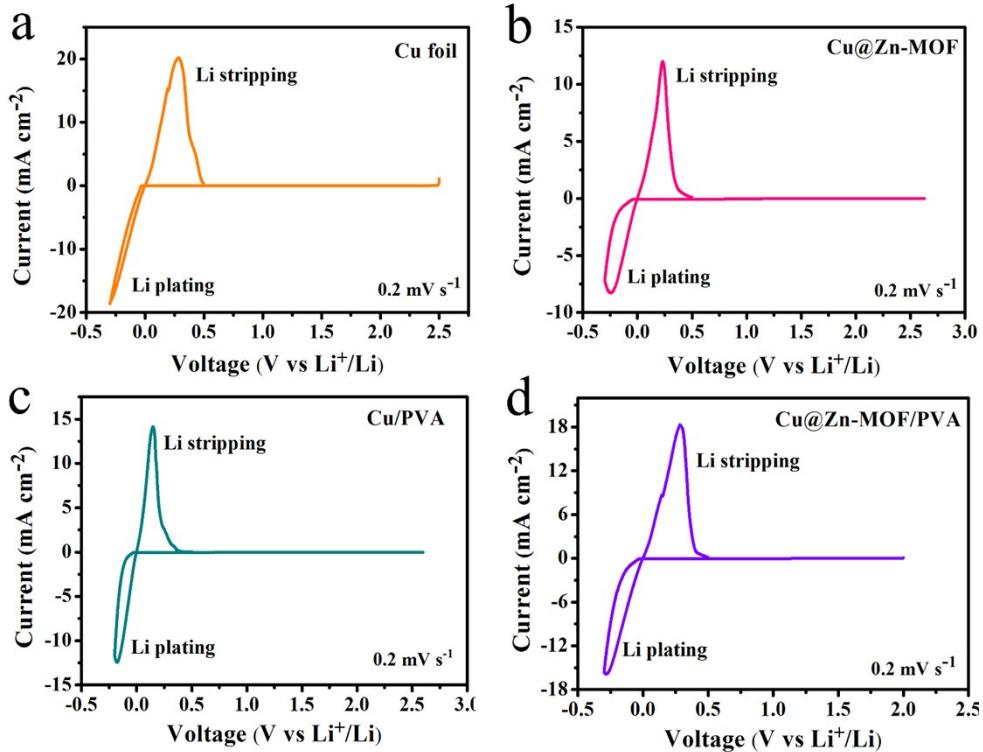
**Fig. S9** Cyclic voltammetry curve of artificial SEI film (a) Cu foil; (b) Cu@Zn-MOF; (c) Cu/PVA; (d) Cu@Zn-MOF/PVA.
