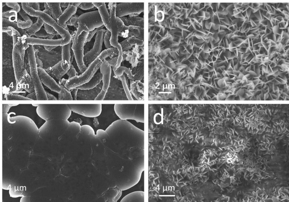
**Fig. S16** Top-view SEM images of Li plating/stripping after first cycles on (a) Cu foil, (b) Cu@Zn-MOF,(c) Cu@PVA,(d) Cu@Zn-MOF/PVA with  $1 \text{ mA cm}^{-2}$ ,  $1 \text{ mAh cm}^{-2}$ .
