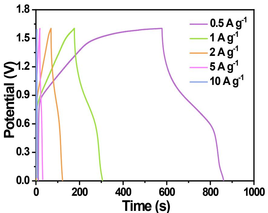
**Fig. S13.** Galvanostatic charge/discharge curves of the PPD-BC//Ni(OH)<sub>2</sub> ASC at various current densities from 0.5 to 10 A g<sup>-1</sup>.
