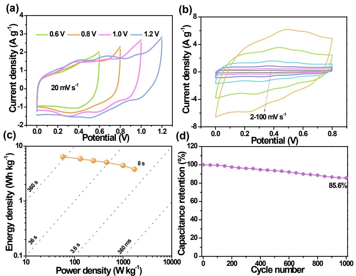
**Fig. S14.** Electrochemical performance of the PPD-BC//PPD-BC symmetric supercapacitor in 1 M H<sub>2</sub>SO<sub>4</sub> electrolyte. (a) CV curves in various operating voltage. (b) CV curves at different scan rates. (c) Ragone plots. (d) Cycling stability at 50 mV s<sup>-1</sup>.
