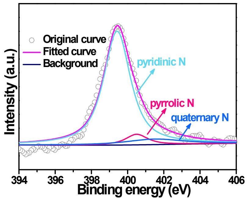
**Fig. S6.** High-resolution N 1s spectra of the PPD-BC.
