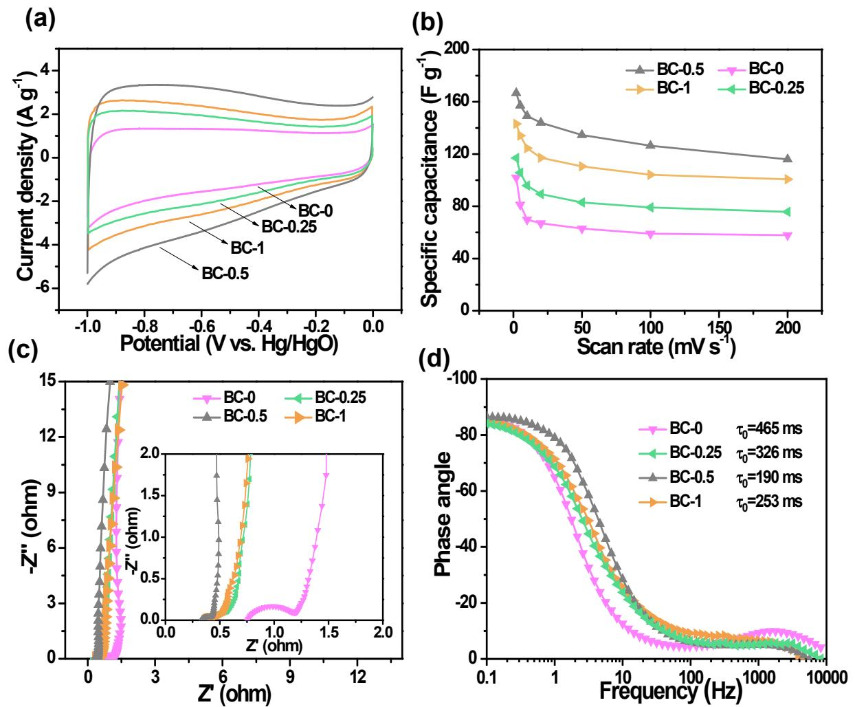
**Fig. S7.** Electrochemical performance of BC- $x$  ( $x=0, 0.25, 0.5, 1$ ). (a) CV curves at  $20 \text{ mV s}^{-1}$ . (b) Specific capacitance as a function of scan rate. (c) Nyquist plots. (d) Bode plots
