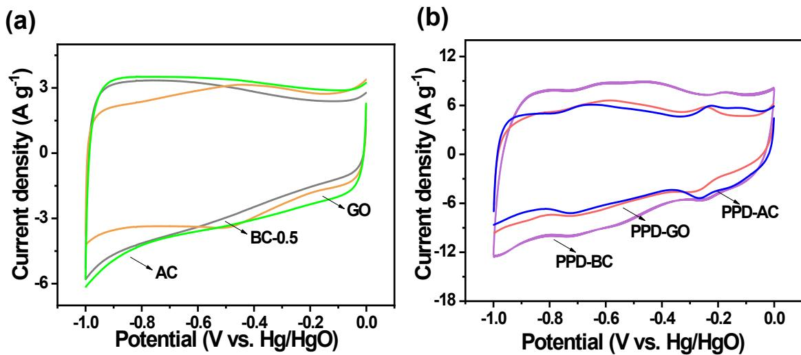
**Fig. S9.** (a) CV curves of the AC, GO, and BC-0.5 at  $20 \text{ mV s}^{-1}$  (b) CV curves of the PPD-AC, PPD-GO, and PPD-BC at  $20 \text{ mV s}^{-1}$ .
