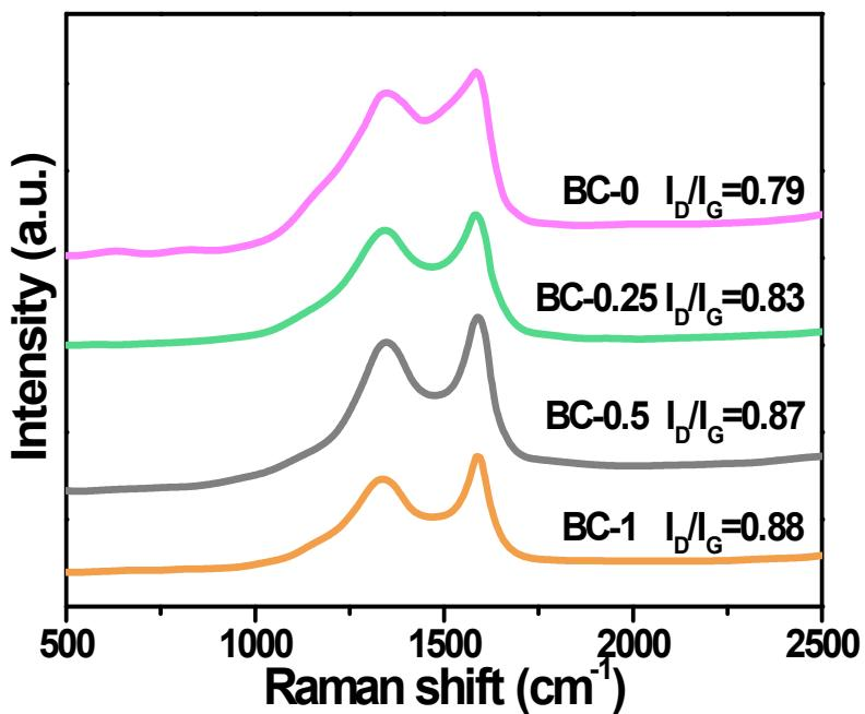
**Fig. S4.** Raman spectra of BC-x (x=0, 0.25, 0.5, 1).
