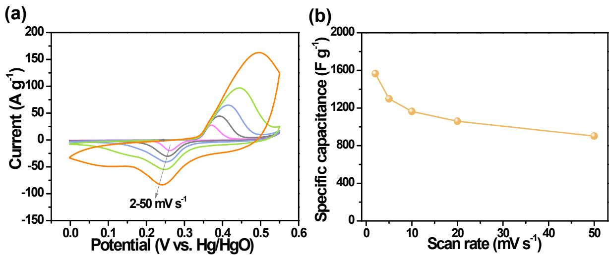
**Fig. S12.** Electrochemical performance of  $\text{Ni(OH)}_2$ . (a) CV curves at different scan rates from 2 to 50  $\text{mV s}^{-1}$ . (b) Specific capacitance at different scan rates from 2 to 50  $\text{mV s}^{-1}$ .
