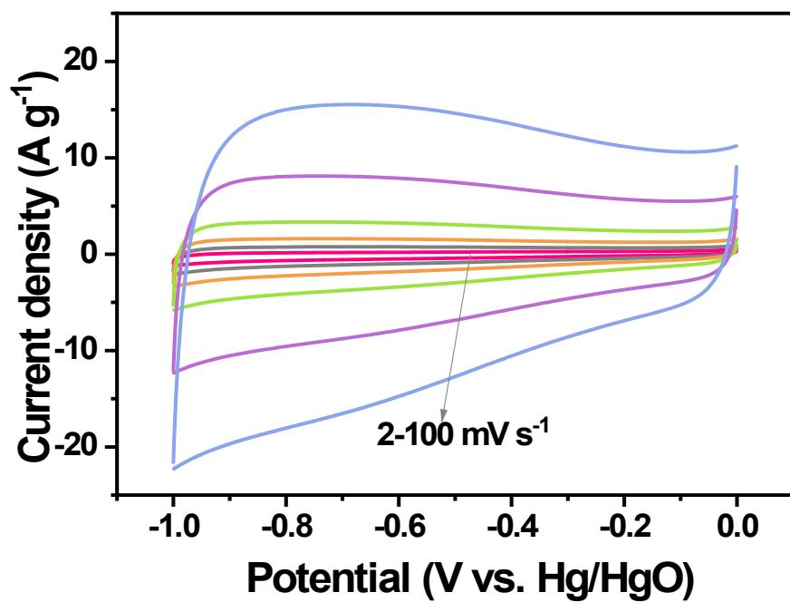
**Fig. S8.** CV curves of the BC-0.5 at the scan rates from 2 to 100  $\text{mV s}^{-1}$
