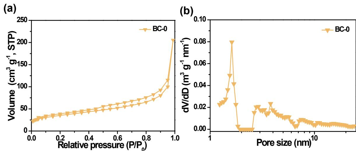
**Fig. S2.** (a, b) Nitrogen adsorption-desorption isotherms and relative pore size distributions of BC-0.
