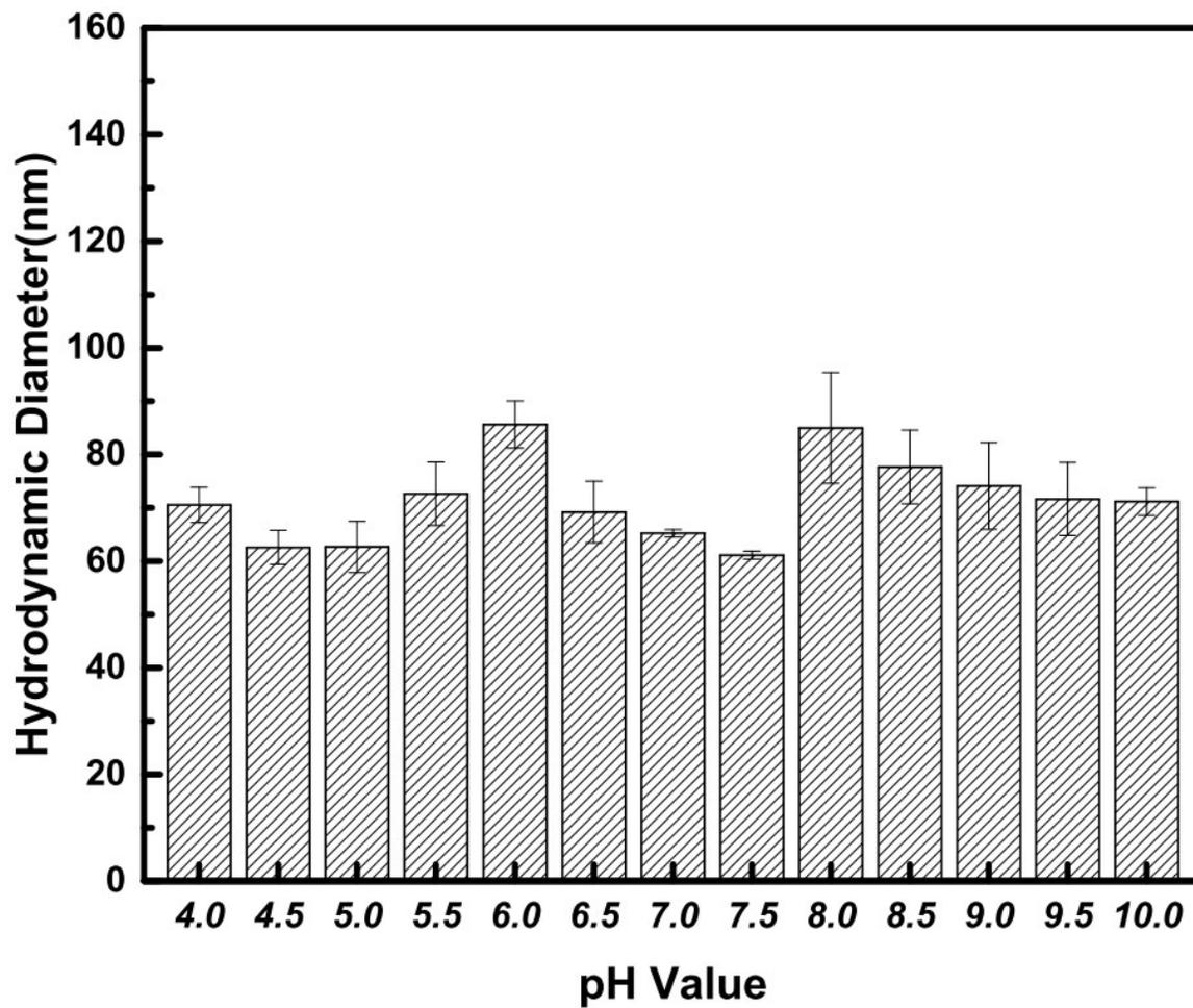
**Figure S5.** Effect of solution pH on the hydrodynamic diameter of LysNP-AuNCs. LysNP-AuNCs were prepared in 10 mM phosphate buffer at pH 4.0–10.0.
