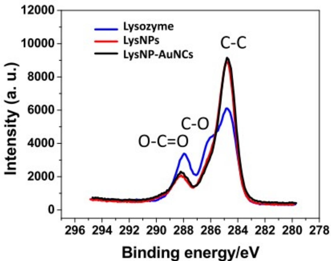
**Figure S10.** High-resolution C1S XPS spectra of LysNP-AuNCs (black curve), LysNPs (red curve), and lysozyme (blue line). LysNP-AuNCs, LysNPs, and lysozyme were all prepared in 10 mM phosphate buffer at pH 10.
