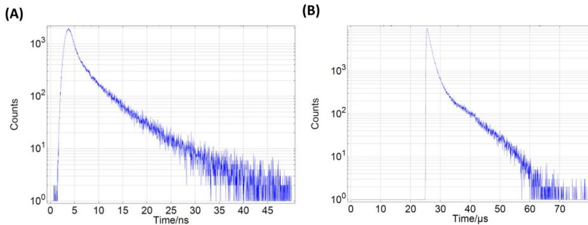
**Figure S2.** Fluorescence lifetime decay of LysNP-AuNCs at emission wavelength of (A) 495 and (B) 676 nm.
