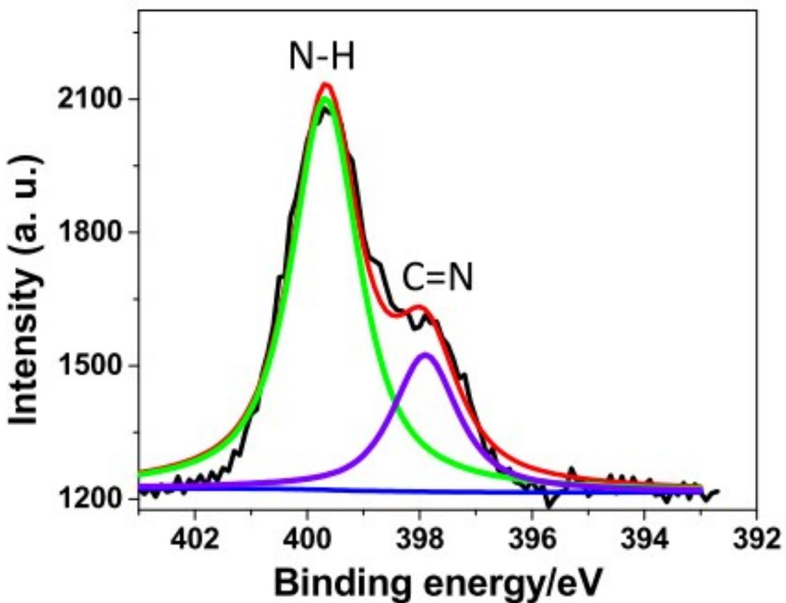
**Figure S9.** High-resolution N1s XPS spectra of LysNP-AuNCs. The original spectrum is in black, the fitted spectrum is in red, the deconvoluted spectra are in green (C=N) and violet (N-H bond).
