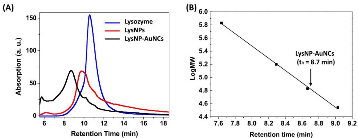
**Figure S7.** (A) SEC chromatograms of LysNP-AuNCs (black line), LysNPs (red line), and lysozyme (blue line). (B) A plot of the logarithm of protein molecular weight versus the retention time.
