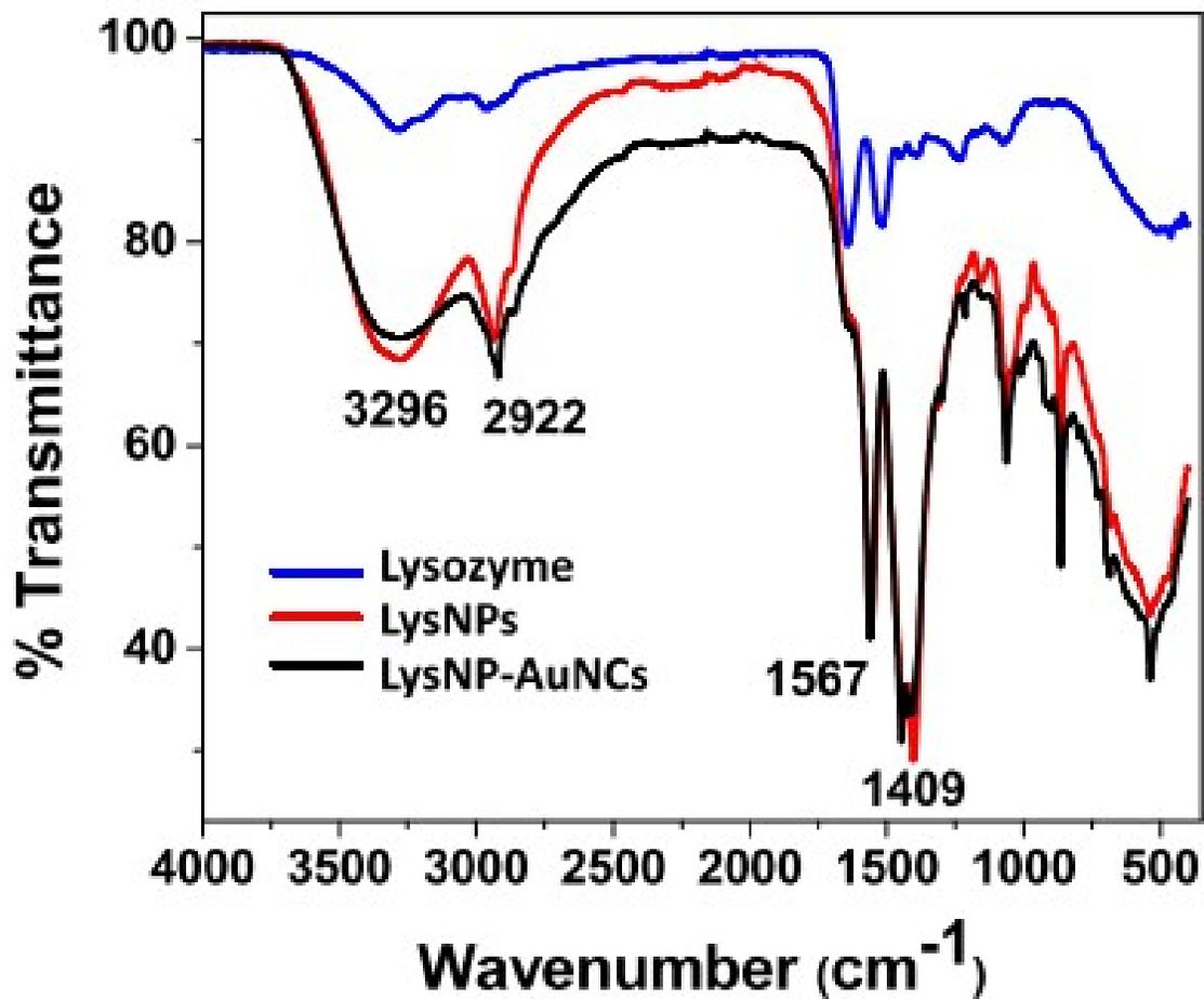
**Figure S11.** FT-IR spectra of LysNP-AuNCs (black curve), LysNPs (red curve), and lysozyme (blue line). LysNP-AuNCs, LysNPs, and lysozyme were all prepared in 10 mM phosphate buffer at pH 10.
