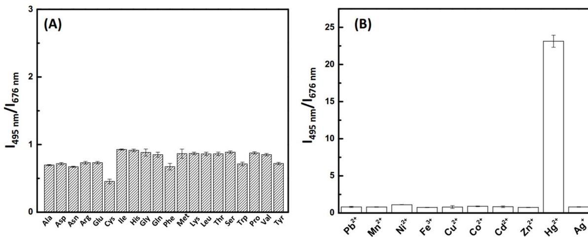
**Figure S14.** Effects of (A) amino acids and (B) metal ions on the  $I_{495 \text{ nm}}/I_{676 \text{ nm}}$  value of LysNP-AuNCs. The concentration of amino acids and metal ions are both 100  $\mu\text{M}$ . LysNP-AuNCs were prepared in 10 mM phosphate buffer at pH 7.5.
