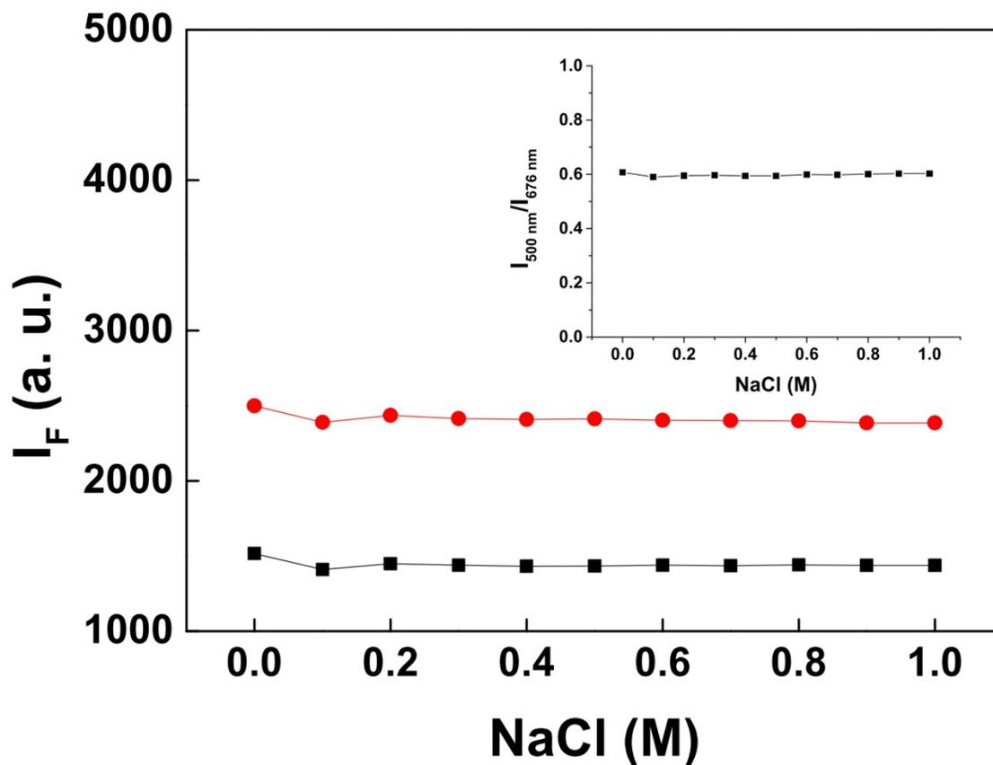
**Figure S3.** Effect of the NaCl concentration on the fluorescence intensity of LysNP-AuNCs at 495 nm (solid black square) and 676 nm (solid red circle). Inset: the  $I_{500 \text{ nm}}/I_{676 \text{ nm}}$  value of lysNP-AuNCs as a function of the NaCl concentration. LysNP-AuNCs were prepared in 10 mM phosphate buffer at pH 7.5.
