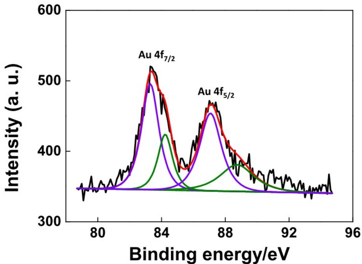
**Figure S6.** High-resolution Au4f XPS spectrum of Lys NPs-AuNCs. The original spectrum is in black, the fitted spectrum is in red, the A(0) 4f<sub>7/2</sub> and 4f<sub>5/2</sub> spectra are in purple, and the A(I) 4f<sub>7/2</sub> and 4f<sub>5/2</sub> spectra are in green
