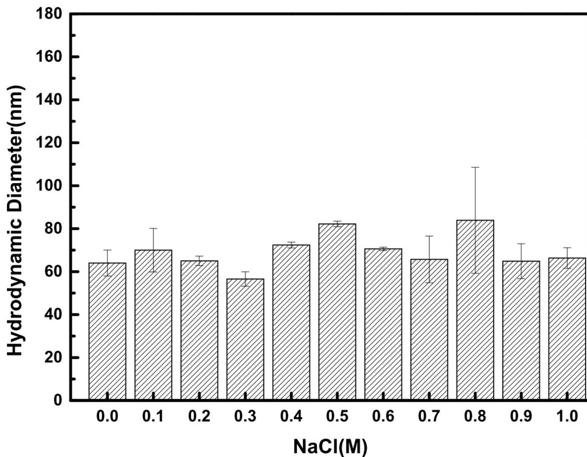
**Figure S4.** Effect of the NaCl concentration on the hydrodynamic diameter of LysNP-AuNCs. LysNP-AuNCs were prepared in 10 mM phosphate buffer at pH 7.5.
