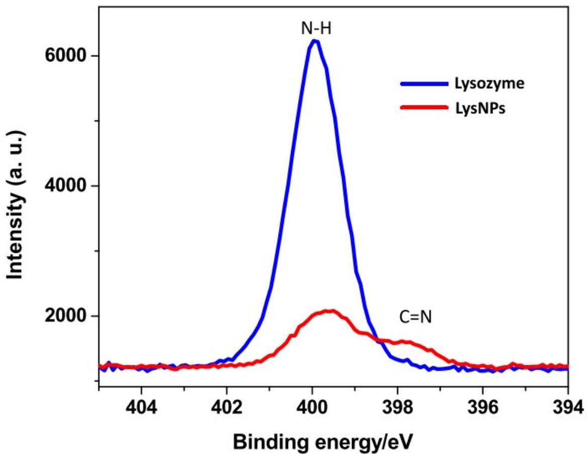
Figure S8. High-resolution N1s XPS spectrum of Lysozyme and LysNPs.
