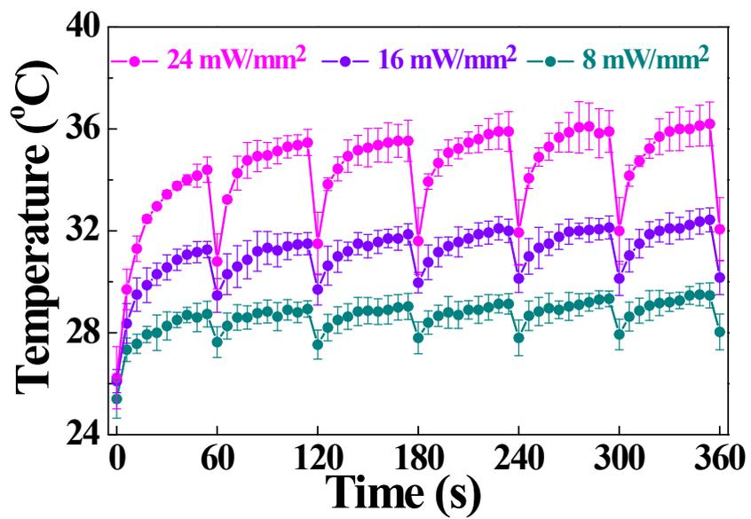
Figure S6. Changes of temperature for the hydrogel actuator under switchable irradiation of NIR light.
