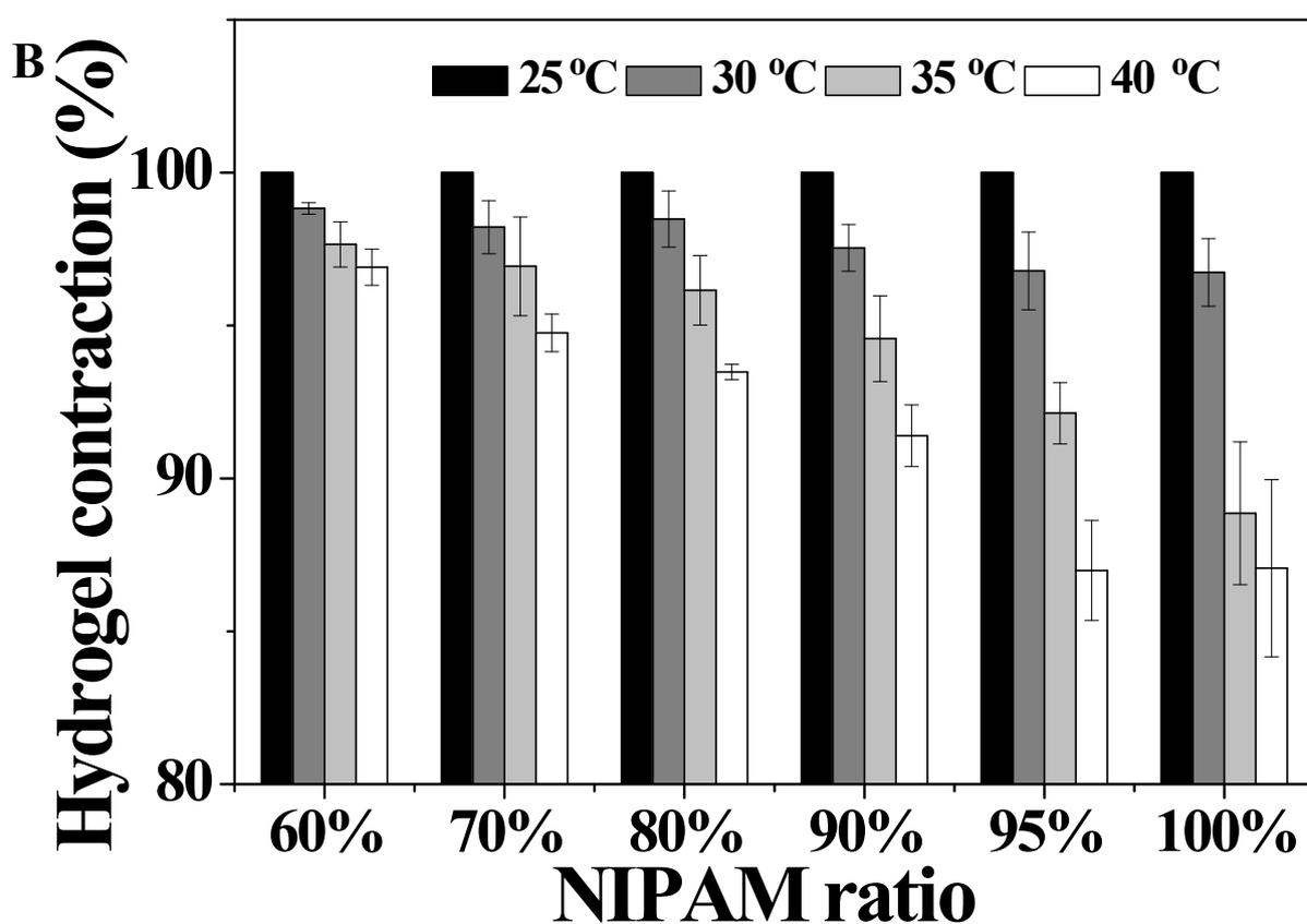
**Figure S2. Characterizations of thermal responses for the hydrogel actuators. (A) Optical images of the hydrogel actuators. (B) Quantitative analysis the hydrogel contraction at different temperature.**
