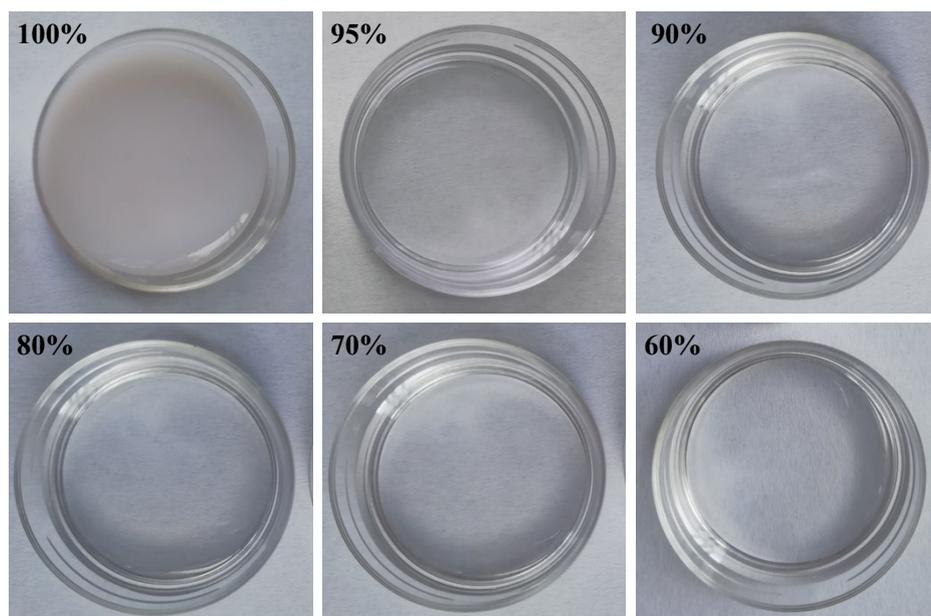
**Figure S1. Analyzing the optical transparency of hydrogel actuators prepared with different NIPAM ration in the monomer from 100% to 60%.**
