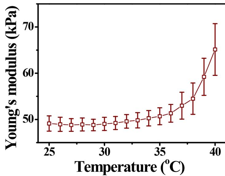
Figure S7. The Young's modulus of the prepared hydrogel actuator as a function of temperature.
