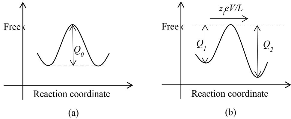
**Figure S4.** Schematic of the field effect on the activation energy for the rate process controlling the anodic growth of Ti nanotubes.
