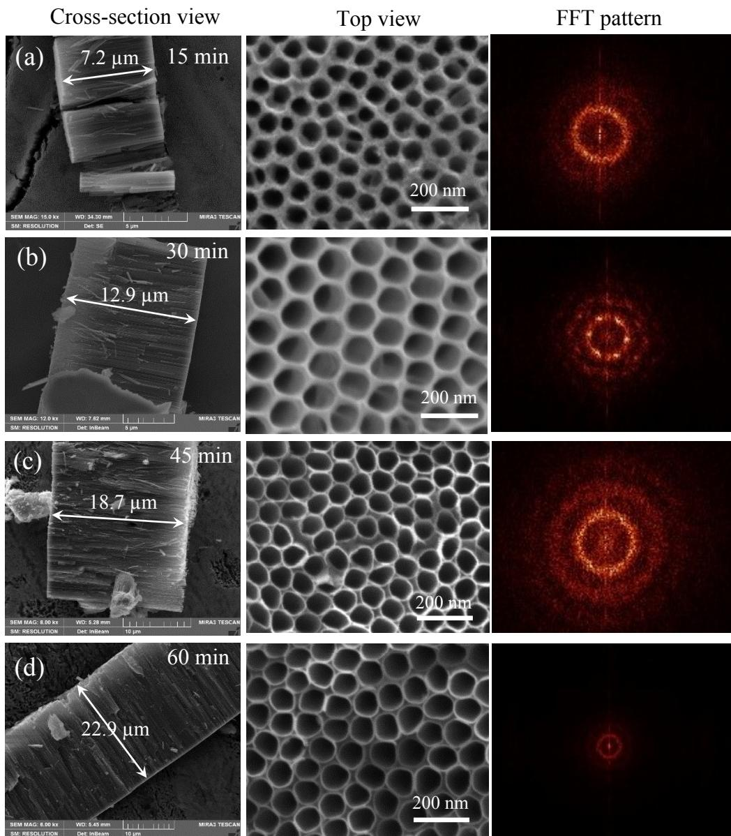
**Figure S2.** SEM images and the corresponding FFT patterns of  $\text{TiO}_2$  nanotube arrays formed at different anodization times (voltage: 50 V, temperature: 50°C): (a) 15 min, (b) 30 min, (c) 45 min, and (d) 60 min.
