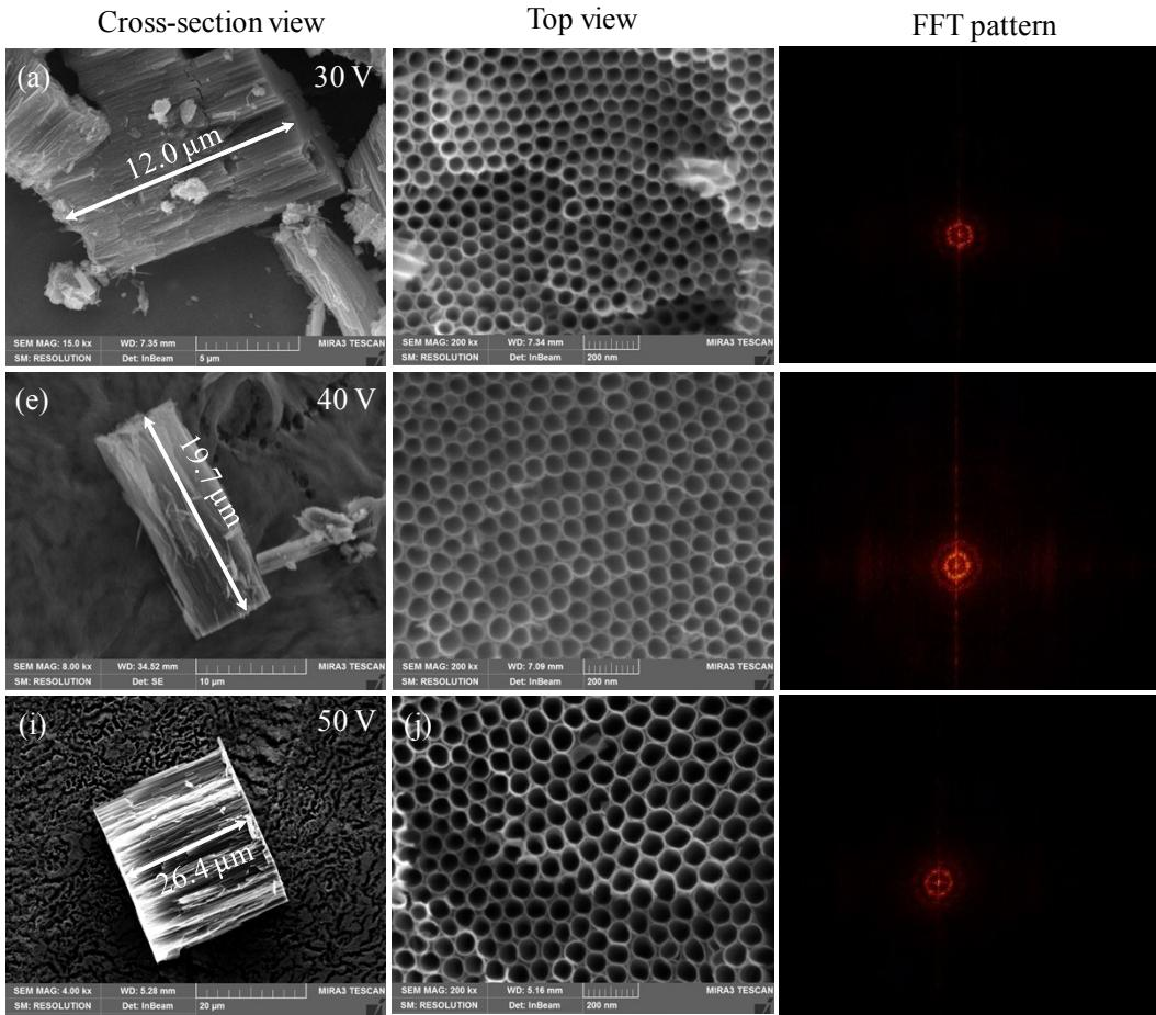
**Figure S3.** SEM images and the corresponding FFT patterns of  $\text{TiO}_2$  nanotube arrays formed at different anodization voltages (time: 60 min, temperature: 50°C): (a) 30 V, (b) 40 V, and (c) 50 V.
