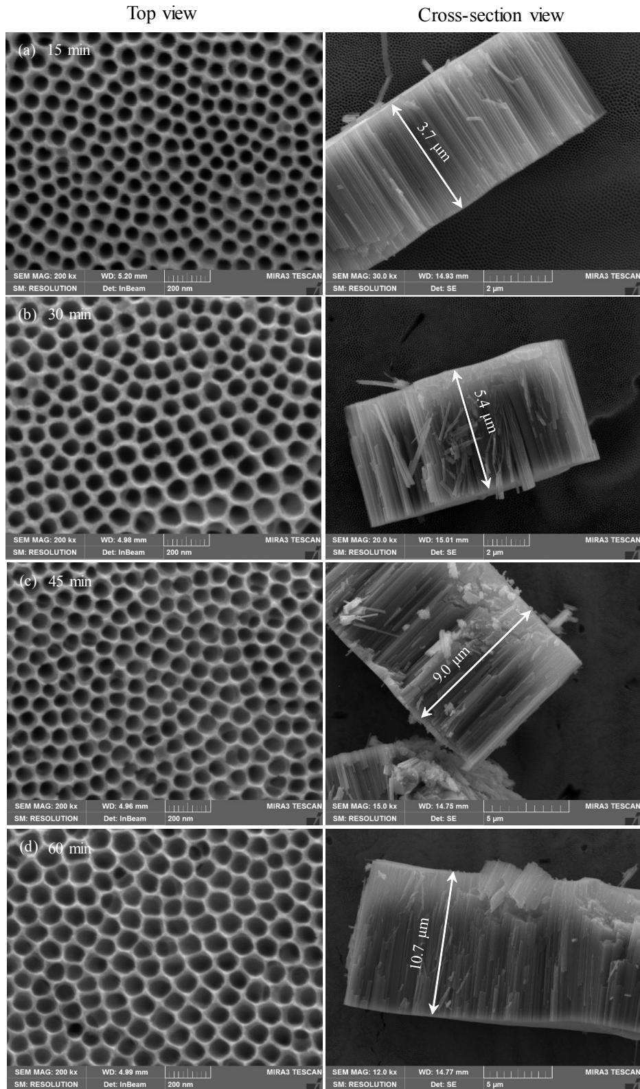
**Figure S1.** SEM images of the TNTs synthesized at a temperature of 40 °C and a voltage of 40 V with different anodization times: (a) 15 min, (b) 30 min, (c) 45 min, and (d) 60 min.
