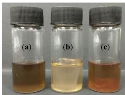
**Fig. S12** Gel fraction tests with the same amount of (a) LCE-1, (b) LCE-2, and (c) LCE-3 immersed in THF with fixed volume at room temperature for 12 h to investigate the cross-linking degree and the retrocycloaddition-based de-cross-linking efficiency in our LCE films.
