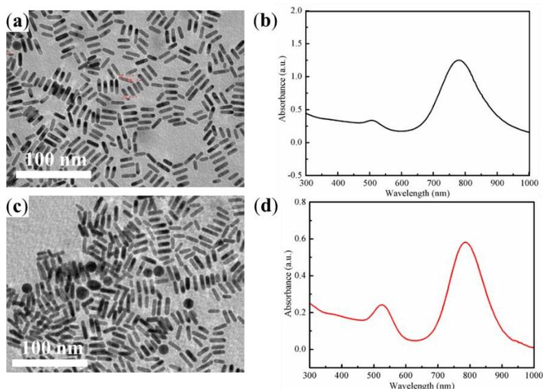
**Fig. S2** (a, c) TEM images and (b, d) UV-vis spectra for (a, b) the aqueous dispersed CTAB-GNRs, and (c, d) the organ soluble PMMS-GNRs.
