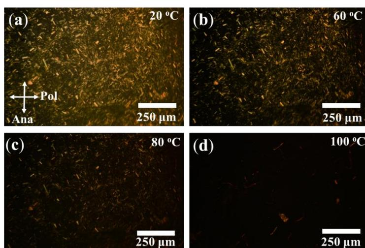
**Fig. S13** POM images of a 313 nm UV light-crosslinked GNR/LCE composite film without stretching at different temperature of (a) 20 °C, (b) 60 °C, (c) 80 °C, (d) 100 °C.
