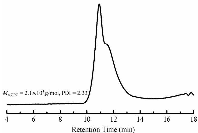
**Fig. S11** GPC chromatogram of the copolymer P(BP<sub>0.8</sub>-r-CM<sub>0.2</sub>). Polymerization conditions: [COC-BP]<sub>0</sub>: [COC-CM]<sub>0</sub>: [2nd generation Grubbs' catalyst]<sub>0</sub> = 350: 85: 1, n<sub>COC-BP</sub> = 0.99 mmol, V<sub>DCM</sub> = 2.0 mL, T = 55 °C, N<sub>2</sub> atmosphere.
