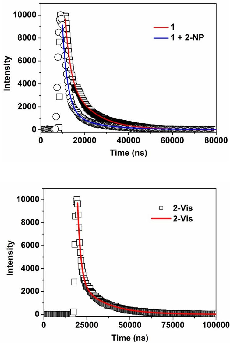
**Figure S6.** The lanthanide emission lifetimes of **1** (without the addition of 2-NP and with the addition of 700  $\mu$ M 2-NP) and **2** in  $\text{CH}_3\text{CN}$ .
