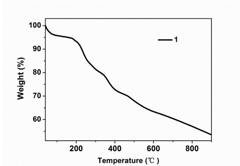
**Figure S2.** The thermogravimetric analysis of **1**.
