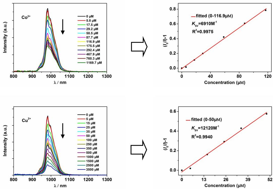
**Figure S8.** NIR luminescent sensing of **1** (15  $\mu\text{M}$ ) to metal ions in  $\text{CH}_3\text{CN}$  ( $\lambda_{\text{ex}} = 390 \text{ nm}$ ).
