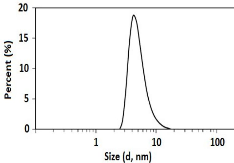
**Figure S4.** Dynamic light scattering (DLS) measurements of **1** in CH<sub>3</sub>CN.
