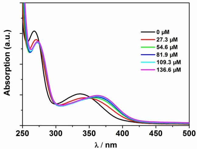
**Figure S10.** UV-Vis spectra of **1** with the addition of different concentrations of  $\text{Cd}^{2+}$  in  $\text{CH}_3\text{CN}$ .
