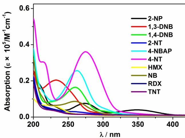
**Figure S12.** UV-Vis absorption spectra of explosives in  $\text{CH}_3\text{CN}$ .
