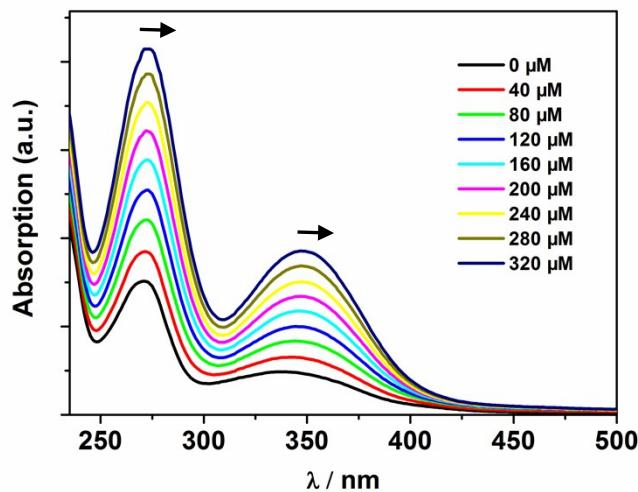
**Figure S11.** UV-Vis spectra of **1** with the additional of 2-NP in  $\text{CH}_3\text{CN}$ .
