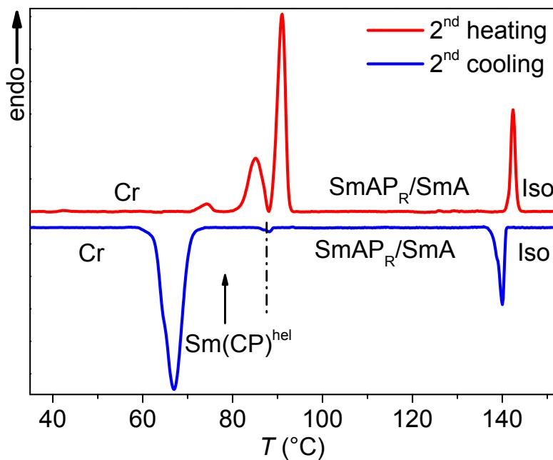
**Figure S30.** DSC heating and cooling traces of compound **C12/14** recorded at rates of 10 K min<sup>-1</sup>.
