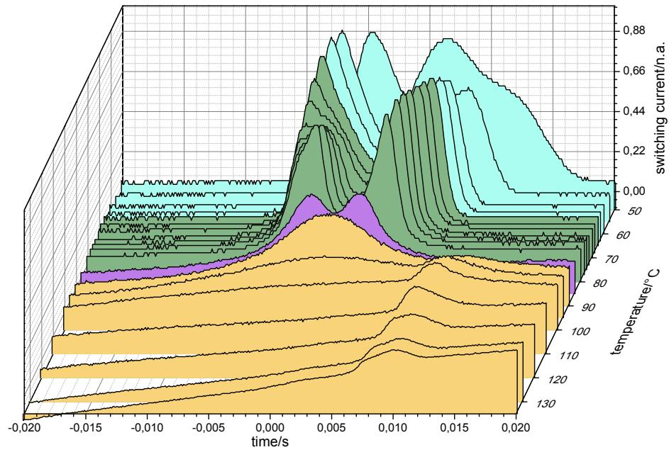
**Figure S16.** Polarization current response of **B16/6** depending on the temperature as measured in a ITO-coated cell (6  $\mu\text{m}$ ) under a triangular wave voltage of 160 V<sub>pp</sub> and a frequency of 10 Hz.
