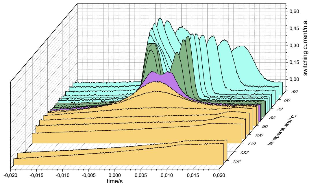
**Figure S24.** Polarization current response of **B22/6** depending on the temperature as measured in a ITO-coated cell (6  $\mu$ m) under a triangular wave voltage of 160 V<sub>pp</sub> and a frequency of 10 Hz.
