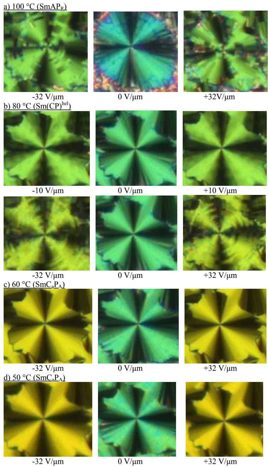
**Figure S20** (continued). Textures of the distinct mesophases of compound **B18/6** at the given temperatures in a planar cell as observed between crossed polarizers in the ground state without applied E-field (middle) and as observed for under an applied E-field at the indicated voltages (left/right).
