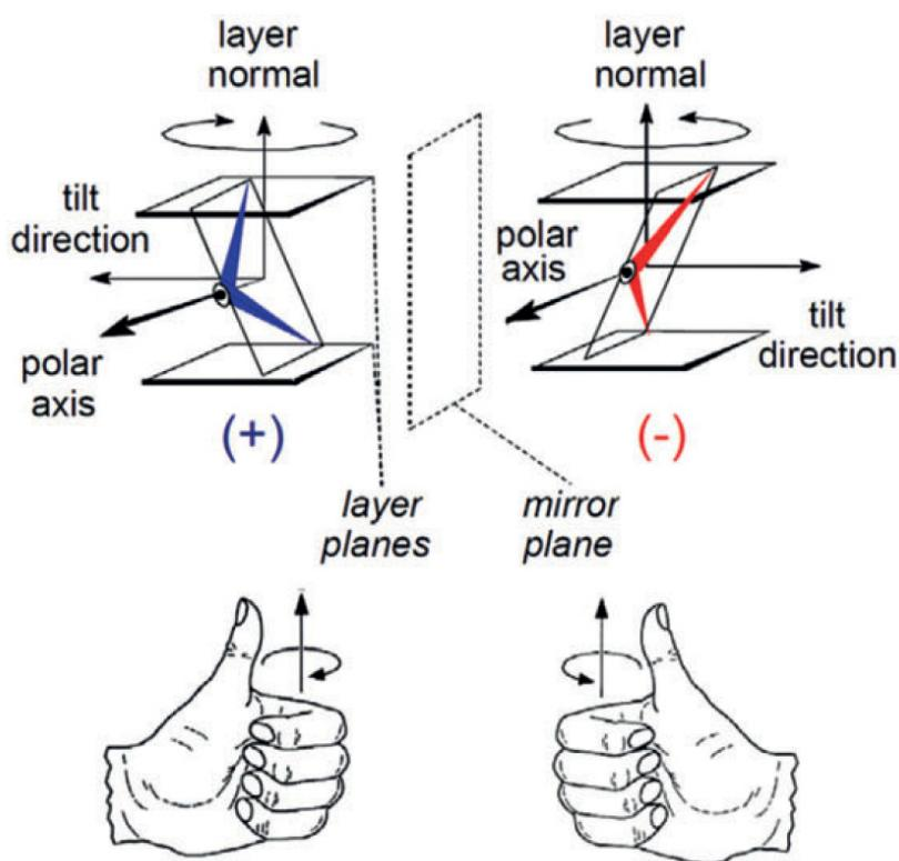
**Scheme S3.** Layer chirality and the structures of the polar SmC phases of bent-core mesogens. The orthogonal combination of tilt and polar order leads to reduced  $C_{2v}$  symmetry and superstructural chirality of the layers (adapted from ref.<sup>S14</sup>); blue/red color indicates the chirality sense; reproduced from Ref. S14 with permission from The Royal Society of Chemistry
