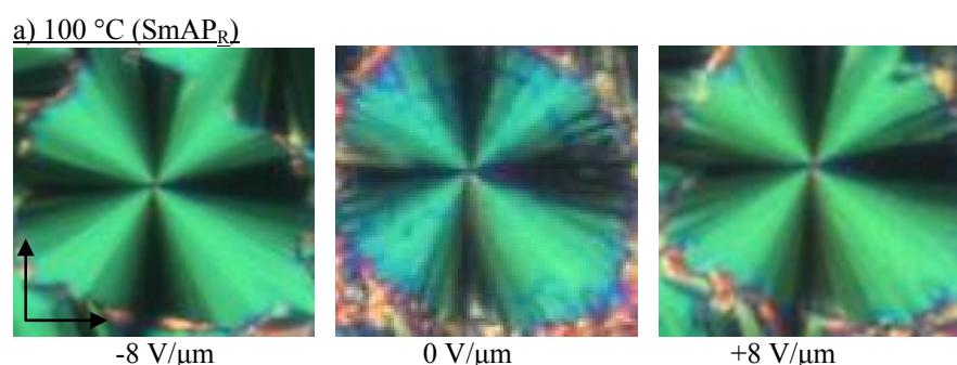
**Figure S20.** Textures of the  $\text{SmAP}_R$  of compound **B18/6** at the given temperatures in a planar cell as observed between crossed polarizers in the ground state without applied E-field (middle) and as observed for under an applied E-field of  $-/+ 8\text{ V}/\mu\text{m}$  (left/right).
