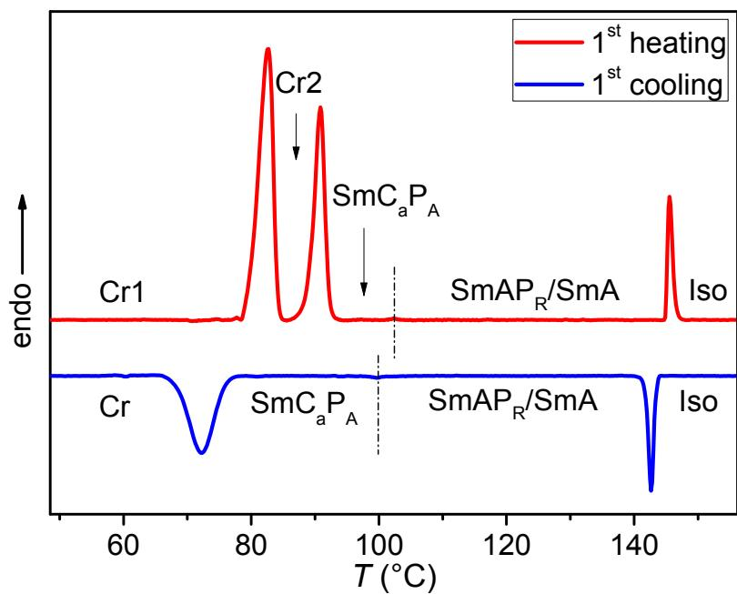
**Figure S53.** DSC heating and cooling traces of compound **D18/O6** recorded at rates of 10 K min<sup>-1</sup>.
