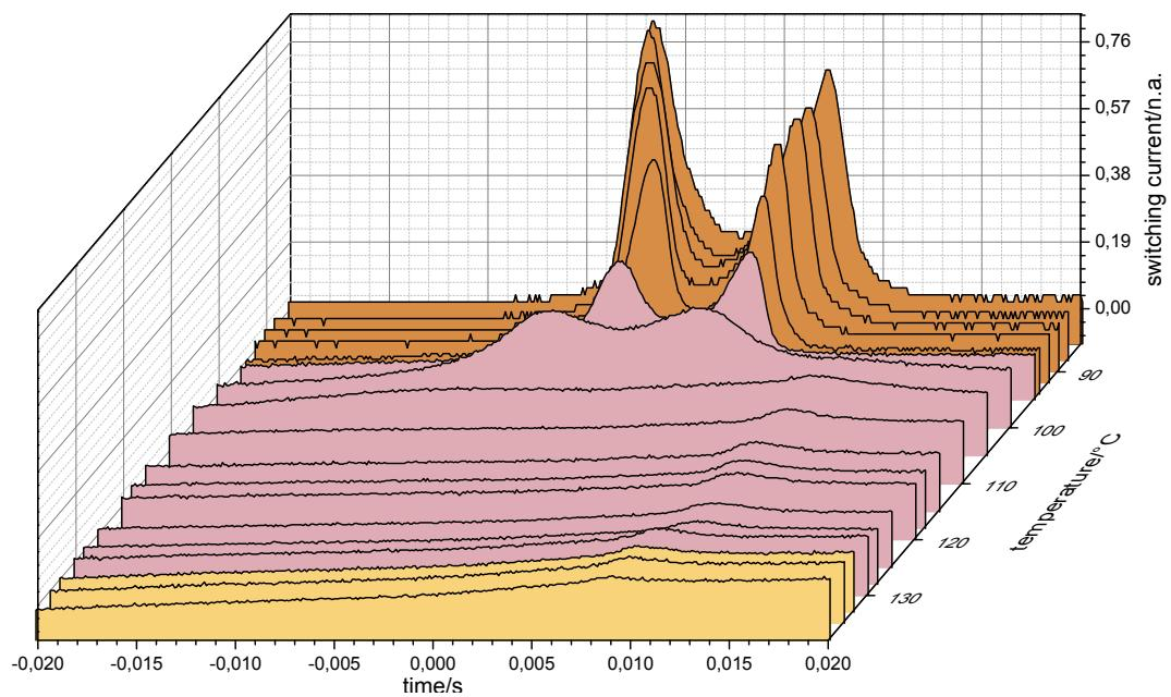
**Figure S49.** Polarization current response of **B18/18** depending on the temperature as measured in a ITO-coated cell (6  $\mu\text{m}$ ) under a triangular wave voltage of 160 V<sub>pp</sub> and a frequency of 10 Hz.
