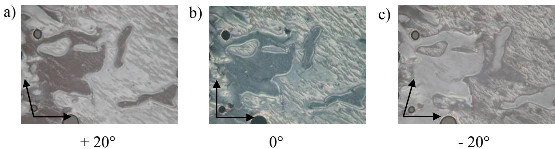
**Figure S35.** Chiral tilt-domains in the  $\text{SmCsP}_\text{R}^{[*]}$  phase of **C16/14** at  $T = 110$  °C as observed b) between crossed polarizers and a,c) between slightly uncrossed polarizers with the analyzer twisted by  $+/ - 20$  ° out of the perpendicular direction, respectively.
