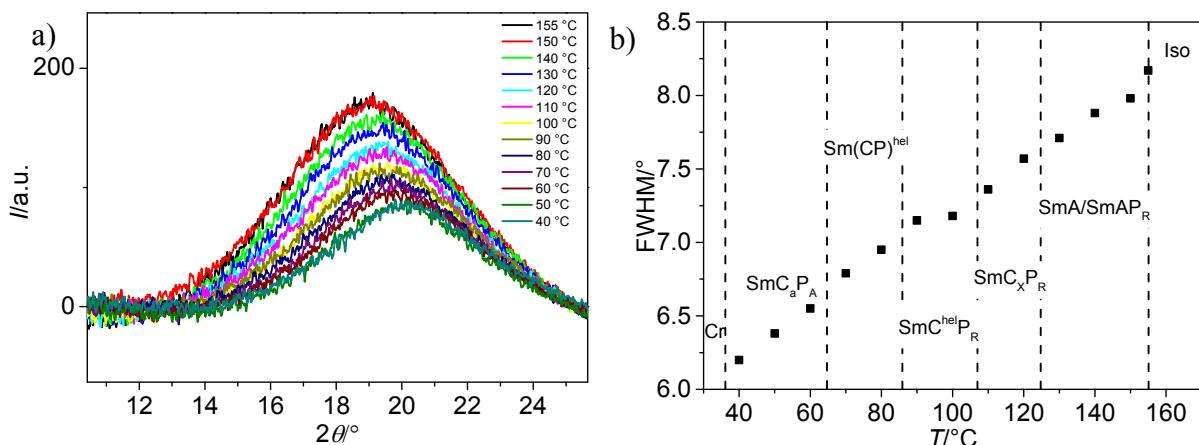
**Figure S56.** XRD data of compound **DO18/6** a)  $2\theta$  scans of the wide angle scatterings, b) plot of FWHM of the WAXS depending on the temperature.
