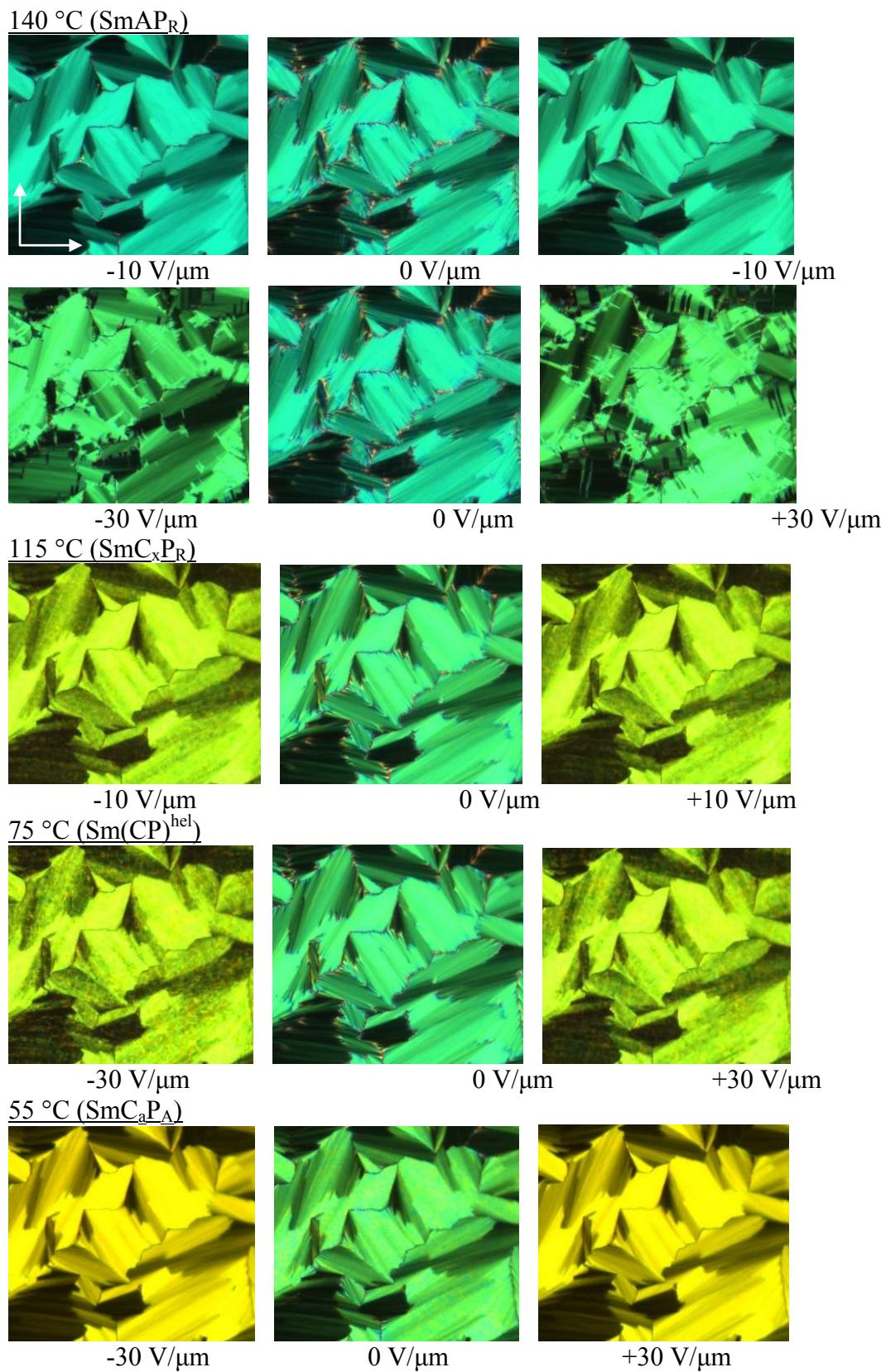
**Figure S57.** Textures of the distinct mesophases of compound **DO18/6** at the given temperatures in a planar cell as observed between crossed polarizers in the ground state without applied E-field (middle) and as observed for under an applied E-field at the indicated voltages (left/right).
