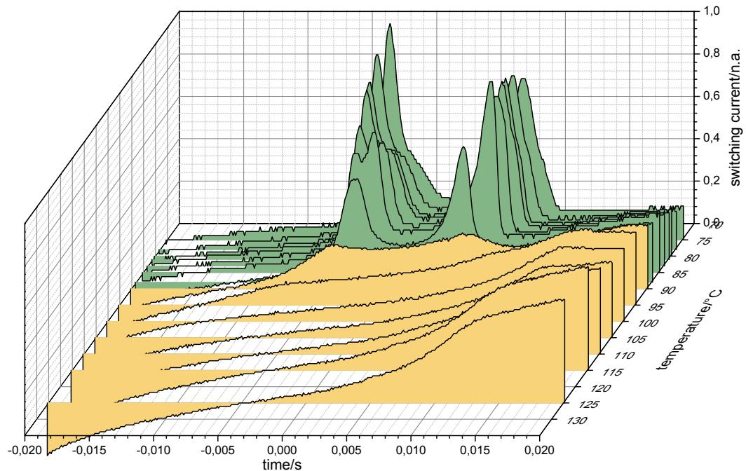
**Figure S31.** Polarization current response of **C12/14** depending on the temperature as measured in a ITO-coated cell (6  $\mu\text{m}$ ) under a triangular wave voltage of 160 V<sub>pp</sub> and a frequency of 10 Hz.
