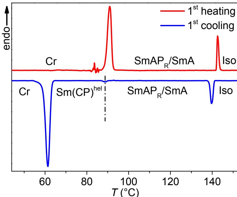
**Figure S26.** DSC heating and cooling traces of compound **C12/12** recorded at rates of 10 K min<sup>-1</sup>.
