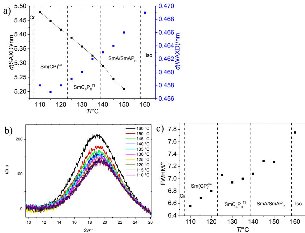
**Figure S63.** XRD data of compound **DO22/O6** a) plot of  $d$ -values of layer spacings and maxima of the wide angle scatterings depending on the temperature, b)  $2\theta$  scans of the WAXS, d) plot of FWHM depending on the temperature.
