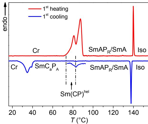
**Figure S21.** DSC heating and cooling traces of compound **B20/6** recorded at rates of 10 K min<sup>-1</sup>.
