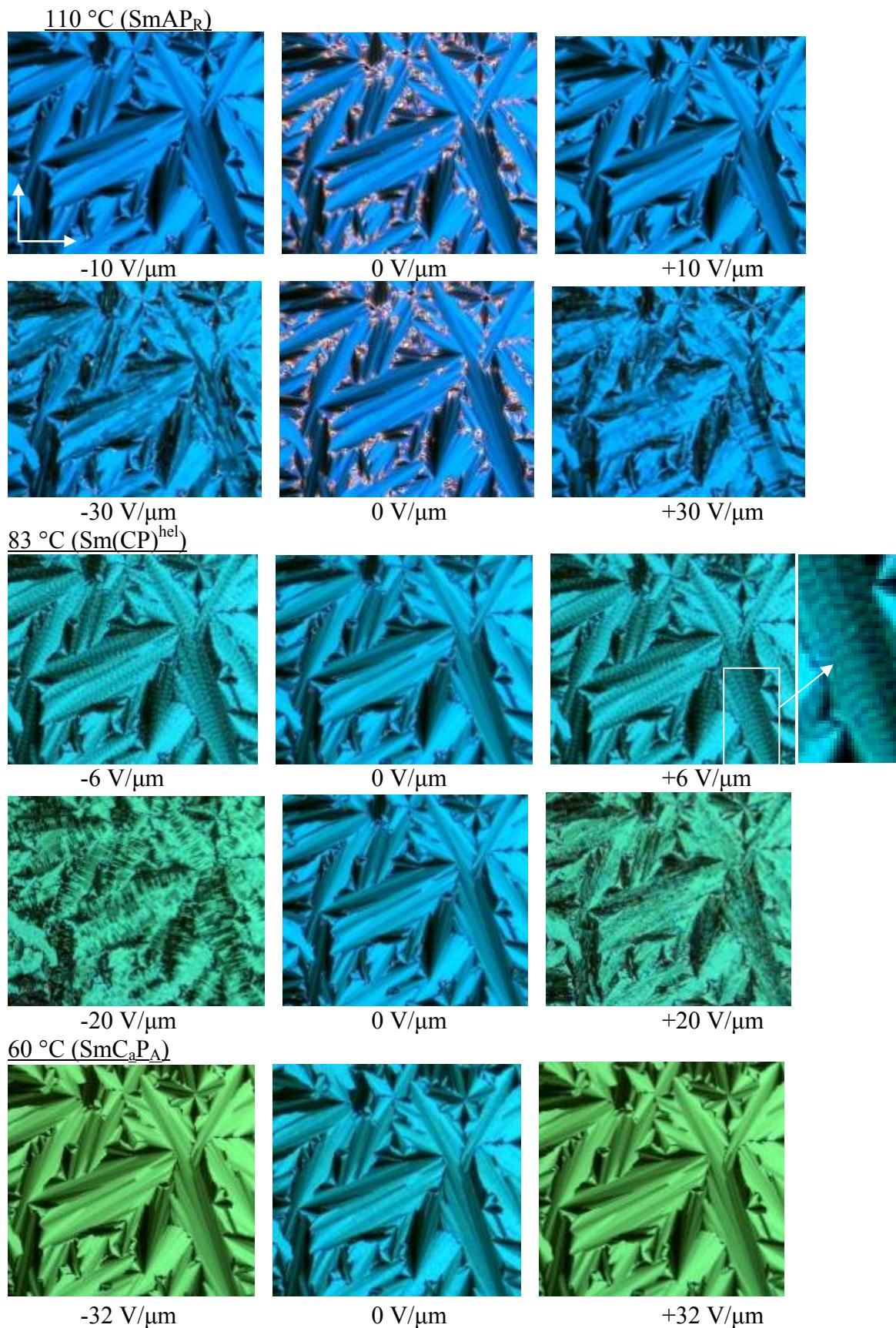
**Figure S25.** Textures of the distinct mesophases of compound **B22/6** at the given temperatures in a planar cell as observed between crossed polarizers in the ground state without applied E-field (middle) and as observed for under an applied E-field at the indicated voltages (left/right); the tiger stripe texture can be observed at  $\pm 6\text{ V}/\mu\text{m}$ .
