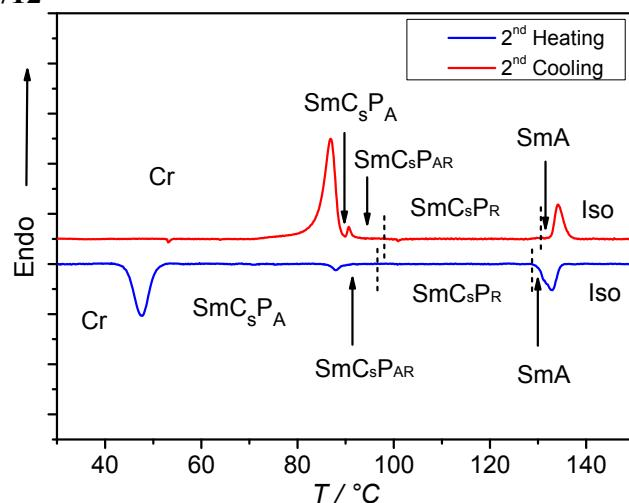
**Figure S78.** DSC heating and cooling traces of compound **F12/12** recorded at rates of 10 K  $\text{min}^{-1}$ .
