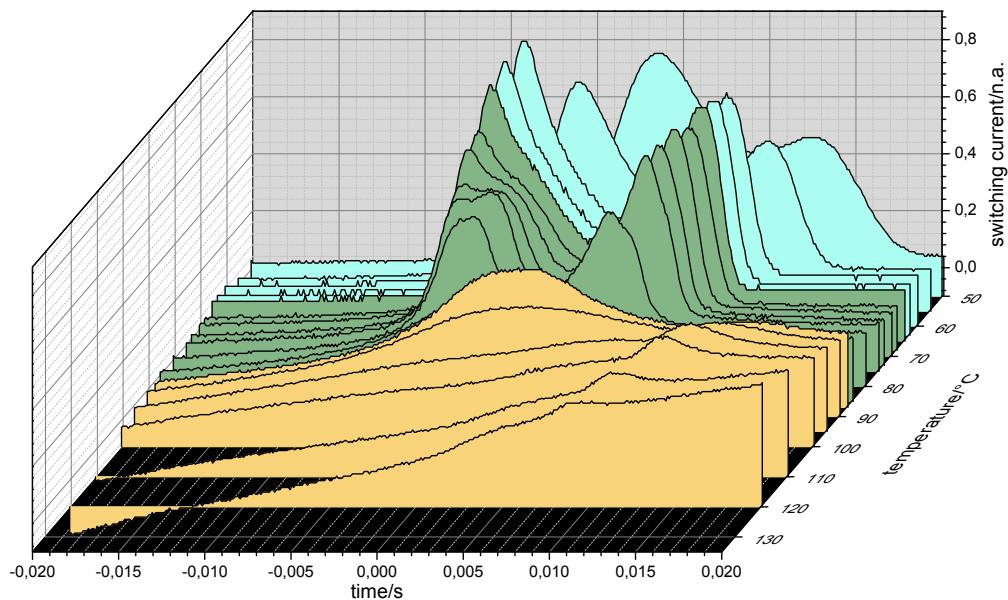
**Figure S13.** Polarization current response of **B14/6** depending on the temperature as measured in a ITO-coated cell (6  $\mu$ m) under a triangular wave voltage of 160 V<sub>pp</sub> and a frequency of 10 Hz.
