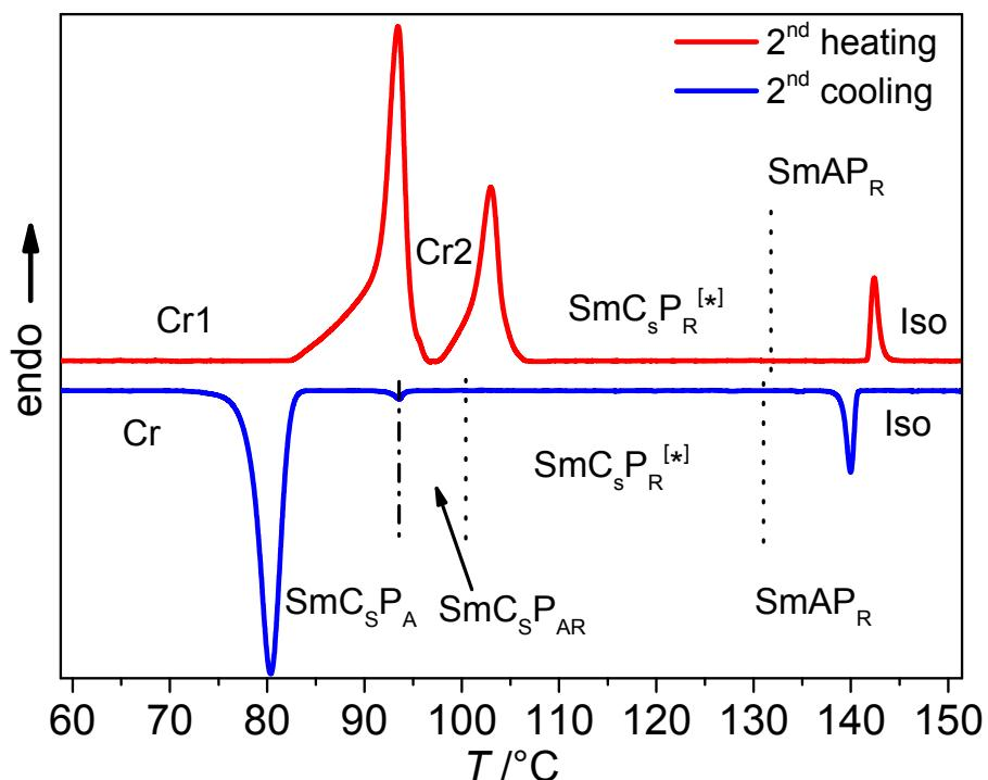
**Figure S47.** DSC heating and cooling traces of **C18/18** recorded at rates of  $10 \text{ K min}^{-1}$ ;
