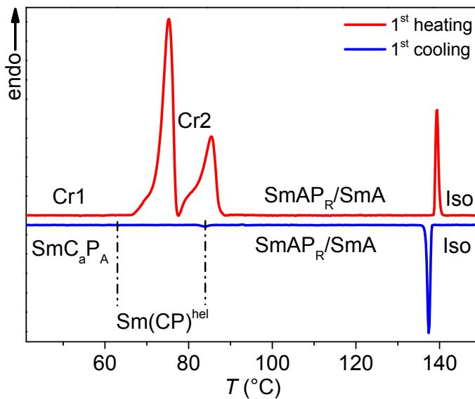
**Figure S14.** DSC heating and cooling traces of compound **B16/6** recorded at rates of 10 K min<sup>-1</sup>
