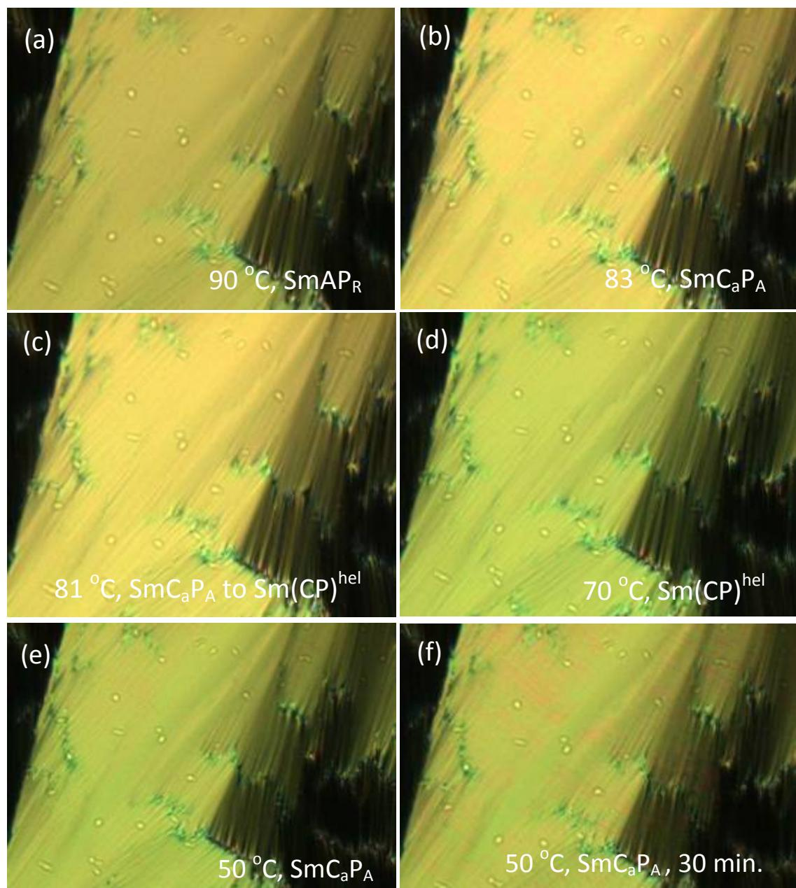
**Figure S8.** Development of the planar textures of compound **B12/6** with decreasing temperature; note the speckled texture in b), e) and f).
