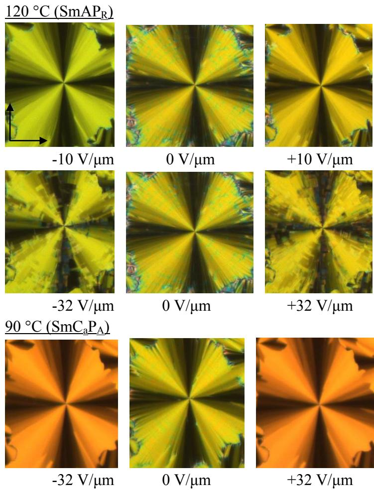
**Figure S55.** Textures of the distinct mesophases of compound **D18/O6** at the given temperatures in a planar cell as observed between crossed polarizers in the ground state without applied E-field (middle) and as observed for under an applied E-field at the indicated voltages (left/right).
