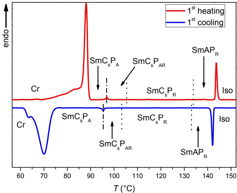
**Figure S40.** DSC heating and cooling traces of compound **C18/14** recorded at rates of 10 K min<sup>-1</sup>.
