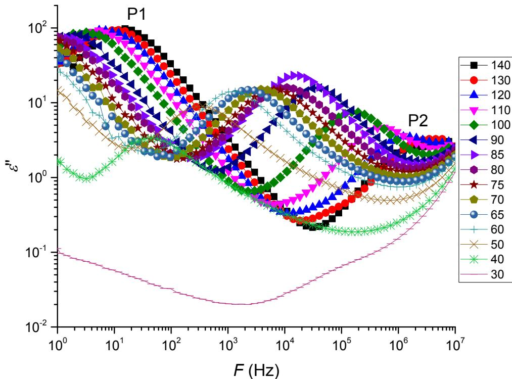
**Figure S11.** Frequency dependance of the  $\epsilon''$  for selected temperatures as observed in a 10  $\mu\text{m}$  planar cell.
