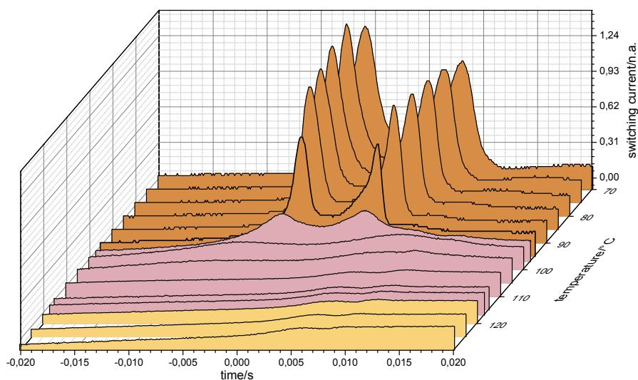
**Figure S34.** Polarization current response of **B14/14** depending on the temperature as measured in a ITO-coated cell (6  $\mu\text{m}$ ) under a triangular wave voltage of 160 V<sub>pp</sub> and a frequency of 10 Hz.
