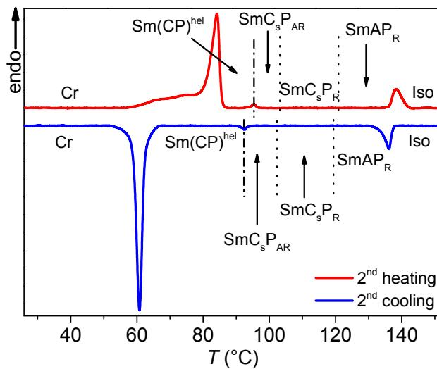
**Figure S32.** DSC heating and cooling traces of compound **C14/14** recorded at rates of 10 K min<sup>-1</sup>.
