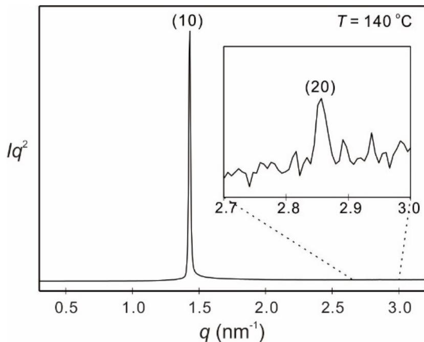
**Figure S85.** SAXS pattern of **EO12/O12** at 140 °C showing the weak (20) layer reflection and indicating the absence of a 2d-lattice (investigated with synchrotron source).
