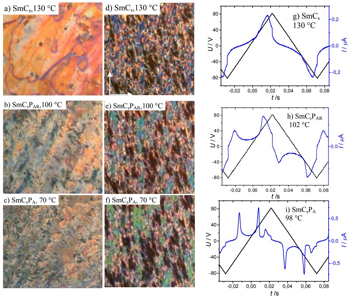
**Figure S82.** Homeotropic (left) and planar textures (middle) as observed between crossed polarizers and corresponding polarization current curves (right) of compound **EO12/12** at the given temperatures in the indicated LC phases; 160 Vpp, in a 6  $\mu\text{m}$  PI-coated ITO cell.
