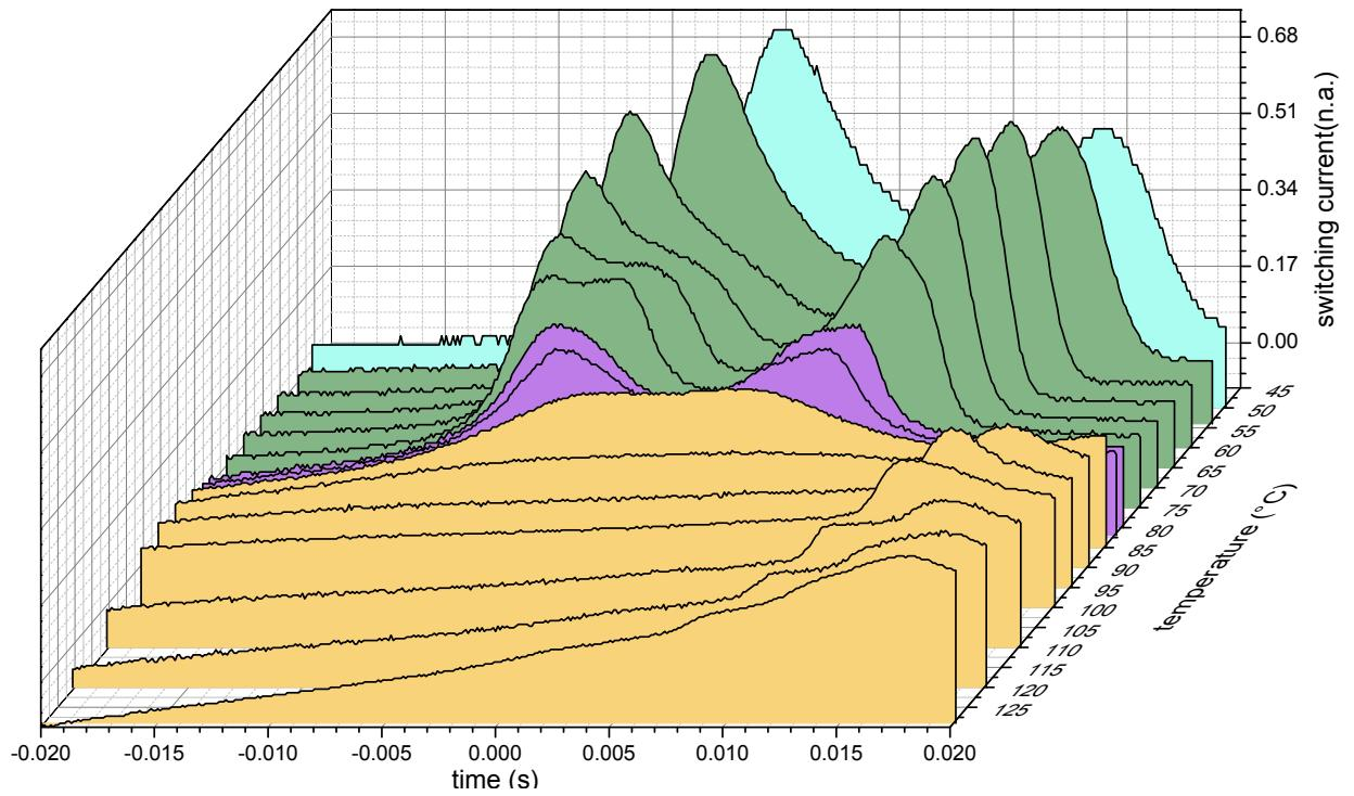
**Figure S10.** Polarization current response of **B12/6** depending on the temperature as measured in a ITO-coated cell (6  $\mu\text{m}$ ) under a triangular wave voltage of 160 V<sub>pp</sub> and a frequency of 10 Hz.
