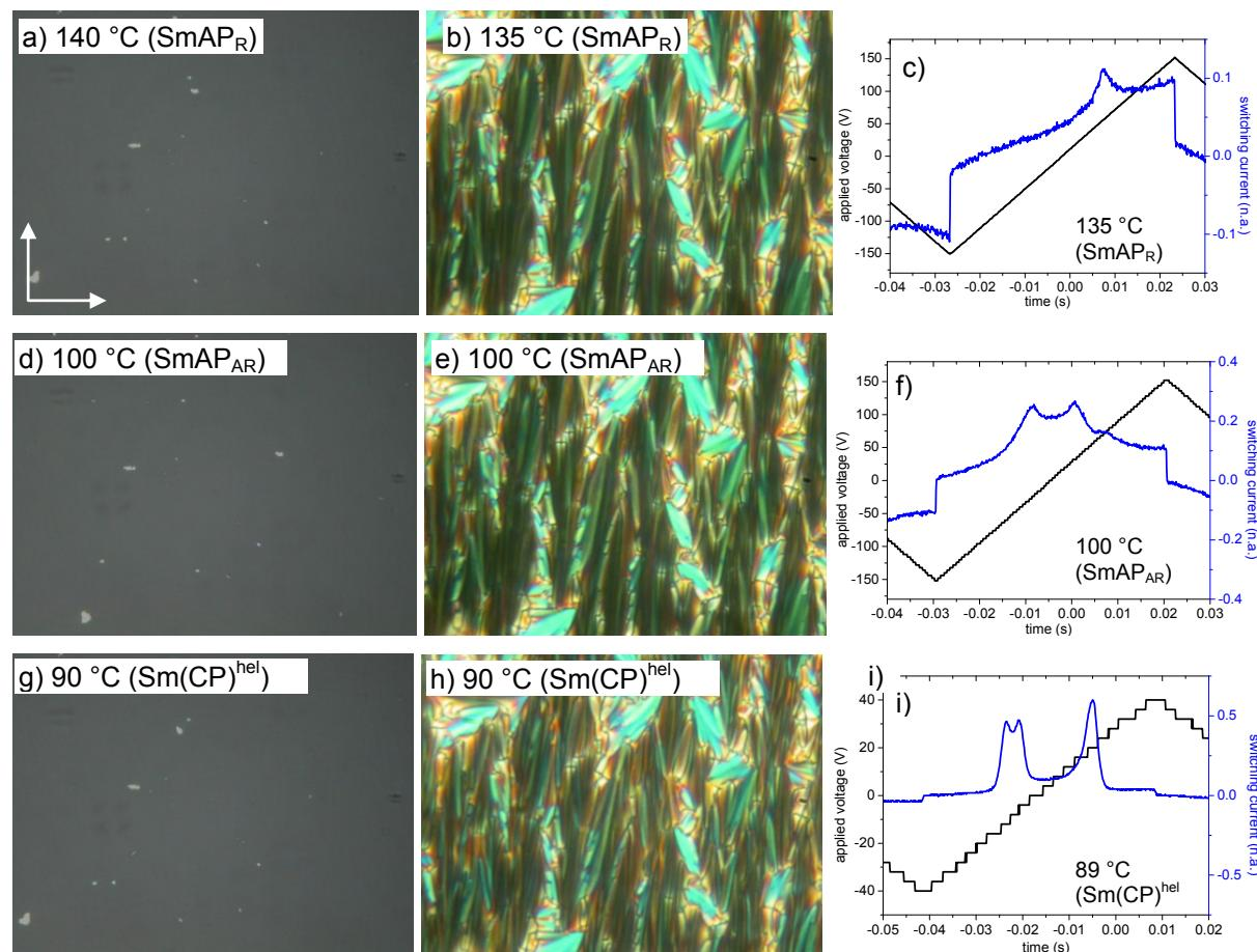
**Figure S69.** Homeotropic (left) and planar textures (middle) as observed between crossed polarizers and corresponding polarization current curves (right) of compound **DO12/12** at the given temperatures in the indicated LC phases. The polarization current response was measured in an ITO-coated cell (6  $\mu\text{m}$ , PI-coated) under a triangular wave voltage and a
