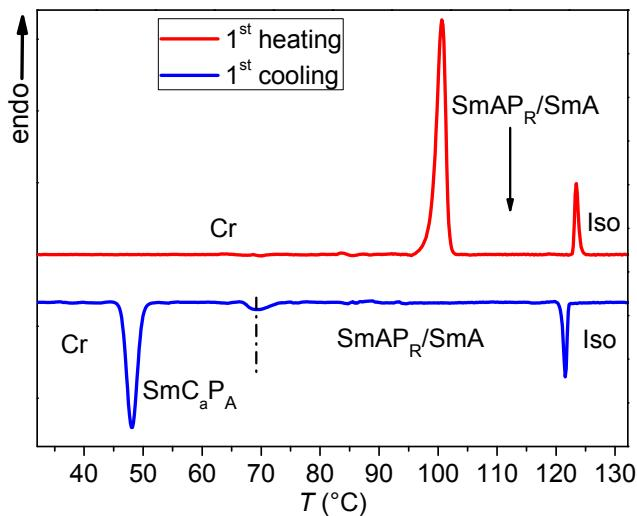
**Figure S2.** DSC heating and cooling traces of compound **B8/6** recorded at rates of 10 K min<sup>-1</sup>.
