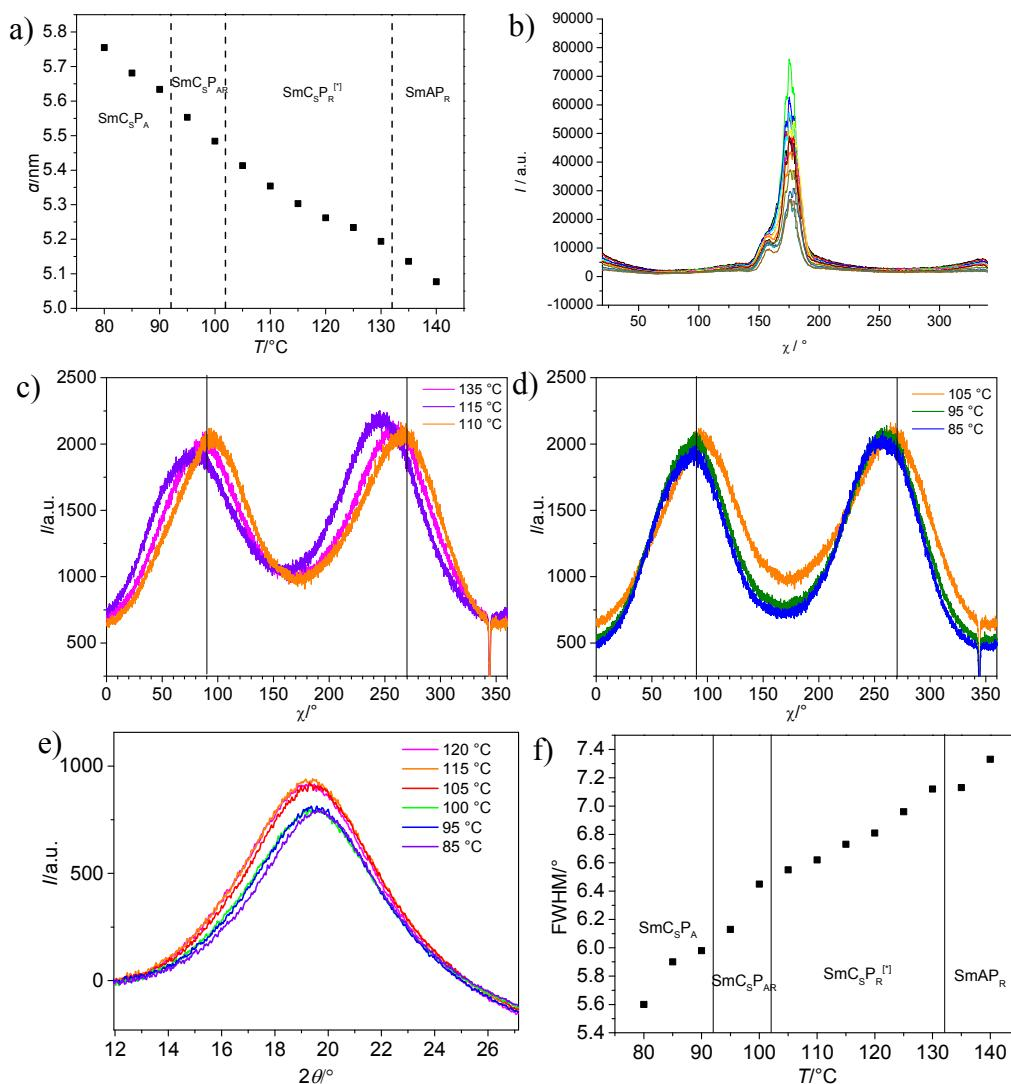
**Figure S 44.** XRD data of a magnetically aligned sample of compound **C22/12**. a) Plot of  $d$ -values of the layer spacing depending on temperature, b) intensity distribution of the SAXS ( $2\theta = 1-3^\circ$ ; main maximum at  $176^\circ$ , the small peak is due to misalignment) and c,d) the
