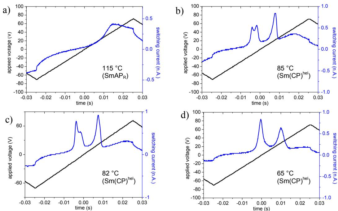
**Figure S27.** Polarization current response curves of **C12/12** at the indicated temperatures, measured in an ITO-coated cell (6  $\mu$ m) under a triangular wave voltage of 140 Vpp and a frequency of 10 Hz. a) SmAP<sub>R</sub>-phase at 115 °C, b-d) Sm(CP)<sup>hel</sup>-phase at b) 85 °C, c) 82 °C and d) 65 °C.
