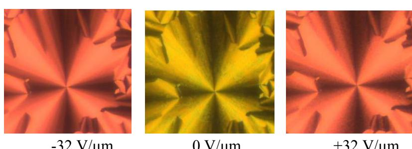
**Figure S7.** Textures of the distinct mesophases of compound **B10/6** at the given temperatures in a planar cell as observed between crossed polarizers in the ground state without applied E-field (middle) and as observed under an applied E-field at the indicated voltages (left/right).
