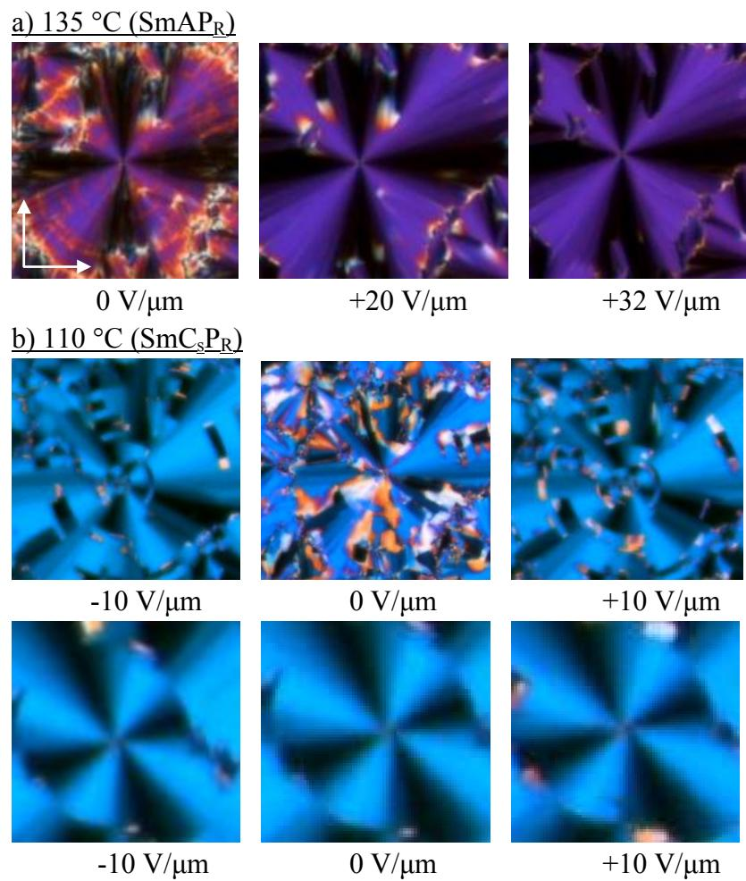
**Figure S42.** Textures of the distinct mesophases of compound **C18/14** at the given temperatures in a planar cell as observed between crossed polarizers in the ground state without applied E-field and as observed under an applied E-field at the indicated voltages; see Fig. 14 for the switching in the SmC<sub>S</sub>P<sub>A</sub> and field induced Sm(CP)<sup>hel</sup> phases.
