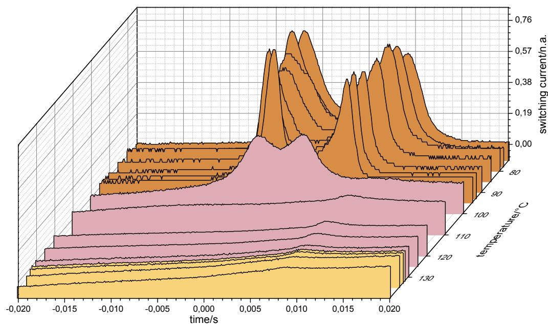
**Figure S41.** Polarization current response of **C18/14** depending on the temperature as measured in a ITO-coated cell (6  $\mu\text{m}$ ) under a triangular wave voltage of 160 V<sub>pp</sub> and a frequency of 10 Hz.
