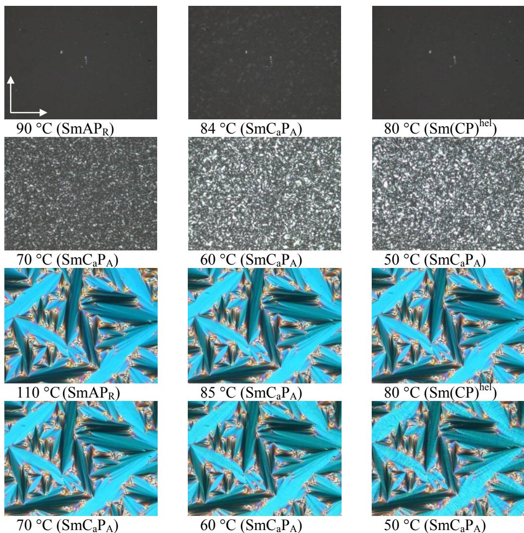
**Figure S18.** Textures of compound **B18/6** as observed between crossed polarizers depending on temperature; the two top rows show the homeotropic textures and the two bottom rows the planar fan-like textures at the given temperatures in the indicated LC phases;
