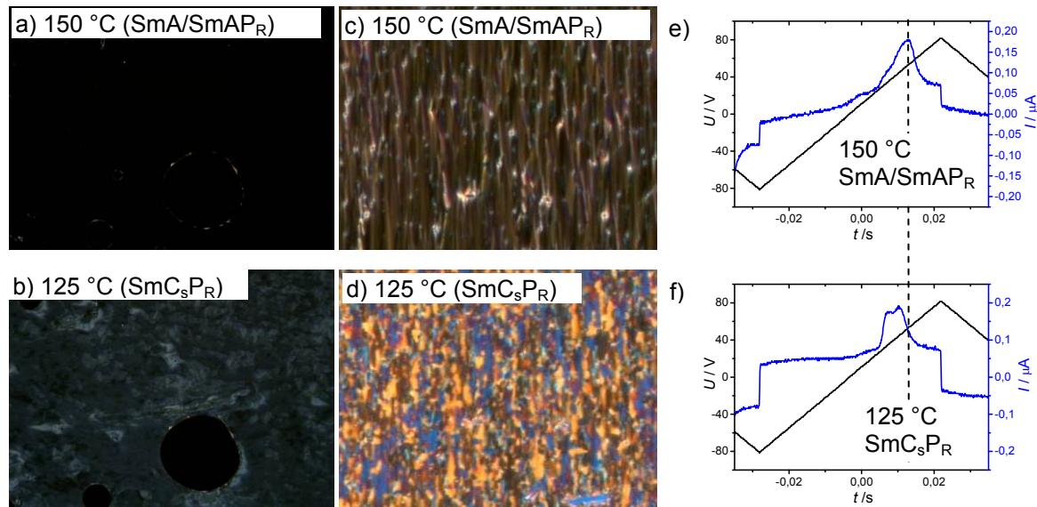
**Figure S77.** Homeotropic (left, a-b) and planar textures (middle, c-d) as observed between crossed polarizers and corresponding polarization current curves (right, e-f) of compound **DO14/O14** at the given temperatures in the indicated LC phases. The polarization current response was measured in an ITO-coated cell (6  $\mu\text{m}$ , PI-coated) under a triangular wave voltage and a frequency of 10 Hz.
