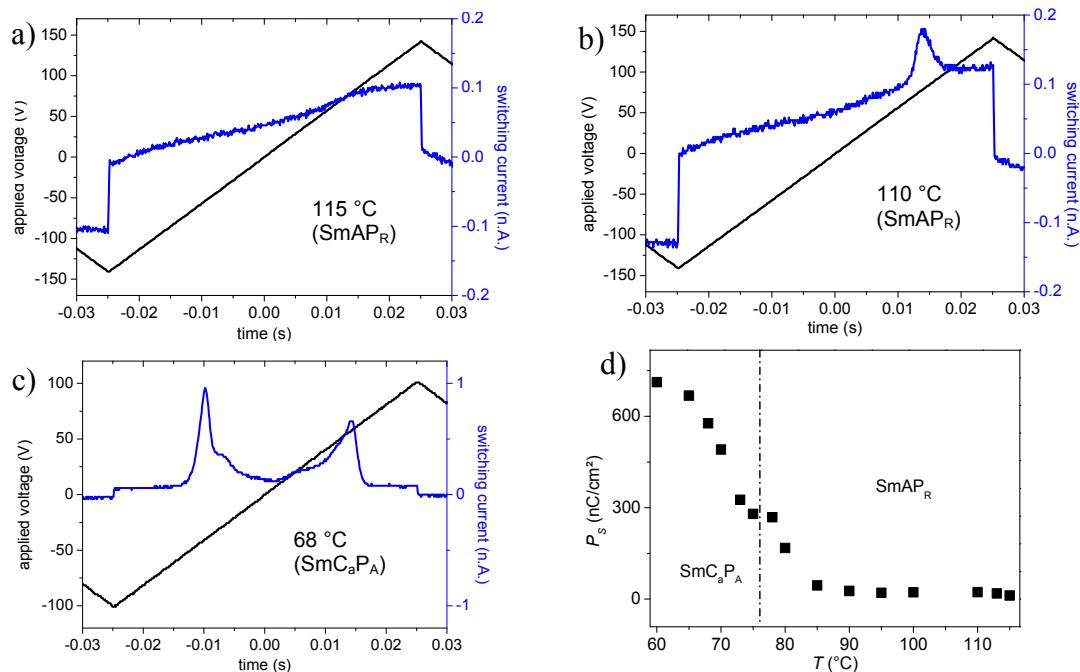
**Figure S3.** Polarization current response curves of **B8/6** at the indicated temperatures, measured in a ITO-coated cell (6  $\mu\text{m}$ ) under a triangular wave voltage of a,b)  $V_{\text{PP}} = 280$  V (Sm $A$ P<sub>R</sub>, a)  $T = 115$  °C, b)  $T = 110$  °C) and c)  $V_{\text{PP}} = 200$  V (SmC<sub>a</sub>P<sub>A</sub>,  $T = 68$  °C) and a frequency of 10 Hz; d) shows the development of the polarization values depending on  $T$ .
