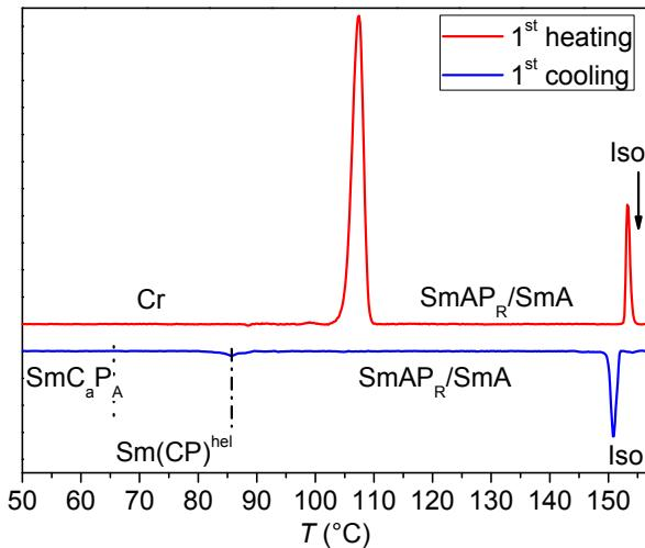
**Figure S65.** DSC heating and cooling traces of compound **DO12/6** recorded at rates of 10 K min<sup>-1</sup>.
