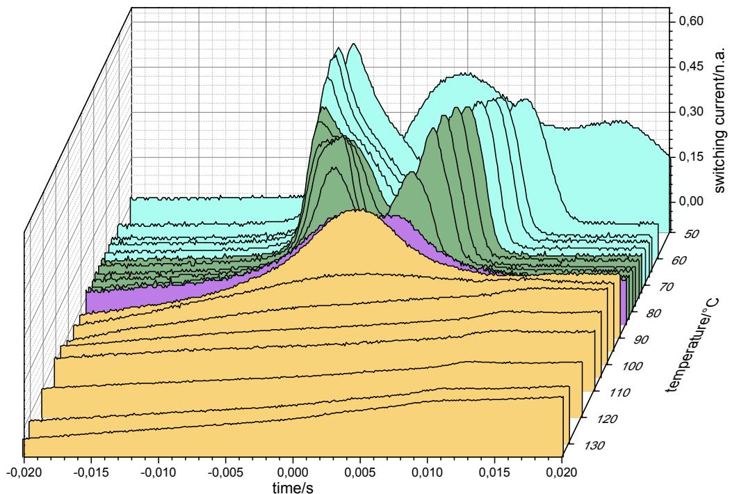
**Figure S22.** Polarization current response of **B20/6** depending on the temperature as measured in a ITO-coated cell (6  $\mu\text{m}$ ) under a triangular wave voltage of 160 V<sub>pp</sub> and a frequency of 10 Hz.
