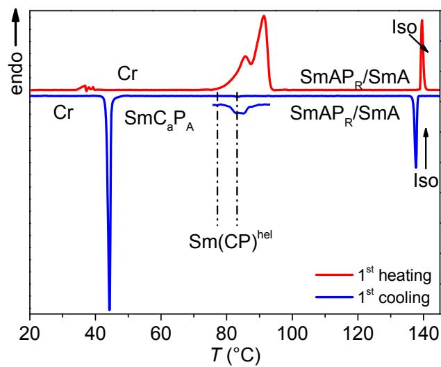
**Figure S23.** DSC heating and cooling traces of compound **B22/6** recorded at rates of 10 K min<sup>-1</sup>.
