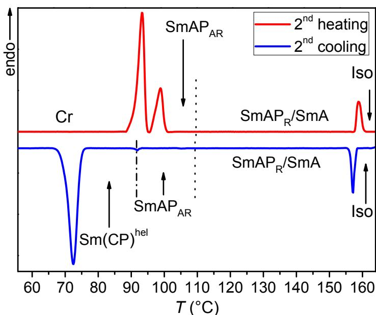
**Figure S68.** DSC heating and cooling traces of compound **DO12/12** recorded at rates of 10 K min<sup>-1</sup>.
