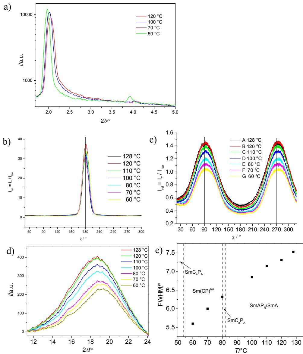
**Figure S9.** XRD data of compound **B12/6**. a) SAXS pattern; b) intensity distribution of the SAXS along  $\chi$  ( $2\theta = 1-5^\circ$ ) and c) of the WAXS along  $\chi$  ( $2\theta = 15-25^\circ$ ); there is no detectable tilt  $> 5^\circ$ ; d)  $2\theta$  scans of the WAXS and e) plot of FWHM of the WAXS depending on the temperature.
