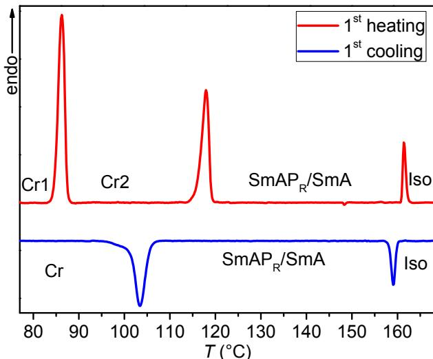
**Figure S60.** DSC heating and cooling traces of compound **DO18/O6** recorded at rates of 10 K min<sup>-1</sup>.
