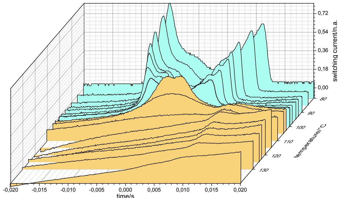
**Figure S54.** Polarization current response of **D18/O6** depending on the temperature as measured in a ITO-coated cell (6  $\mu\text{m}$ ) under a triangular wave voltage of 160 Vpp and a frequency of 10 Hz.
