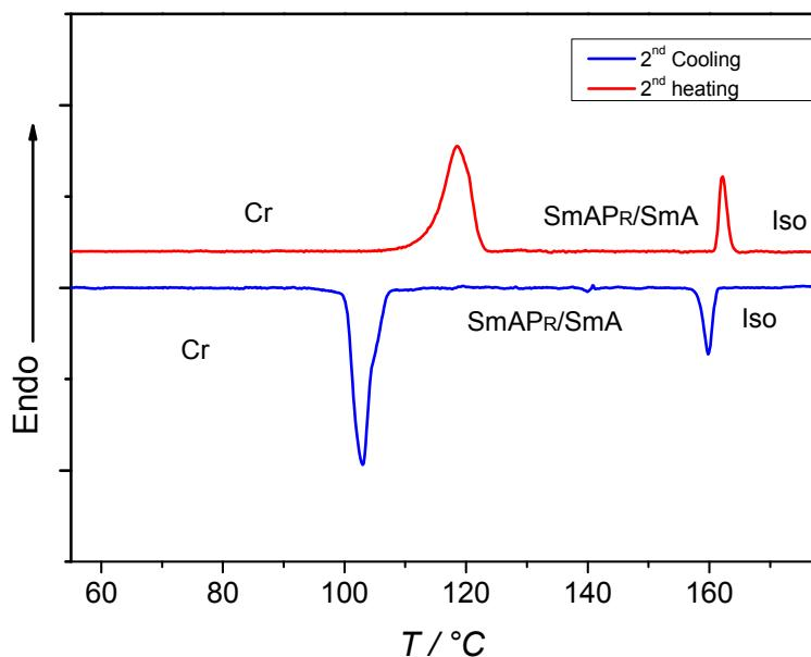
**Figure S72.** DSC heating and cooling traces of compound **DO12/O12** recorded at rates of 10  $\text{K min}^{-1}$ .
