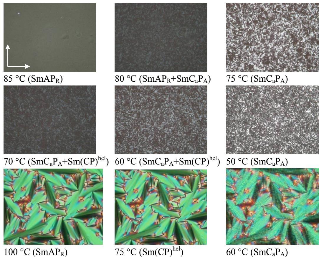
**Figure S5.** Textures as observed between crossed polarizers of compound **B10/6** depending on temperature; the upper two rows show the homeotropic textures and the bottom row the planar fan-like texture at the given temperatures in the indicated LC phases;
