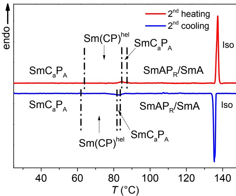
**Figure S12.** DSC heating and cooling traces of compound **B14/6** recorded at rates of 10 K min<sup>-1</sup>.
