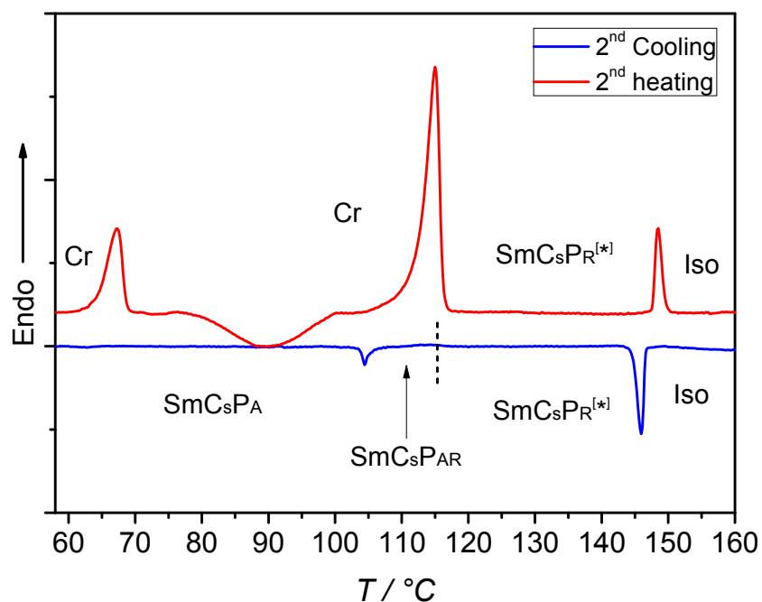
**Figure S84.** DSC heating and cooling traces of compound **EO12/O12** recorded at rates of 10 K min<sup>-1</sup>.
