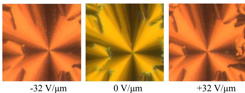
c)  $62\text{ }^{\circ}\text{C}$  ( $\text{SmC}_a\text{P}_A$  +  $\text{Sm}(\text{CP})^{\text{hel}}$ , coexistence))
