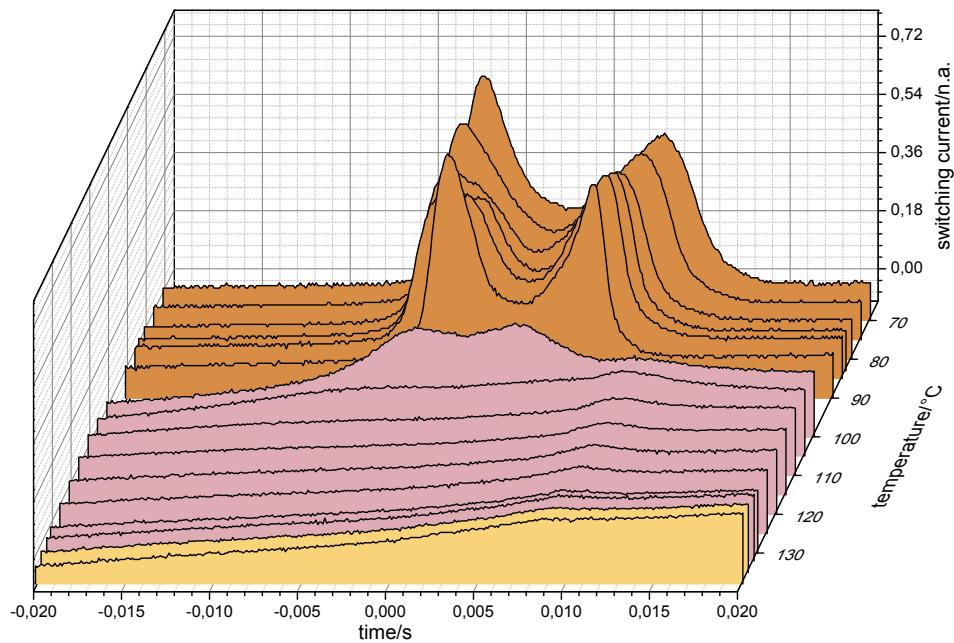
**Figure S45.** Polarization current response of **C22/12** depending on the temperature as measured in a ITO-coated cell (6  $\mu\text{m}$ ) under a triangular wave voltage of 160 V<sub>pp</sub> and a frequency of 10 Hz.
