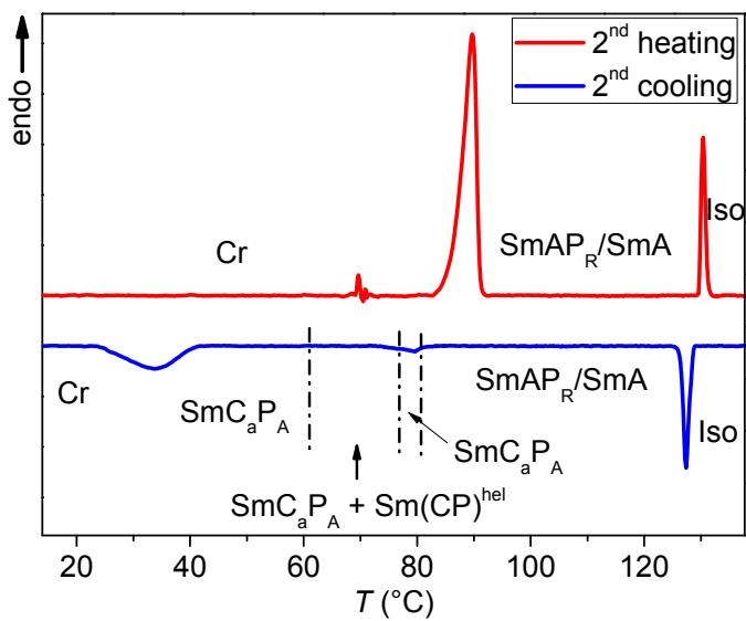
**Figure S4.** DSC heating and cooling traces of compound **B10/6** recorded at rates of 10 K min<sup>-1</sup>.
