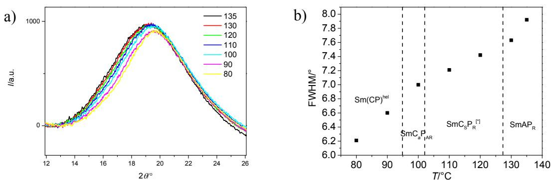
**Figure S36.** WAXD data of compound **C16/14**. a)  $2\theta$  scans and b) plot of FWHM depending on the temperature.
