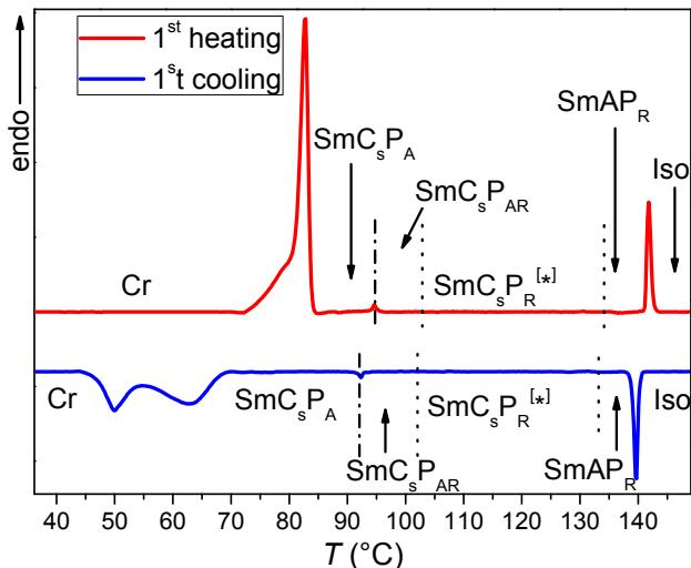
**Figure S43.** DSC heating and cooling traces of compound **C22/12** recorded at rates of 10 K min<sup>-1</sup>
