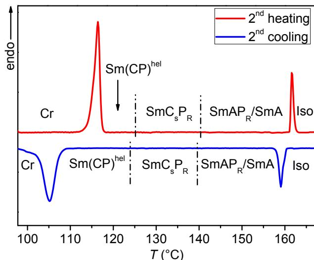
**Figure S62:** DSC traces of compound **DO22/O6** on heating and cooling at a constant rate of 10 K min<sup>-1</sup>.
