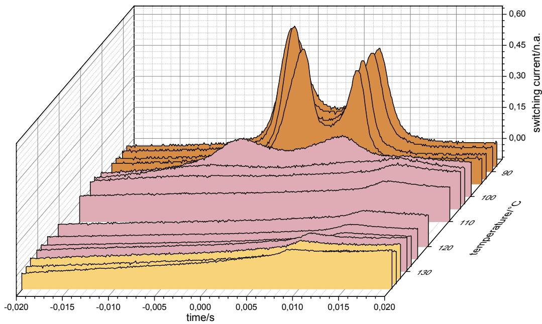
**Figure S51.** Polarization current response of **B22/18** depending on the temperature as measured in an ITO-coated cell (6  $\mu\text{m}$ ) under a triangular wave voltage of 160 V<sub>pp</sub> and a frequency of 10 Hz.
