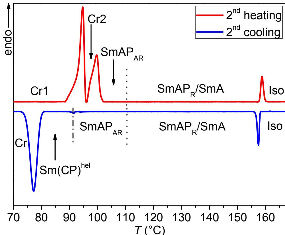
**Figure S73.** DSC heating and cooling traces of compound **DO12/14** recorded at rates of 10  $\text{K min}^{-1}$ .
