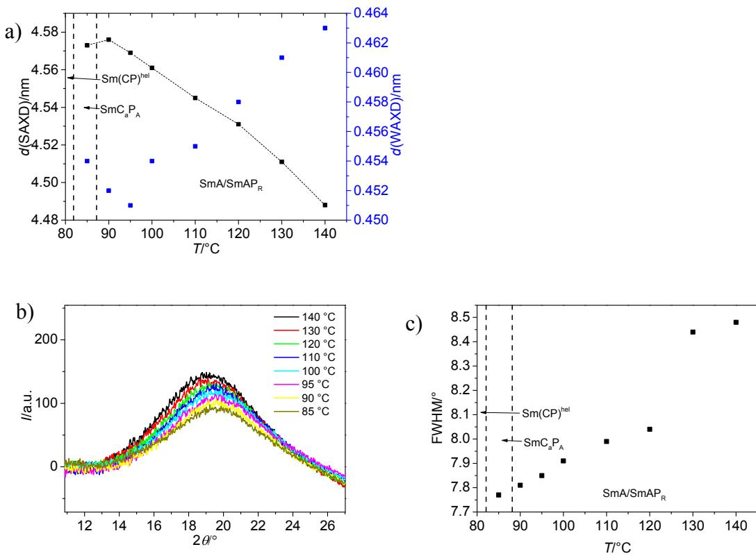
**Figure S66.** XRD data of compound **DO12/6**. a) plot of  $d$ -values of layer spacings and maxima of the wide angle scatterings depending on the temperature, b)  $2\theta$  scans of the WAXS, d) plot of FWHM depending on the temperature.
