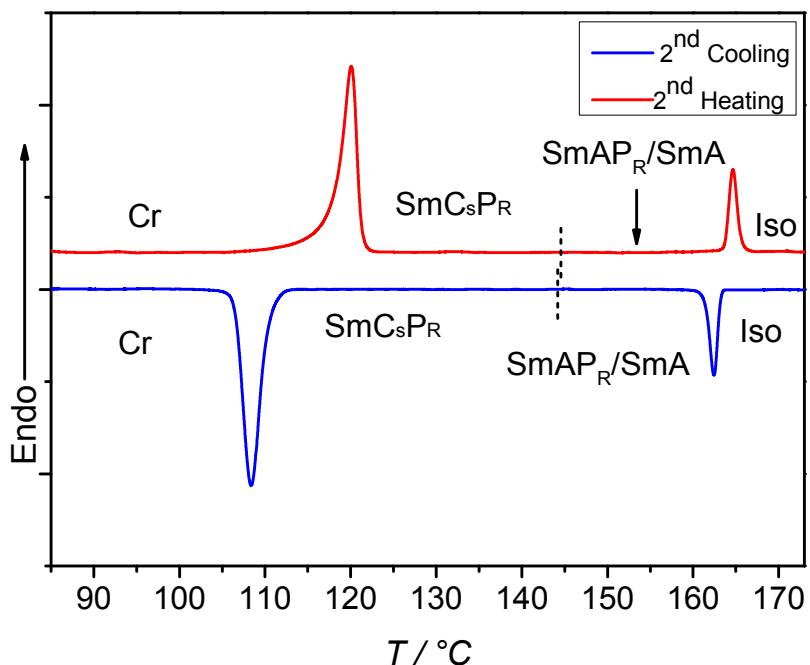
**Figure S75.** DSC heating and cooling traces of compound **DO14/O14** recorded at rates of 10  $\text{K min}^{-1}$ .
