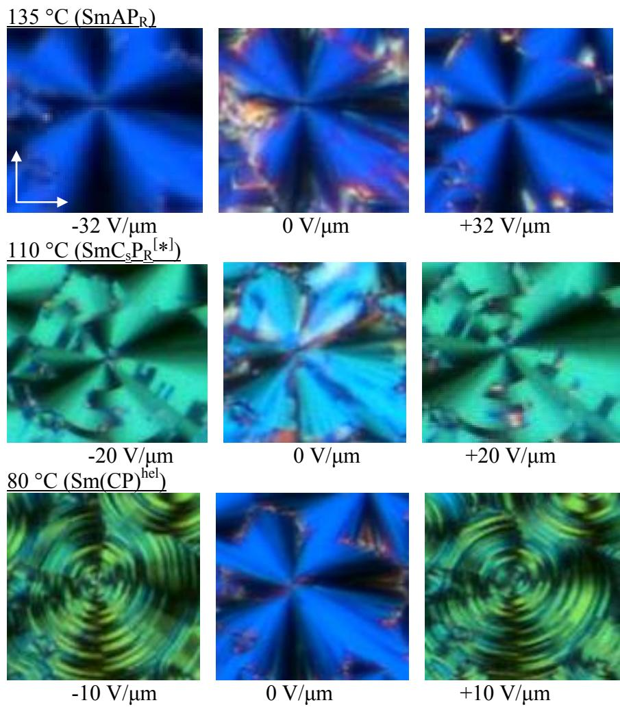
**Figure S38.** Textures of the distinct mesophases of compound **C16/14** at the given temperatures in a planar cell as observed between crossed polarizers in the ground state without applied E-field (middle) and as observed for under an applied E-field at the indicated voltages (left/right).
