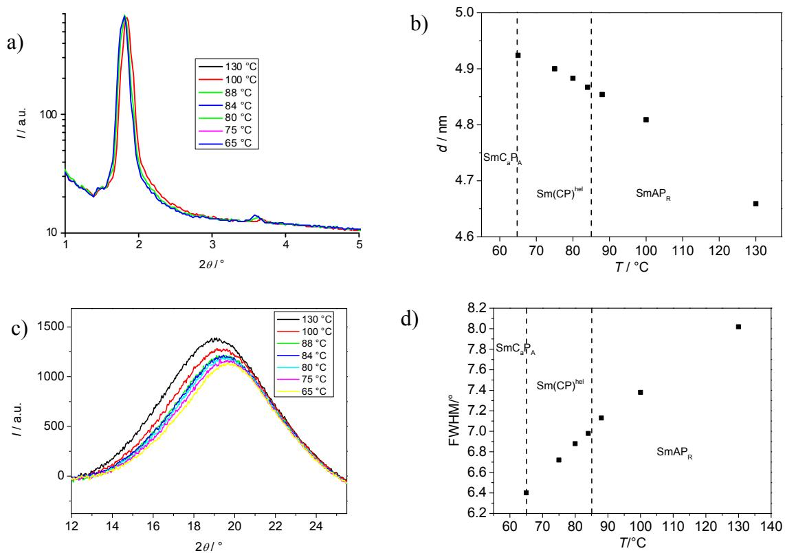
**Figure S15.** XRD data of compound **B16/6**. a) Plot of the small angle diffraction pattern; b) plot of  $d$ -values of the layer spacing depending on temperature, c)  $2\theta$  distribution and c) FWHM values of the wide angle scattering depending on the temperature.
