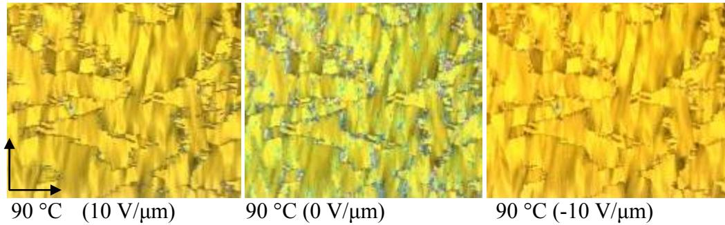
**Figure S83.** Textures of the SmC<sub>s</sub>P<sub>A</sub> phase of compound **EO12/12** in a planar cell as observed between crossed polarizers at the indicated field strengths. Though the birefringence increases in the switched states there is no change of the position of the extinctions showing the SmC<sub>s</sub>P<sub>A</sub>  $\leftrightarrow$  SmC<sub>s</sub>P<sub>F</sub> switching by rotation around the long axis.
