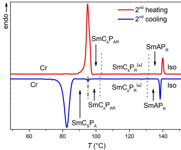
**Figure S50.** DSC heating and cooling traces of compound **C22/18** recorded at rates of 10 K min<sup>-1</sup>
