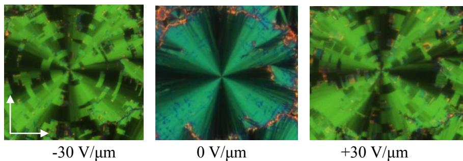
**Figure S61.** Investigation of the switching in the SmAP<sub>R</sub> phase of **DO18/O6** at  $T = 130^\circ\text{C}$  between crossed polarizers under the indicated conditions; synclinic SmC<sub>s</sub>P<sub>F</sub> states are induced under the applied field (tilt domains, left/right) which relax back at 0V to the de Vries like SmA ground state with randomized polar and tilt directions (middle).
