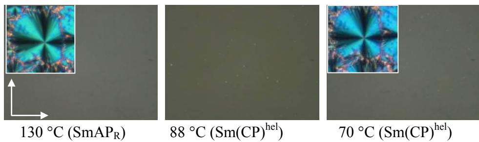
**Figure S28.** Homeotropic textures under crossed polarizers of compound **C12/12** depending on temperature; the two insets show the planar textures at the indicated temperatures.
