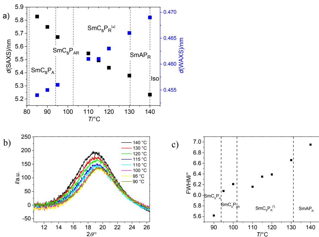
**Figure S48.** XRD data of compound **C18/18**. a)  $d$ -values of the layer spacing and of the maxima of the diffuse wide angle scattering in the XRD patterns depending on temperature; b)  $2\theta$  scans of the wide angle scatterings and c) plot of FWHM of the wide angle scatterings depending on the temperature.
