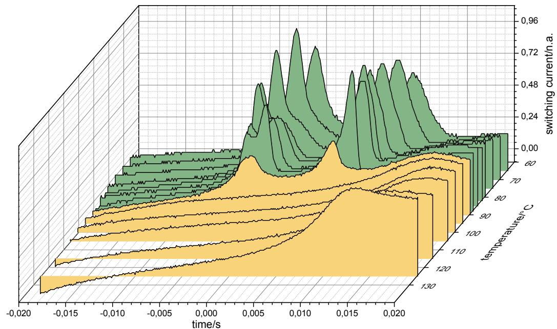
**Figure S29.** Polarization current response of **C12/12** depending on the temperature as measured in a ITO-coated cell (6  $\mu\text{m}$ ) under a triangular wave voltage of 160 V<sub>pp</sub> and a frequency of 10 Hz.
