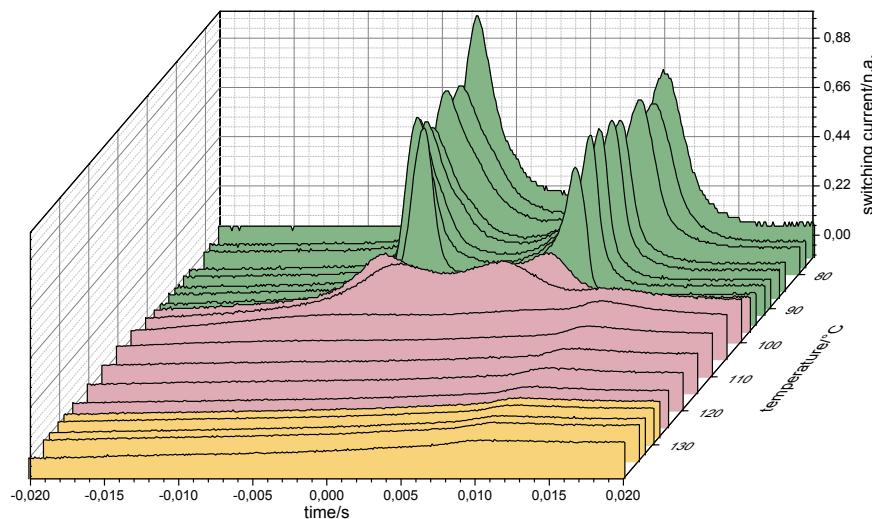
**Figure S37.** Polarization current response of **C16/14** depending on the temperature as measured in a ITO-coated cell (6  $\mu\text{m}$ ) under a triangular wave voltage of 160 V<sub>pp</sub> and a frequency of 10 Hz.
