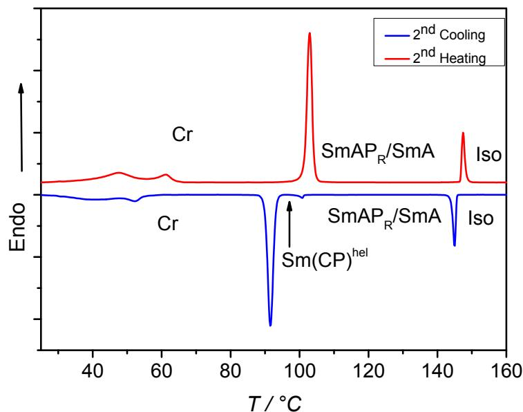
**Figure S70.** DSC heating and cooling traces of compound **D12/O12** recorded at rates of 10 K min<sup>-1</sup>.
