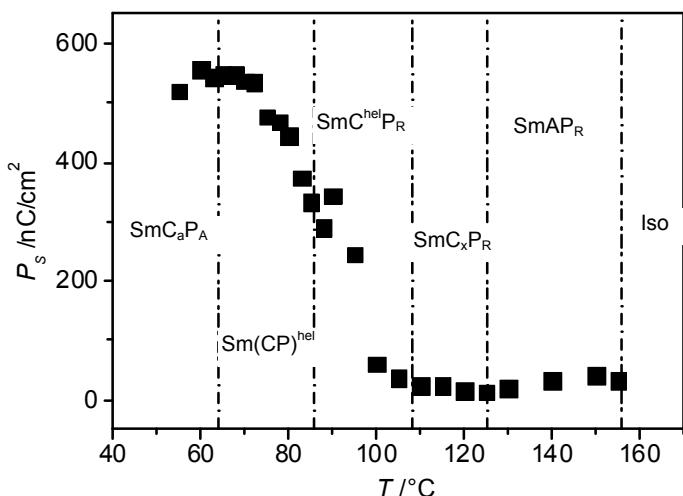
**Figure S59.** a) Polarization values compound **DO18/6** as measured depending on temperature.
