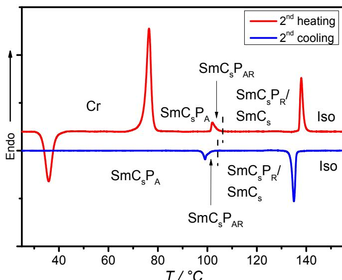
**Figure S81.** DSC heating and cooling traces of compound **EO12/12** recorded at rates of  $10\text{ K min}^{-1}$ .
