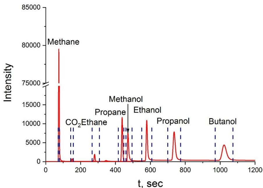
**Figure S5.** Chromatograms of possible products from the photoreduction of  $\text{CO}_2$  (red solid line); vertical blue dashed lines define the confidence intervals used for product identification within  $\pm 5\%$  of the retention time required for maximum product generation.
