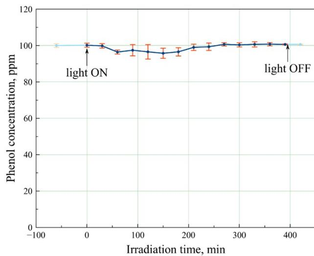
**Figure S7.** Time course of the concentration of phenol in aqueous media in the presence of Ba<sub>1.264(4)</sub>Bi<sub>1.971(4)</sub>O<sub>4</sub> as a function of irradiation time.
