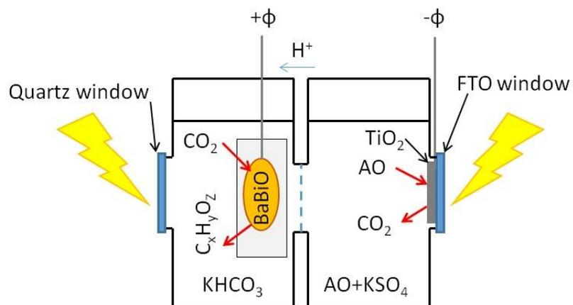
**Figure S6.** Scheme of the PEC cell for the photoelectrochemical reduction of CO<sub>2</sub>; AO is ammonium oxalate, and C<sub>x</sub>H<sub>y</sub>O<sub>z</sub> denotes various products of the CO<sub>2</sub> reduction.
