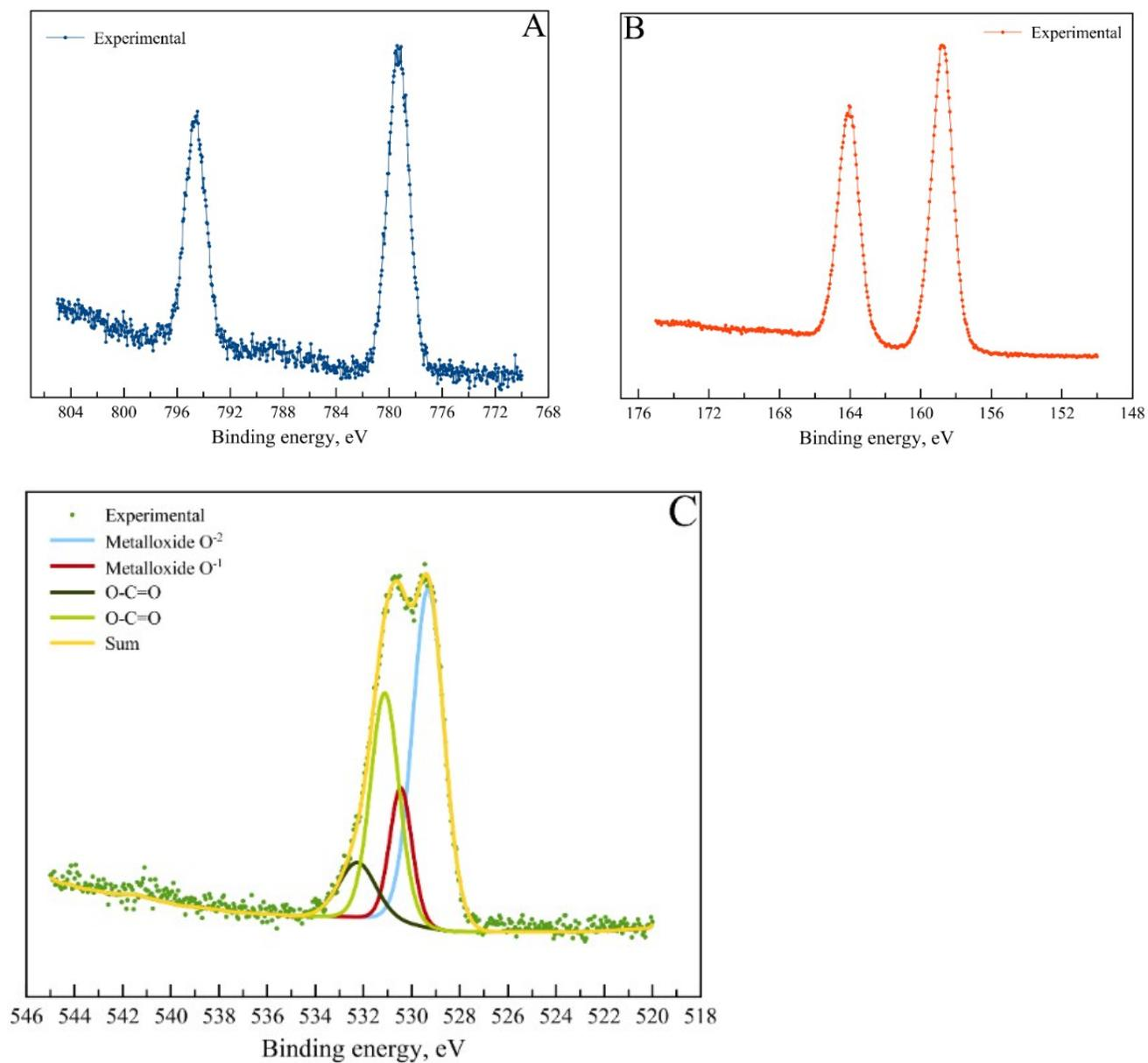
**Figure S2.** XPS spectra and deconvolution results of the synthesized barium bismuthate  $\text{Ba}_{1.264(4)}\text{Bi}_{1.971(4)}\text{O}_4$  sample in the Ba3d (A), Bi4f (B), and O1s (C) regions.
