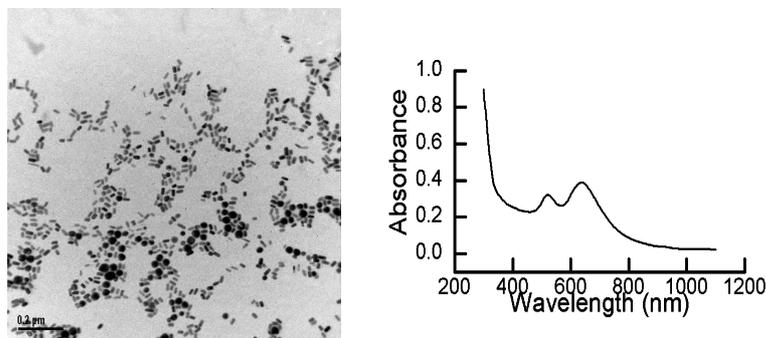
**Fig. S1** TEM image (left) and UV- spectrum (right) of short gold nanorods synthesized by the electrochemical method.
