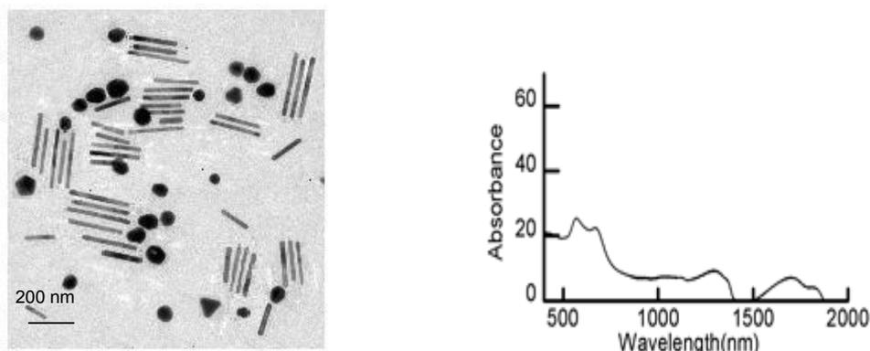
**Fig.S2 TEM and UV-near IR spectrum of long gold nanorods after subtraction of the absorbance background of water at the near IR region.**
