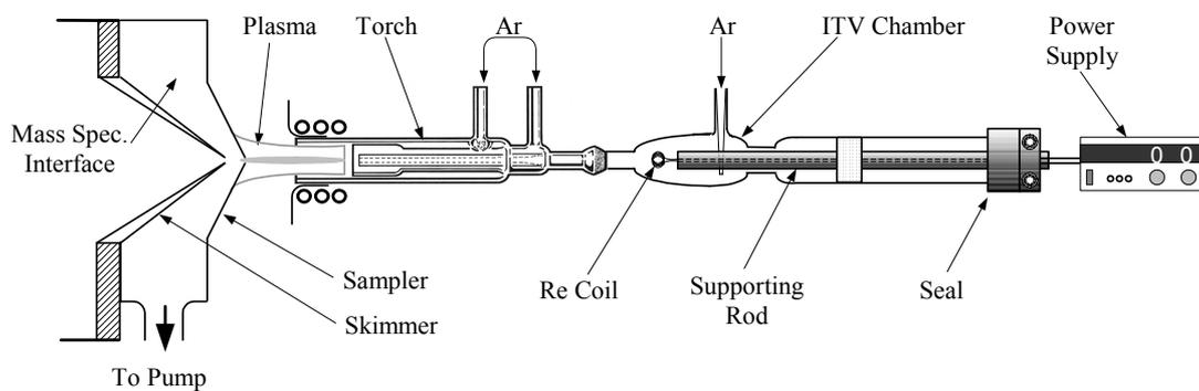
Figure S1: Schematic diagram of an ITV-ICP-MS system (illustration not to scale).
