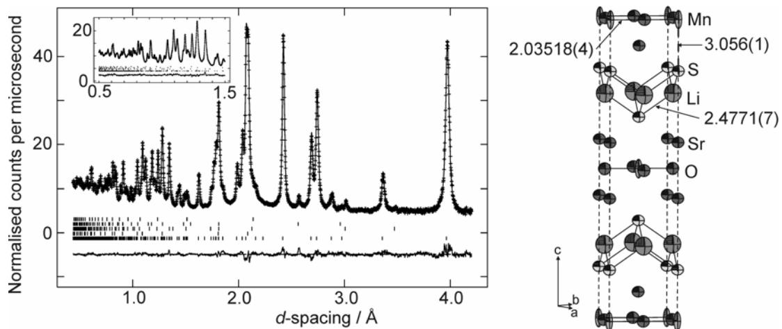
**Fig. S1.** Rietveld refinement of the structure of  $\text{Sr}_2\text{MnO}_2\text{Li}_{1.86(3)}\text{S}_2$  (**1Li**) against PND data at 295 K. Peak position markers are for (from bottom) **1Li** (bottom), Cu, small SrS and SrO impurities (~2%) and V (sample container). The structure diagram shows the unit cell with 99 % anisotropic displacement ellipsoids and selected interatomic distances in Å.
