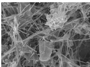
Figure 5. A SEM image of the **1c**/carbon nanofiber composite electrode.
