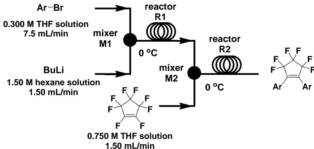
Figure 1. Microflow system for the synthesis of diarylethenes
