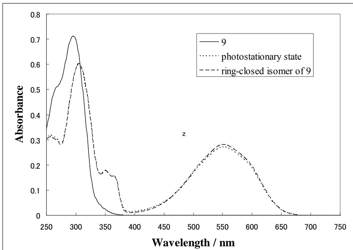
Absorption spectral change of **9** in heptane ( $2.1 \times 10^{-5}$  M) upon irradiation with 313 nm light: **9** (—), **9** in the photostationary state under irradiation with 313 nm light (·····), and the ring-closed isomer of **9** (---).
