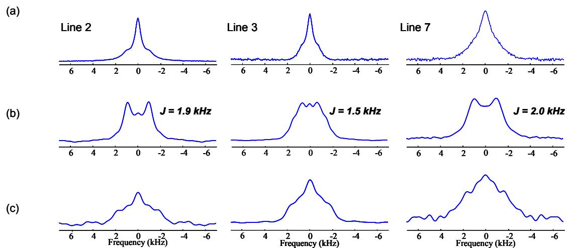
**Figure 3.** Cross-sections of the (a) 2D  $J$ -resolved, (b)  $^{207}\text{Pb}$  single-quantum filtered 2D  $J$ -resolved and (c)  $^{207}\text{Pb}$  double-quantum filtered 2D  $J$ -resolved MAS (30 kHz spinning frequency) spectra for some selected  $^{19}\text{F}$  resonances of  $\text{Pb}_5\text{Ga}_3\text{F}_{19}$ .
