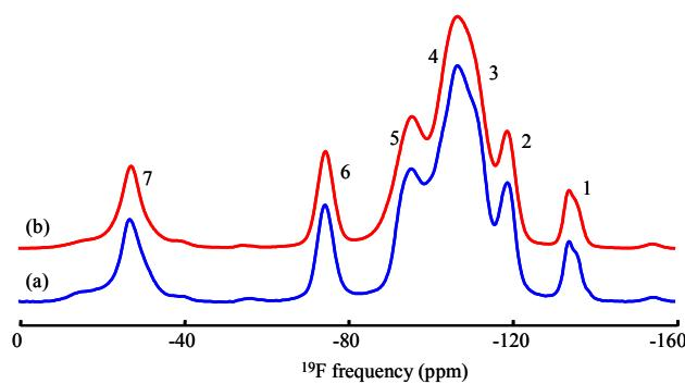
**Figure 1.** (a) experimental and (b) calculated  $^{207}\text{Pb}$  decoupled  $^{19}\text{F}$  MAS spectra of  $\text{Pb}_5\text{Ga}_3\text{F}_{19}$  at spinning rate 30 kHz.
