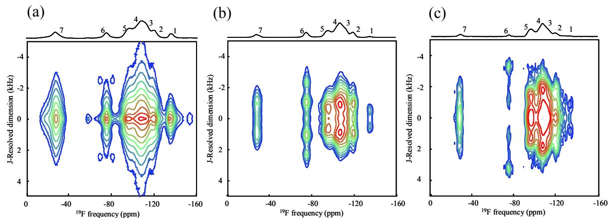
**Figure 2.**  $^{19}\text{F}$ - $^{207}\text{Pb}$  MAS (30 kHz)  $J$ -resolved spectra (a) without filtering, (b) with  $^{207}\text{Pb}$  single-quantum filtering and (c) with  $^{207}\text{Pb}$  double-quantum filtering.
