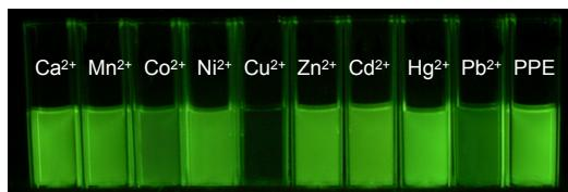
Fig. S3. Photography of solutions of PPE- $\text{CO}_2^-/\text{M}^{2+}$  ( $5 \mu\text{M} / 10 \mu\text{M}$ ) illuminated with a UV-lamp.
