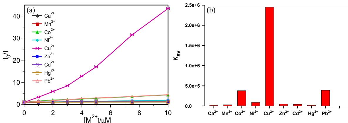
Fig. S2. (a) Stern-Volmer (SV) plot of PPE- $\text{CO}_2^-$  ( $5 \mu\text{M}$ ) titrated with different metal ions ( $M^{2+}$ ) in 0.01 M HEPES buffer solution; (b)  $K_{sv}$  Values for quenching of PPE- $\text{CO}_2^-$  with different metal ions. The  $K_{sv}$  was determined by fitting the linear region of the SV-plot.
