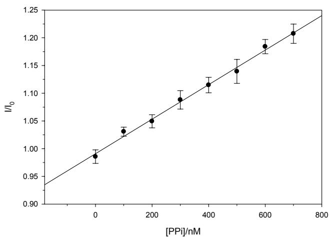
Fig. S4. Fluorescence response of PPE-CO<sub>2</sub><sup>-</sup>/Cu<sup>2+</sup> (5 μM/10 μM) to PPi in the low concentration range (0 – 700 nM). The analytical detection limit (ADL) was calculated to be 80 nM using the equation ADL = 3 δ<sub>bk</sub>/m, where δ<sub>bk</sub> is the standard deviation of the blank and m is the slope of the calibration plot.
