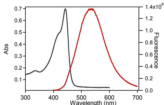
Fig. S1. Absorption (left) and emission (right) of PPE- $\text{CO}_2^-$  in 0.01 M HEPES buffer solution ( $\text{pH} = 7.5$ ),  $[\text{PPE-}\text{CO}_2^-] = 5 \mu\text{M}$ .
