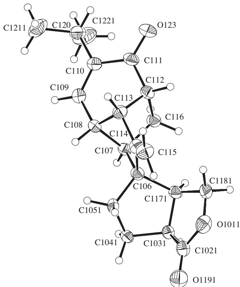
**Figure S8.** Anisotropic displacement ellipsoid plot of molecule two of compound **17** (CCDC-658576) with labeling of selected atoms. Only the major sites of disordered atoms are displayed. Ellipsoids show 30% probability levels. Hydrogen atoms are drawn as circles with small radii.
