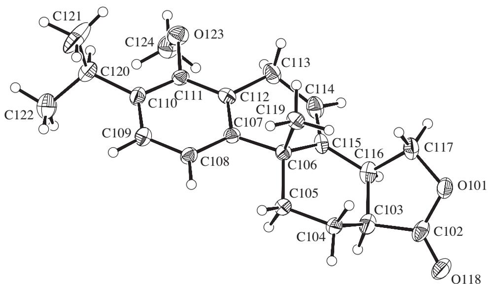
**Figure S6.** Anisotropic displacement ellipsoid plot of molecule two of compound **16** (CCDC-658575) with labeling of selected atoms. Ellipsoids show 30% probability levels. Hydrogen atoms are drawn as circles with small radii.
