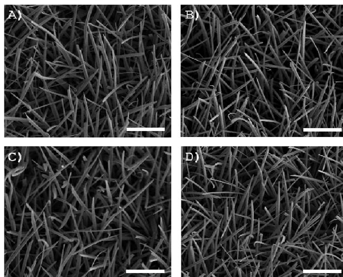
**Figure S3.** SEM images (tilt view) of vapor-deposited CN-TFMBE surfaces on various substrates: A) glass slide, B) silicon substrate, C) poly(methyl methacrylate) film on silicon substrate, D) perfluoropolymer film on silicon substrate, respectively. (scale bar is 10 $\mu$ m)
