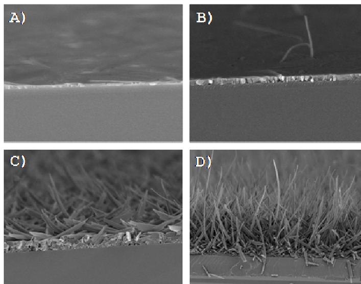
**Figure S2.** SEM images of vapor-deposited CN-TFMBE surfaces (cross-sectional view) on silicon substrates for various film thickness: A) 50nm, B) 500nm, C) 1.9  $\mu\text{m}$ , D) 8.0  $\mu\text{m}$ .
