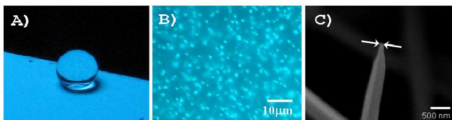
**Figure S1.** A) Photograph of the fluorescent superhydrophobic surface and a water droplet placed on the surface. The surface was excited by a 365 nm hand-held UV lamp ( $1.2 \text{ mW}\cdot\text{cm}^{-2}$ ). B) A fluorescence image of the nanostructured surface obtained by optical microscopy. C) SEM image of pine-needle-shaped (60-70nm) CN-TFMBE (a tilt view of the surface is shown)
