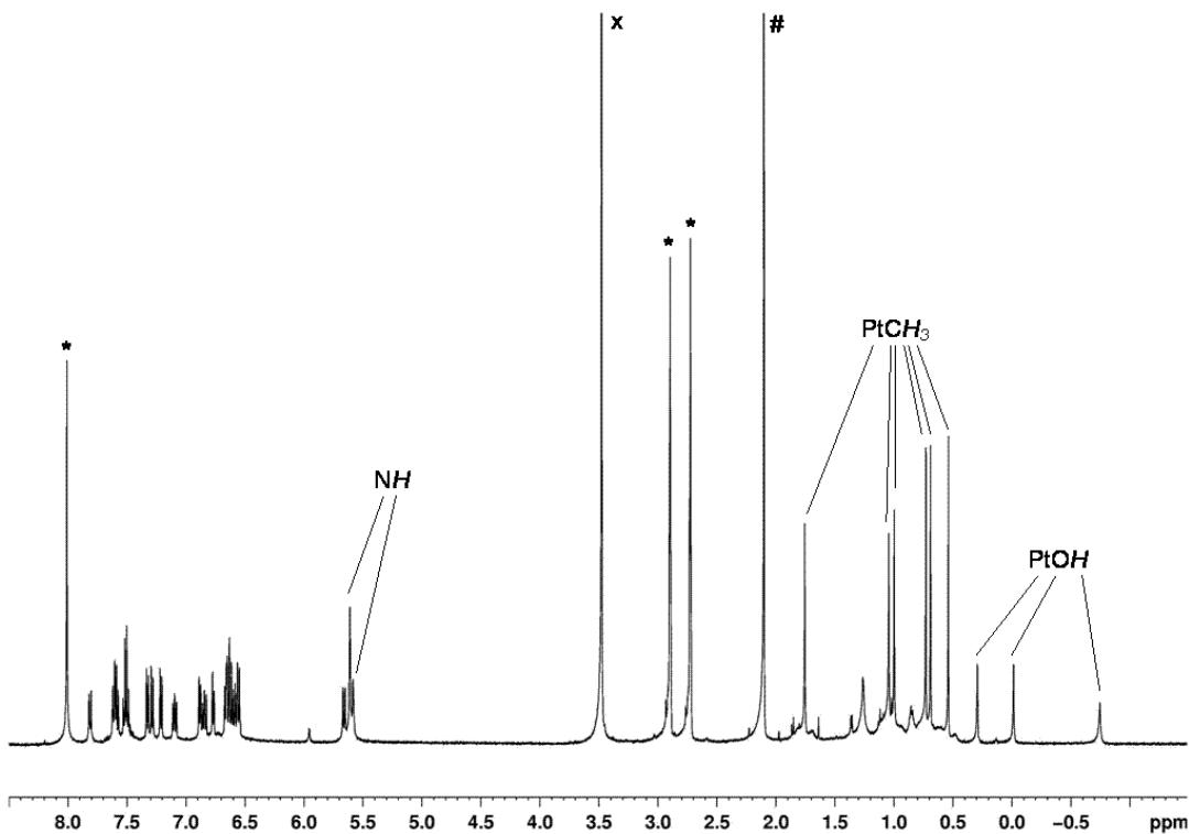
Figure S.1 <sup>1</sup>H NMR spectrum of [Pt(6,6'-diaminobipy\*)Me<sub>2</sub>(OH)]<sub>3</sub> **2** in d<sub>7</sub>-DMF. Solvent impurities: DMF (\*), acetone (#) water (x).
