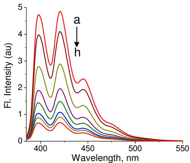
**Fig. S8** Changes in the fluorescence intensity of  $[\mathbf{1}.\text{CuCl}_2]_2$  with the addition of  $5'$ -GMP in the aqueous medium.  $[5'$ -GMP], a) 0 and h) 625  $\mu\text{M}$ .  $\lambda_{\text{ex}}$ , 379 nm.
