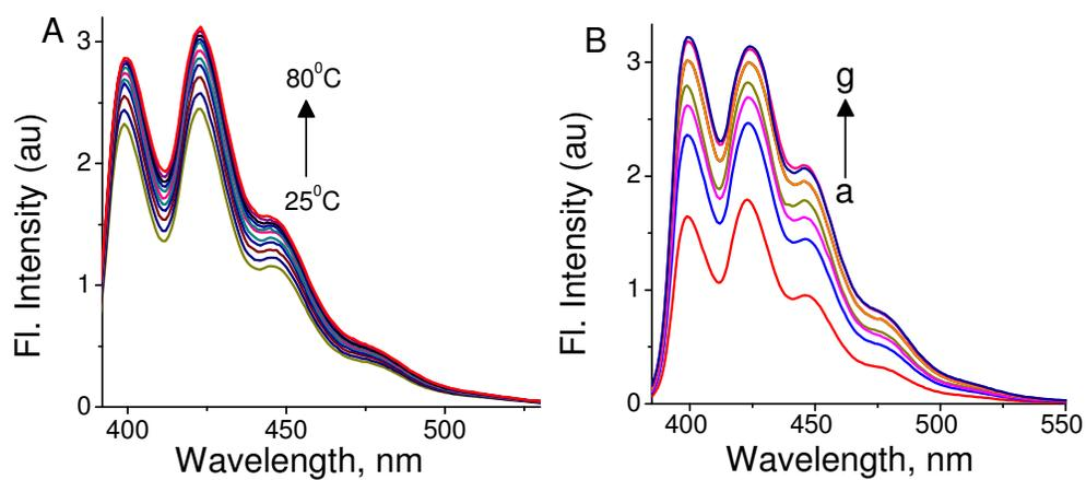
**Fig. S5** Changes in the emission spectrum of [1.CuCl<sub>2</sub>]<sub>2</sub> with A) increasing temperature and B) addition of EDTA. [EDTA] (a) 0, and (g) 625 μM.  $\lambda_{\text{ex}}$ , 379 nm.
