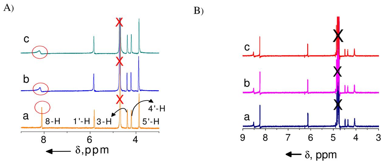
**Fig. S13** Changes in the  $^1\text{H}$  NMR spectra of A) 5'-GMP (10 mM) and B) 5'-AMP (10 mM) with the addition of the metalocyclophane  $[\mathbf{1.CuCl}_2]_2$  in  $\text{D}_2\text{O}$ .  $[\mathbf{1.CuCl}_2]_2$ , a) 0, b) 3.2, and c) 15.8  $\mu\text{M}$ .
