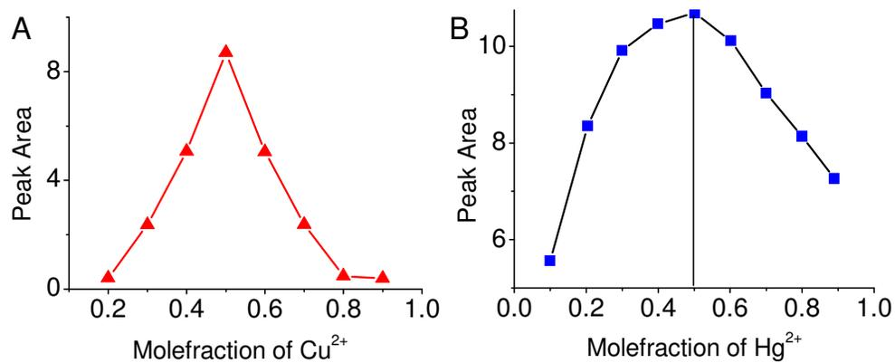
**Fig. S4** Job's plot for the binding of A) CuCl<sub>2</sub> and B) Hg(ClO<sub>4</sub>)<sub>2</sub> with the ligand **1** in 20% DMSO-water.
