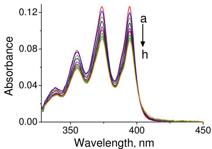
**Fig. S2** Changes in the absorption spectrum of the ligand **1** (20 μM) with the addition of CuCl<sub>2</sub> in 20% DMSO–water. [CuCl<sub>2</sub>], a) 0, and h) 156 μM.
