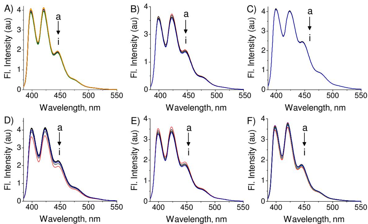
**Fig. S10** Changes in the fluorescence spectrum of the metallocyclophane [1.CuCl<sub>2</sub>]<sub>2</sub> with the addition of A) 5'-AMP, B) adenosine, C) 5'-ATP, D) 5'-GDP, E) guanosine and F) 5'-GTP in the aqueous medium. [Ligand], (a) 0, and (i) 625 μM.  $\lambda_{\text{ex}}$ , 379 nm.
