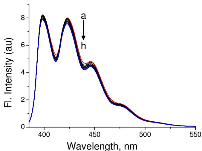
**Fig. S9** Changes in the fluorescence intensity of [1.Hg(ClO<sub>4</sub>)<sub>2</sub>] with the addition of 5'-GMP. [5'-GMP], a) 0 and h) 625 μM.  $\lambda_{\text{ex}}$ , 379 nm.
