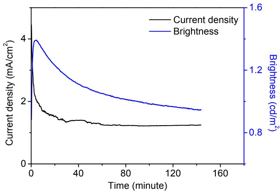
**Figure S9.** Current-density and brightness versus time at 3 V for the LEC based on complex 2.
