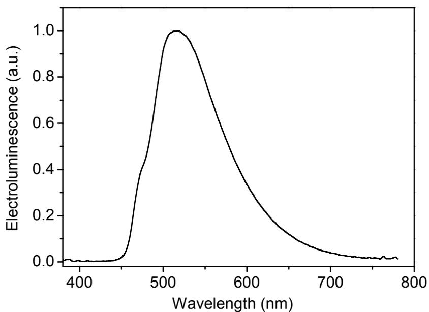
**Figure S8.** EL spectrum of the LEC based on complex 2.
