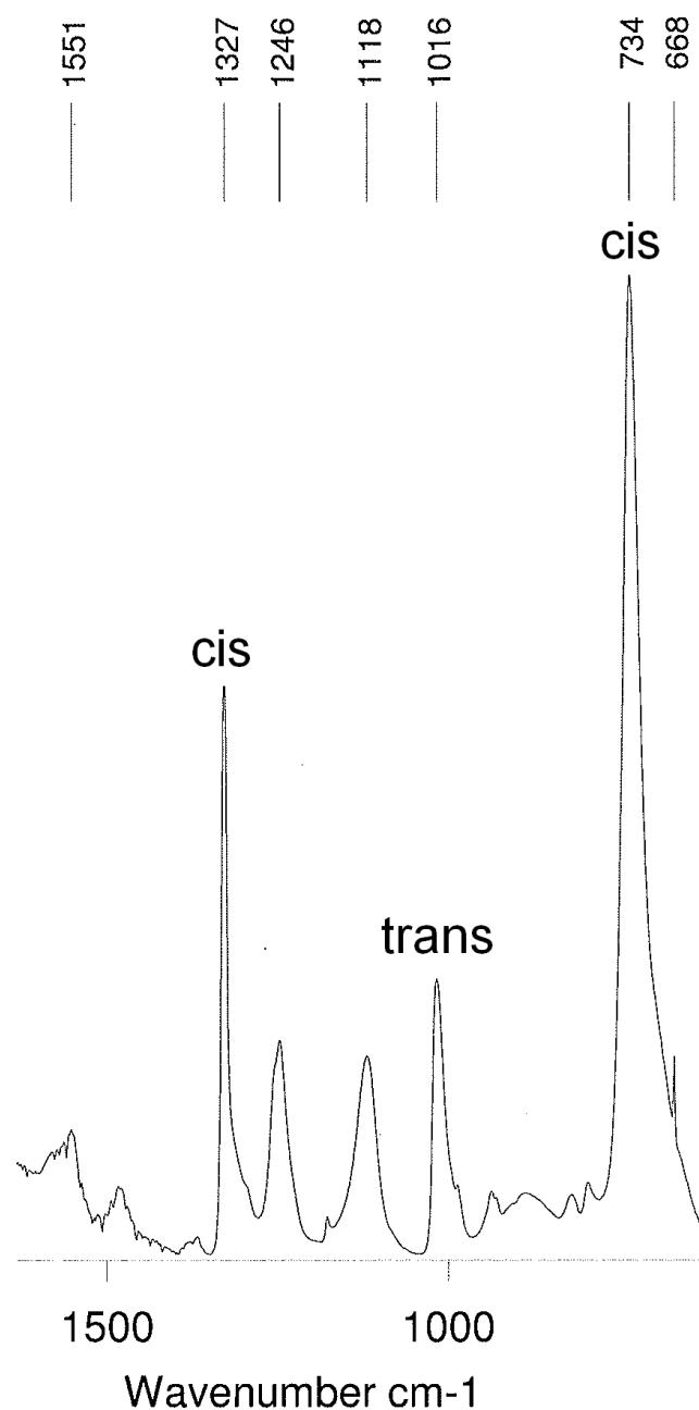
**Figure S1.** IR spectrum (C-H deformation region) of a polyacetylene film formed by 1/MAO in toluene.
