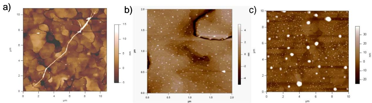
**Fig. S5** TM-AFM images of dropcast MCH solutions ( $c = 1 \times 10^{-5}$  M) (a) **OPV-s** (b) **OPV** and (c) **OPV-s** after rinsing with pure MCH on a gold substrate.
