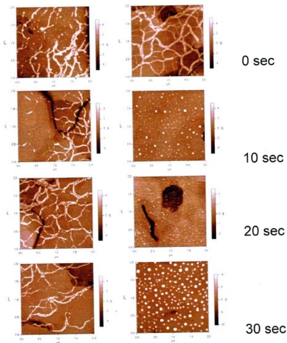
**Fig. S7** Stability of **OPV-s** (left column) and **OPV** (right column) monolayers on gold surface illustrating the capabilities to transfer efficiently the self-assembled fibrils. In a first step, the monolayers were formed by drop casting a molecularly dissolved state (from chloroform solution) on the gold substrate. In a second step the fibrils are deposited from MCH on the substrate and then exposed to chloroform. The rinsing times were 0, 10, 20 and 30 seconds, respectively.
