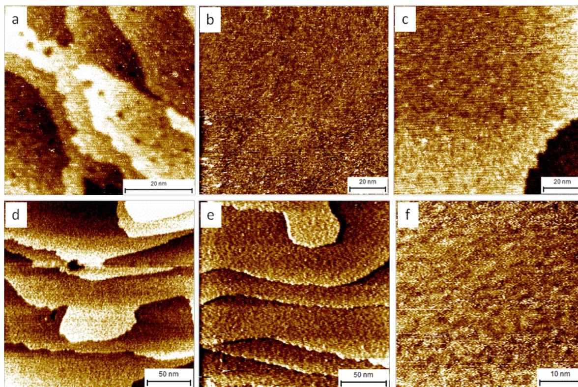
**Fig. S4** STM images obtained after dropcasting **OPV-s** on a gold substrate from TCB (a-b) or from tetradecane (d-f).  $I_{\text{set}}=161\text{pA}$ ,  $V_{\text{set}}=-412\text{mV}$ . The STM-images at both the TCB/HOPG and the tetradecane/HOPG interface are quite unclear but suggest that the surface is randomly covered with molecules.
