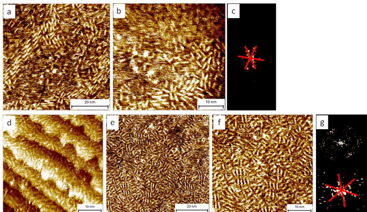
**Fig. S2** STM images of OPV monolayers on a gold substrate formed upon dropcasting from TCB (a-b) or tetradecane (d-f).  $I_{\text{set}}=161\text{pA}$ ,  $V_{\text{set}}=-412\text{mV}$ . The STM images at both the TCB/HOPG and the tetradecane/HOPG interface show a disordered pattern with some dimer formation. c) and g) show the 2D fast Fourier transform of the STM images in TCB and tetradecane, respectively. These indicate that the dimer rows follow approximately three main directions.
