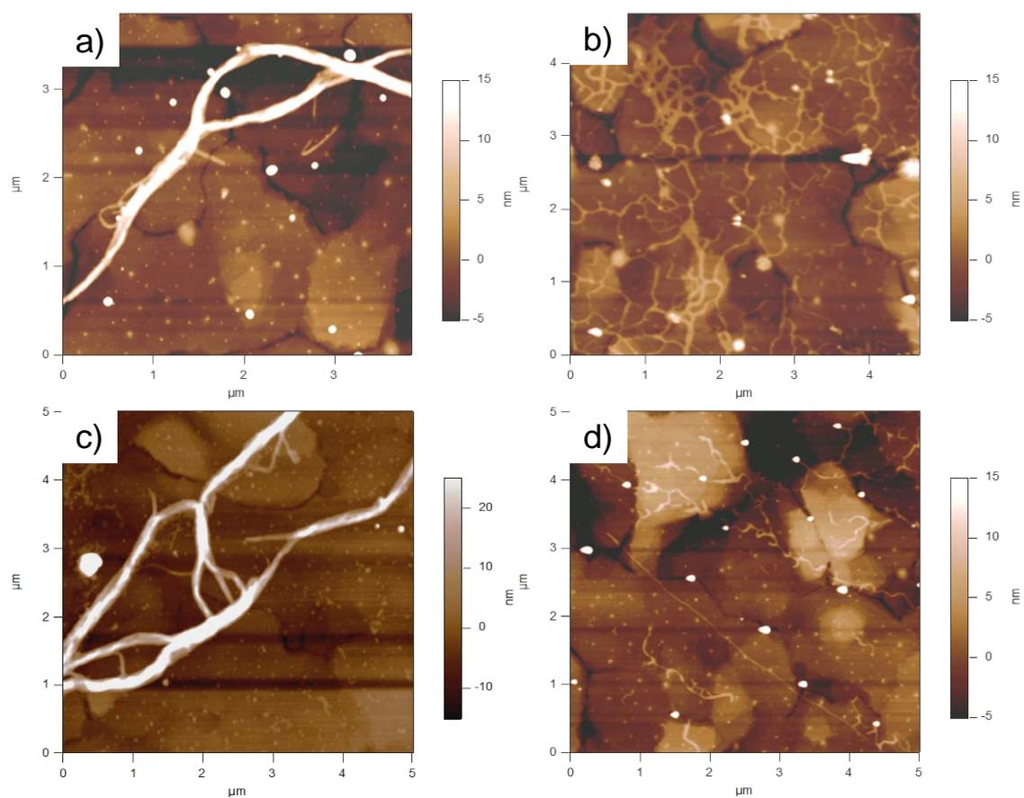
**Fig. S8** TM-AFM images on a gold substrate after dropcasting a MCH solution of either **OPV-s** (a, c) or **OPV** (b, d) on a substrate having a monolayer of **OPV-s** (a,b) or of **OPV** (c,d).
