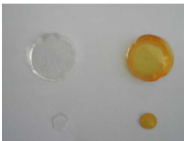
Fig 2S – Membranes photographs before and after conditioning in 10 mM of \text{Ru}(\text{bpy})_3^{2+} used for the transport experiments (top, 10 mm diameter) and potentiometric measurements (bottom, 3 mm diameter).
