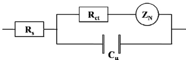
Fig. S2 Equivalent circuit of the symmetrical cells.  $R_s$ , series resistance;  $R_{ct}$ , charge transfer resistance in the electrode/electrolyte interface;  $C_\mu$ , corresponding capacitance in the electrode/electrolyte interface; and  $Z_N$ , Nernst diffusion impedance.
