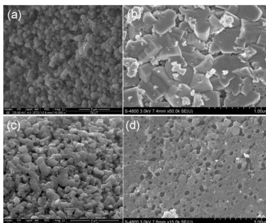
Fig. S1 SEM images of the as-prepared Nb<sub>2</sub>O<sub>5</sub> and NbO<sub>2</sub> samples. (a) H-Nb<sub>2</sub>O<sub>5</sub>, (b) O-Nb<sub>2</sub>O<sub>5</sub>, (c) M-Nb<sub>2</sub>O<sub>5</sub>, and (d) T-NbO<sub>2</sub>.
