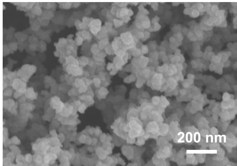
**Fig. S1** SEM image of Pd nanoparticle networks prepared in the absence of  $\text{Cu}^{2+}$ . It was found that Pd porous network structure composed of nanoparticles with an average size of 50 nm was obtained in the absence of  $\text{Cu}^{2+}$  and other conditions kept unchanged.
