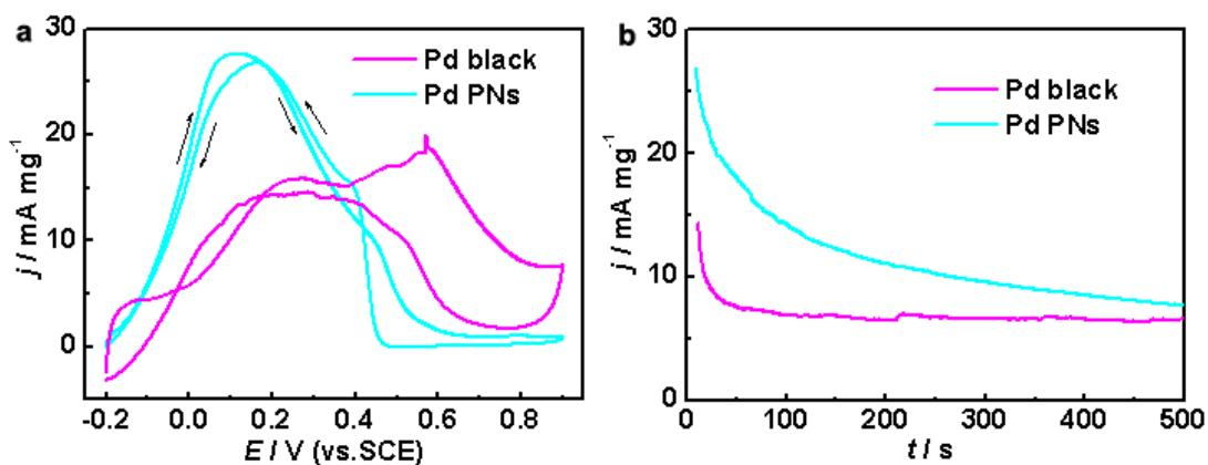
**Fig. S3** CV curves at a scan rate of 0.05V/s (a) and chronoamperometric curve at 0.1V (vs. SCE) (b) of Pd black and Pd PN in 0.1 M  $\text{HCOOH}$  + 0.1M  $\text{H}_2\text{SO}_4$ . The currents were normalized to the amount of Pd catalysts. The arrows in CVs (a) indicate the potential scan direction.
