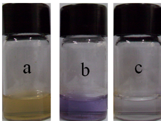
Fig. S2. Verification of amino-group (a. Ag@SiO 2 NPs without functionalization dispersed in water; b. Ag@SiO 2 NPs functionalized with -NH 2 dispersed in water; c. the supernatant liquid of b after centrifugation.).
