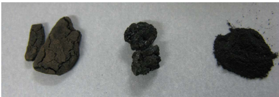
Figure S32 The images of reacted catalyst. The left image is Pd/AC, and the middle image is Pt/AC, the right image is Ni/AC.
