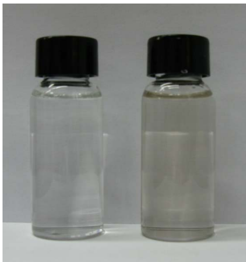
Figure S 31 Detection of evolved gas from a reaction with Pd/C as catalyst. The left image is the original 1 mol L -1 Pb(AC) 2 solution. The right image is the reacted Pb(AC) 2 solution. The reaction indicates that there is no H 2 S coming out of the reaction system.
