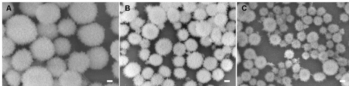
**Figure S4.** SEM images of  $\text{CePO}_4:\text{Tb,Gd}$  obtained at different reaction time: (A) 6 h, (B) and (C) 12 h.
