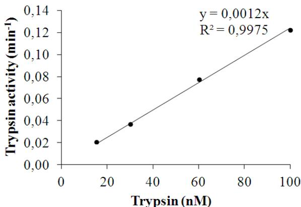
**Fig. S2** Calibration curve of trypsin between 15 and 100 nM in 50 mM TRIS HCl + 10 mM CaCl<sub>2</sub> pH 8.0. Data are the mean from three independent measurements for each concentration.
