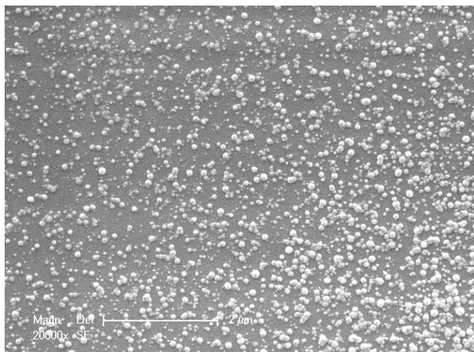
**Fig. S1** SEM of the MIP-NPs.
