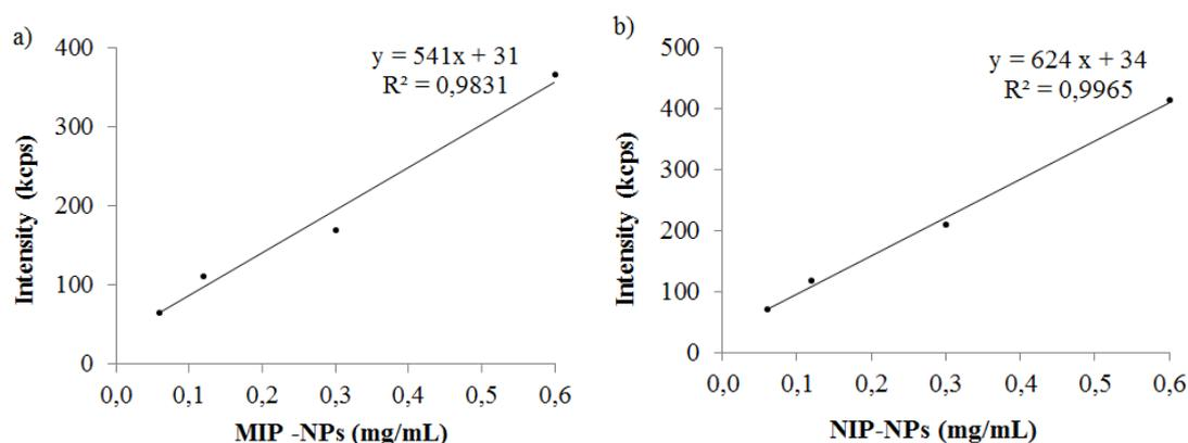
**Fig. S3** Calibration curves of (a) MIP-NPs and (b) NIP-NPs between 0.06 and 0.6 mg/mL in 5 mM TRIS HCl + 10 mM CaCl<sub>2</sub> pH 8.0. Data are the mean from three independent measurements for each concentration.
