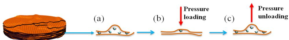
**Scheme S1.** Schematic illustration of the pressure loading and releasing process: (a) initial state; (b) pressure loading and shrinking of the channel; (c) pressure releasing and recovery of the channel.
