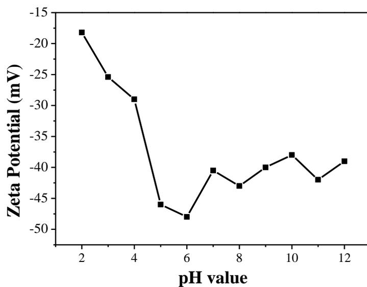
**Fig. S3.** Zeta potential of 0.02 mg ml<sup>-1</sup>GO suspension depends on pH.
