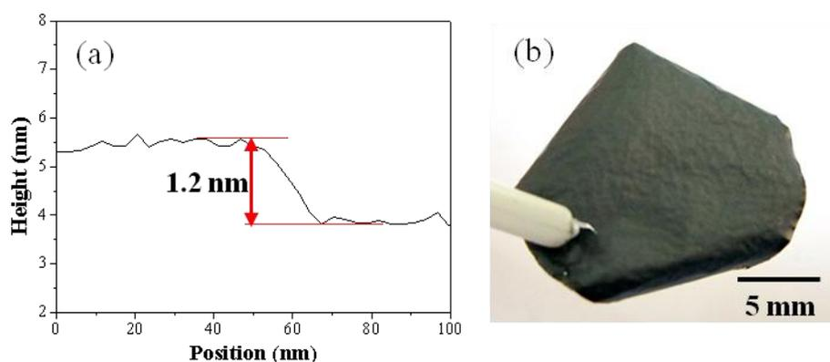
**Figure S1** (a) the thickness profile from the AFM image as marked in main text Figure 1a. (b) Photo image of the free-standing GO membrane prepared from 3 ml 0.02% GO dispersion.
