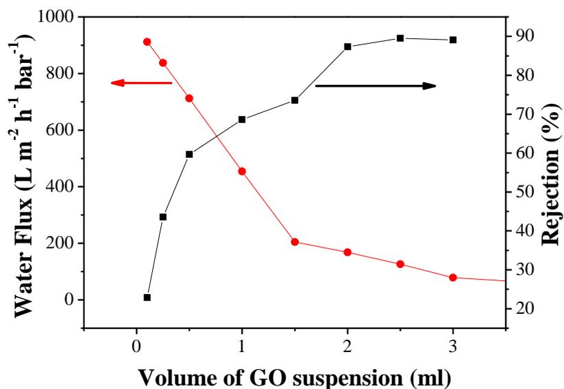
**Fig. S2.** The water flux and rejection rate of EB molecules of GO membrane prepared from different volume of 0.02 mg ml<sup>-1</sup> GO suspension.
