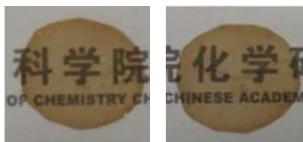
Figure S6. Demonstration of thermo-stability of a FPEEK-QD film (containing red-emitting QDs). (a) Fluorescence spectra. Up: excitation, down: emission. (b) Optical image of the FPEEK-QD film upon an annealing at 150 °C for 30 min. Left: before annealing, Right: after annealing. For the annealed film, the fluorescence spectra and the photograph were taken after the film was cooled down to ambient temperature.
