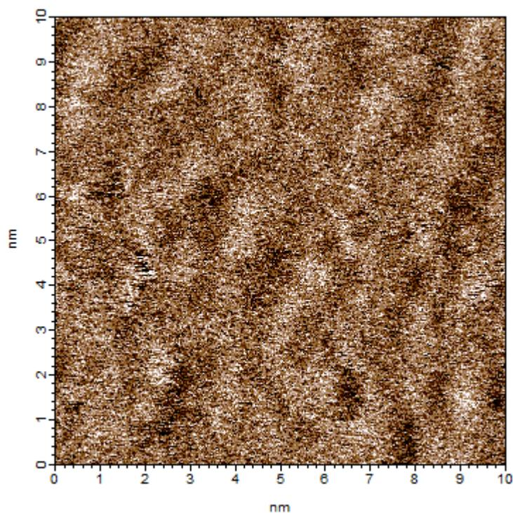
**Figure A.** A contact mode AFM image of a transition zone layer in the PAN-mica system. The slow scan direction is up the image.
