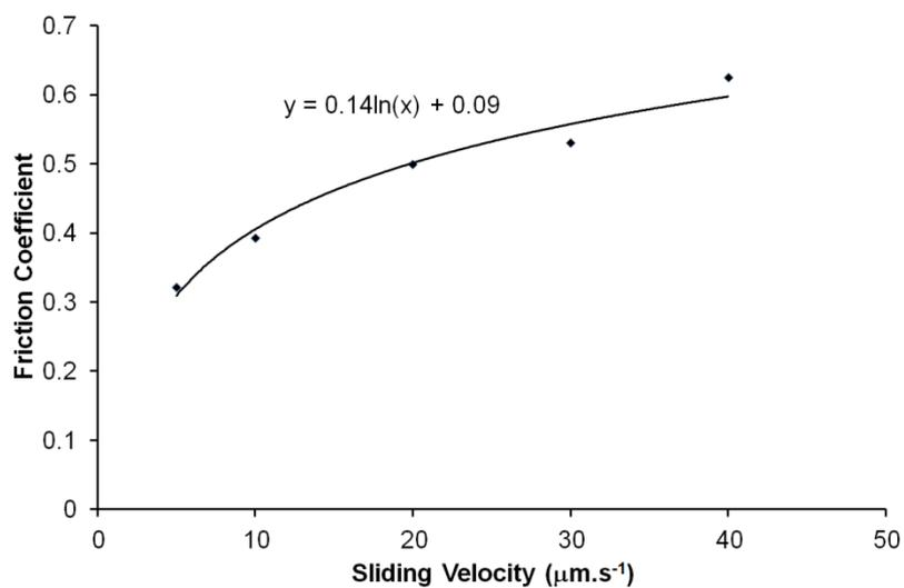
**Figure E.** Colloid probe speed dependant friction coefficient for Region II.
