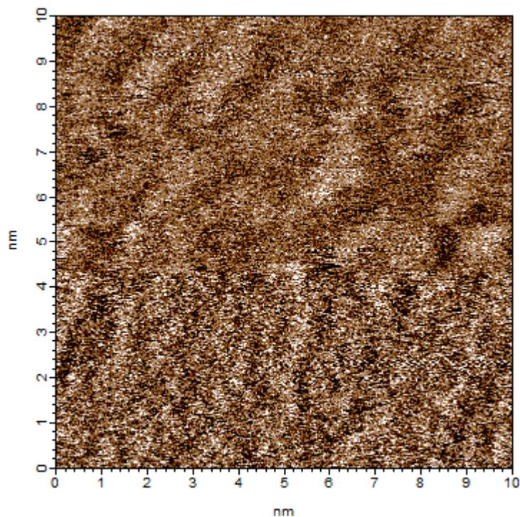
**Figure B.** A contact mode AFM image of the transition from a near surface layer (top) to the innermost layer (bottom) in the PAN-mica system. The slow scan direction is down the image.
