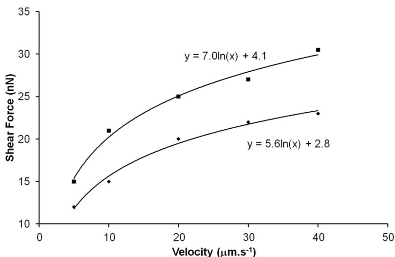
**Figure D.** Representative plots of shear force versus colloid probe sliding velocity at 20 nN (diamonds) and 32 nN (squares) that demonstrate the logarithmic dependency of shear force with sliding velocity.
