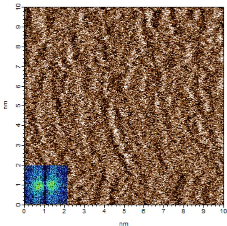
**Figure C.** A contact mode AFM image of the innermost layer of the PAN-mica system. The slow scan direction is up the image. The inset gives the 2D Fourier transform, indicating that the interaggregate periodicity repeat length is  $5 \pm 0.3 \text{ \AA}$ .
