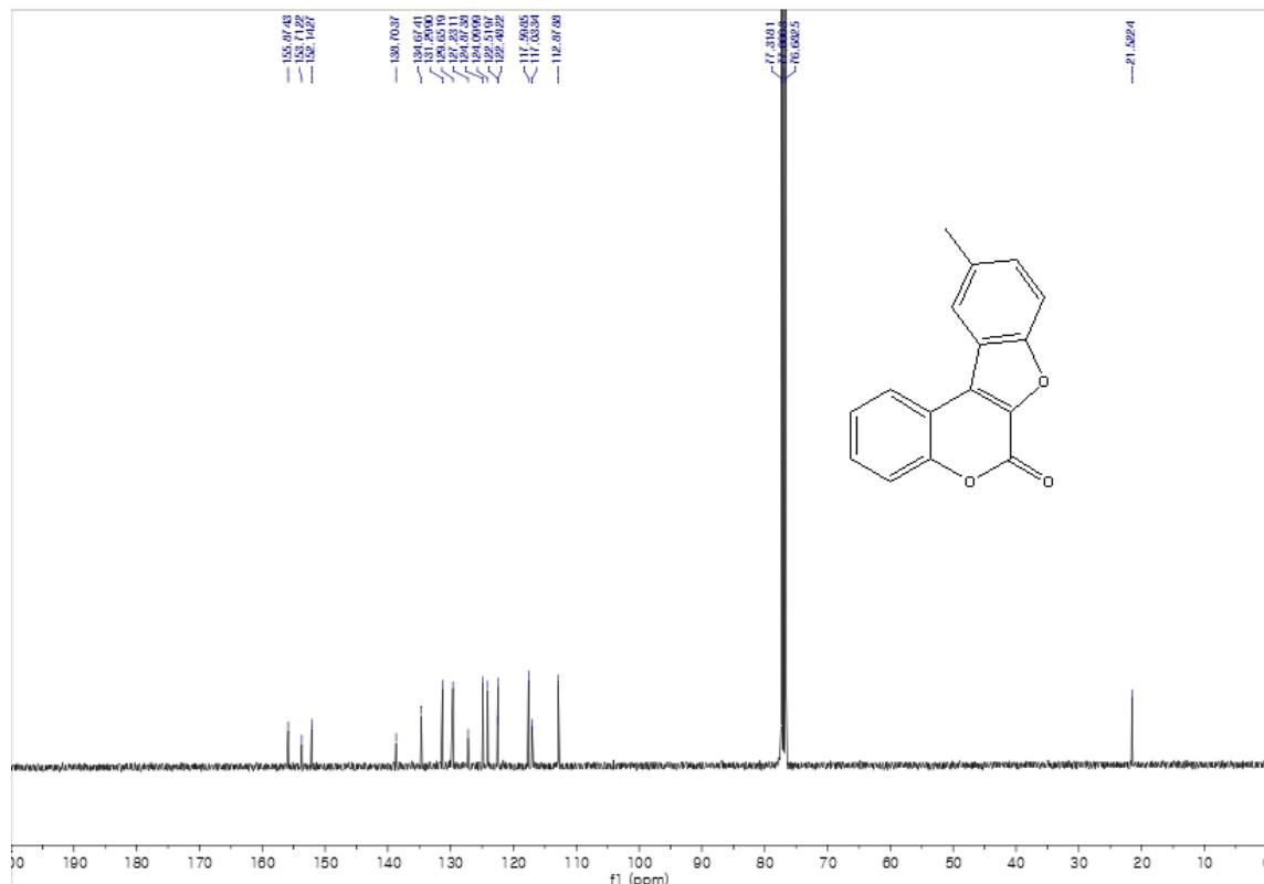
100 MHz, <sup>13</sup>C NMR in CDCl<sub>3</sub>
