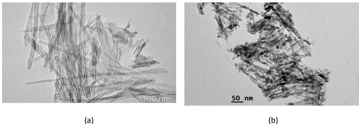
Fig. S2 TEM images of (a) TNT (b) CuTNT-4 photocatalysts
