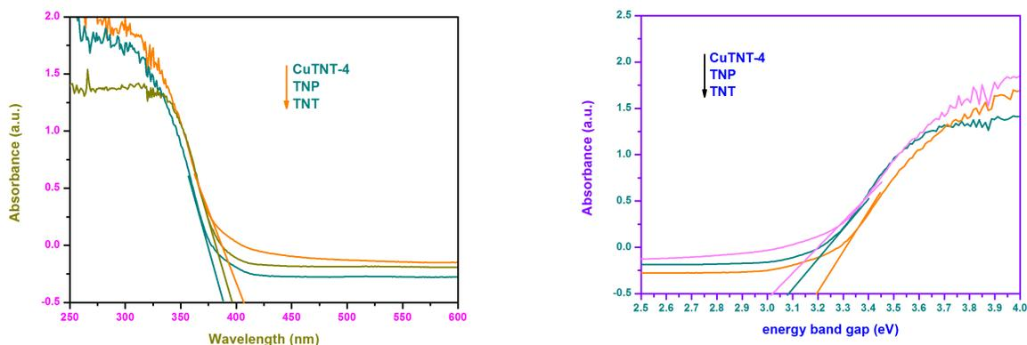
Fig. S3 DRS UV-Vis spectrum of TNP, TNT and CuTNT-4 photocatalysts
