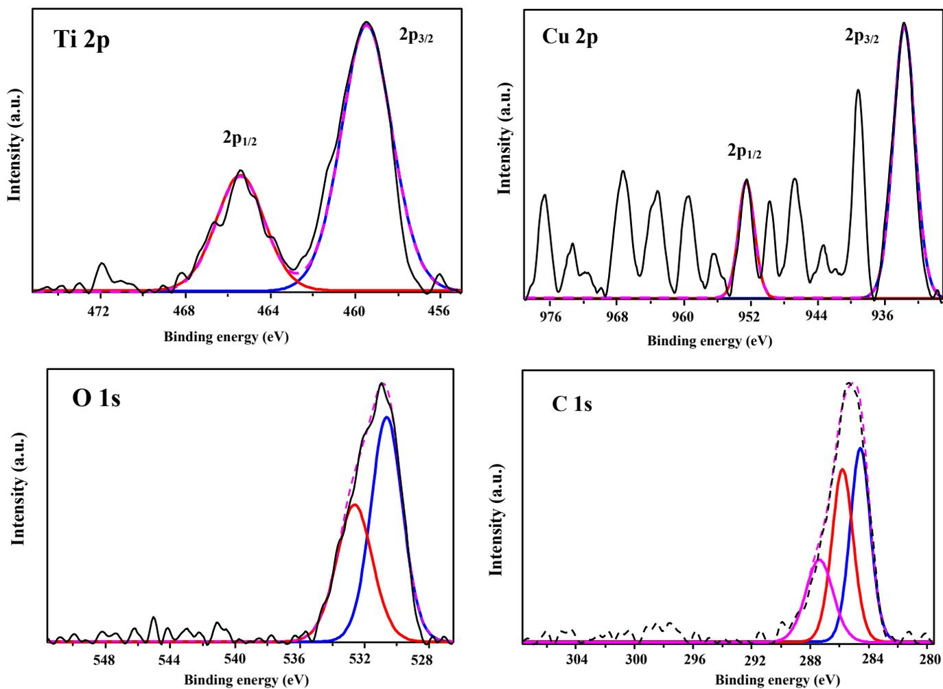
**Fig. S4** XPS spectra of CuTNT-4 photocatalyst.
