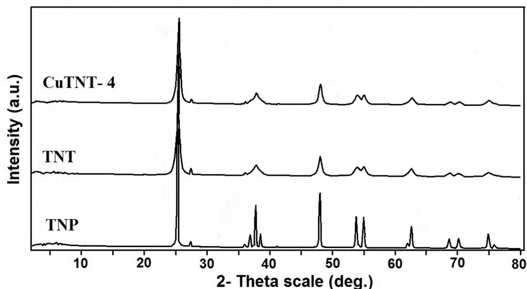
Fig. S1 XRD patterns of TNP, TNT and CuTNT-4 photocatalysts
