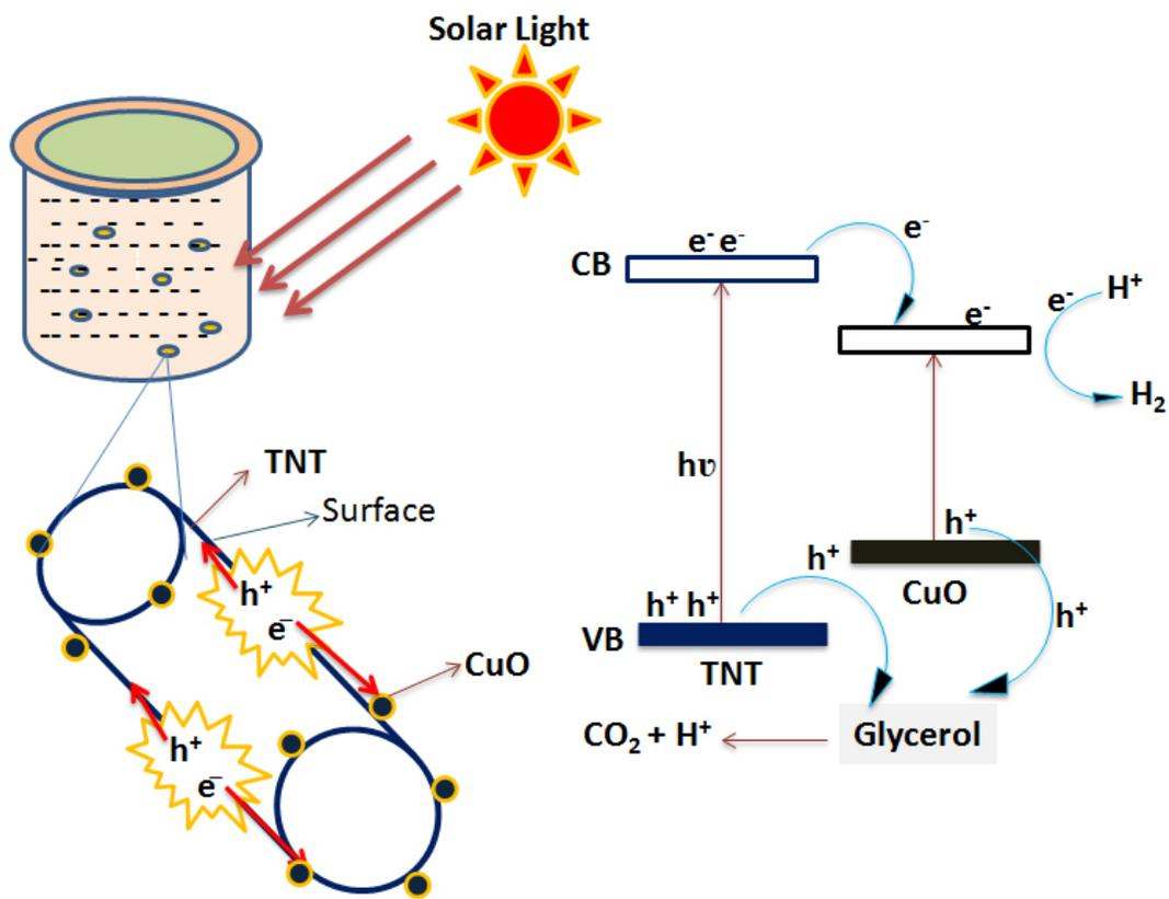
**Fig. S6** Schematic diagram of band gap excitation and charge transfer processes in solar photocatalytic H<sub>2</sub> generation.
