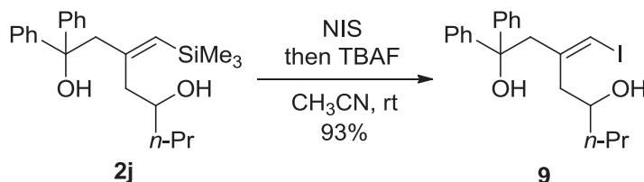
*N*-Iodosuccinimide (70 mg, 0.3 mmol) was added to a solution of **2j** (60 mg, 0.15 mmol) in CH<sub>3</sub>CN
