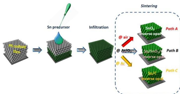
**Figure S1.** A schematic diagram of the p-IO Sn/C, p-IO Sn/SnO<sub>2</sub>/C, and IO SnO<sub>2</sub> syntheses.
