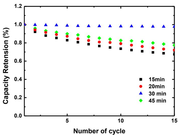
**Figure S4.** The 0.5C discharge cycle performance of p-IO Sn/SnO<sub>2</sub>/C with different sintering time under 4 vol% oxygen in Ar.
