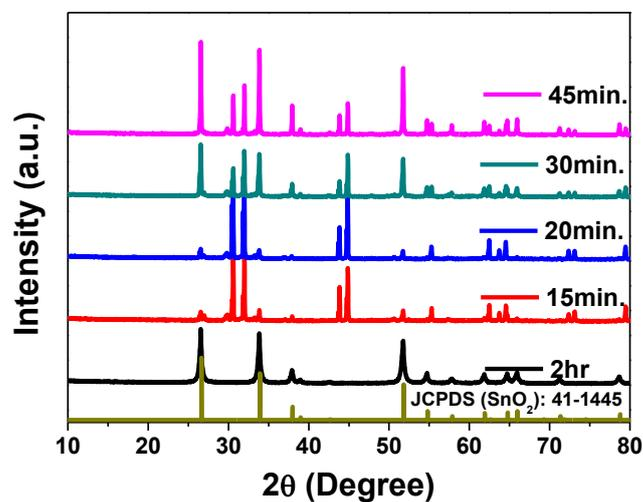
**Figure S3.** XRD patterns of p-IO Sn/SnO<sub>2</sub>/C as a function of sintering time under 4 vol% oxygen in Ar.
