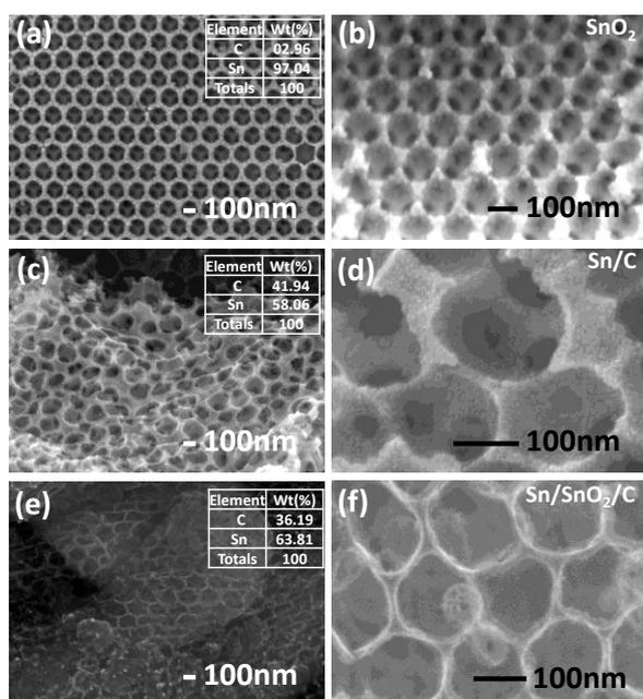
**Figure S6.** SEM images and the elemental ratios of IO SnO<sub>2</sub> (a–b), p-IO Sn/C (c–d), and p-IO Sn/SnO<sub>2</sub>/C (e–f).
