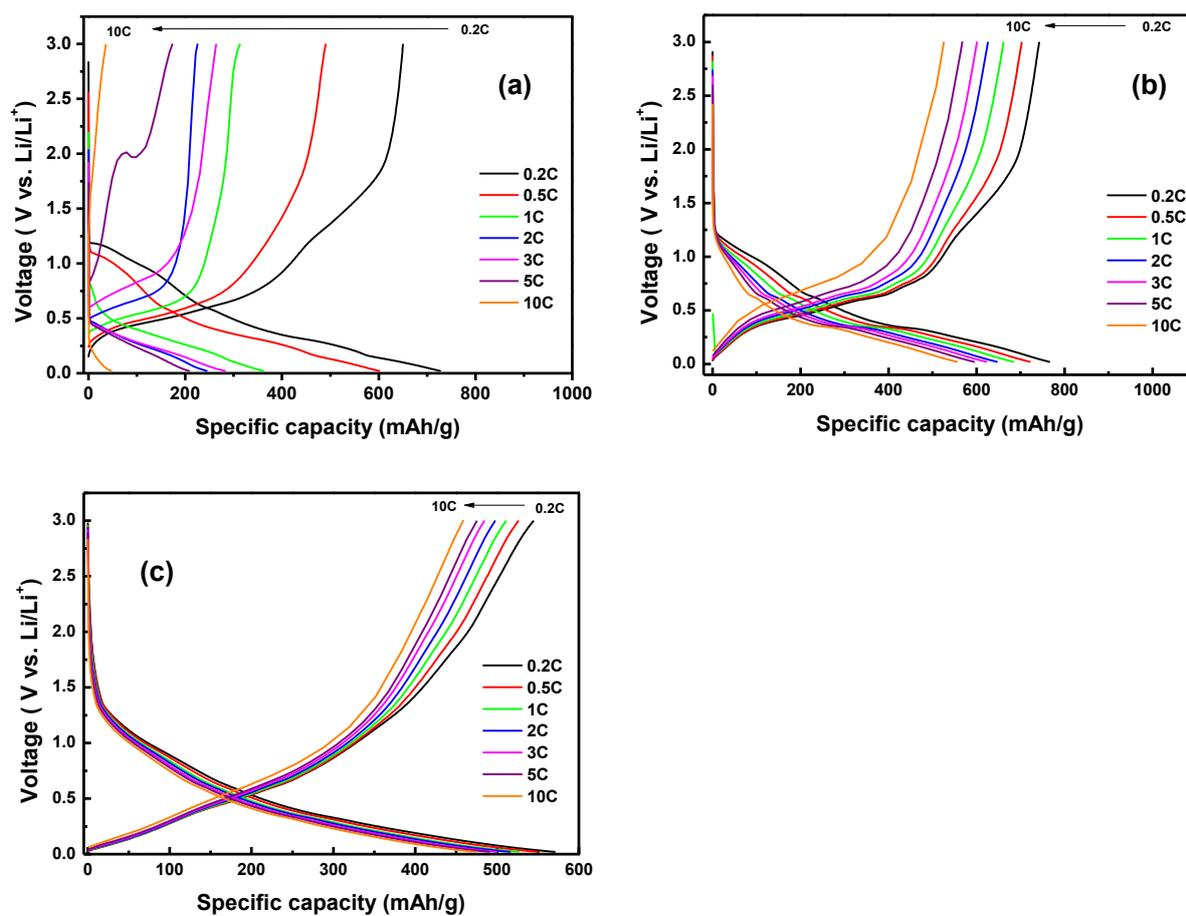
**Figure S7.** Rated curves of the commercial SnO<sub>2</sub> (a), IO SnO<sub>2</sub> (b) and p-IO Sn/SnO<sub>2</sub>/C (c) from 0.2 C to 10 C. All data were obtained after 2cycles with 0.1C charging/discharging rate.
