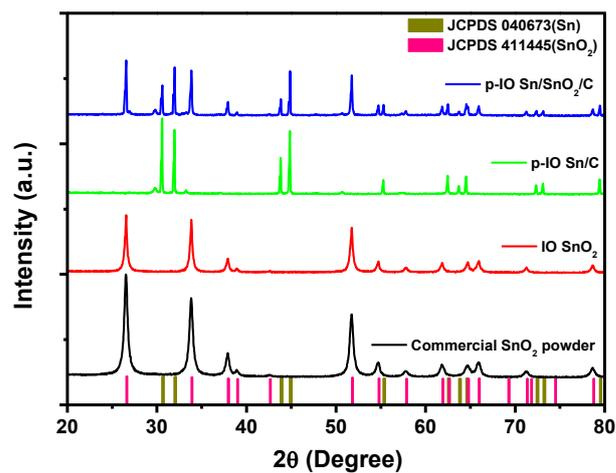
**Figure S5.** XRD patterns of the commercial SnO<sub>2</sub> nanoparticles, IO SnO<sub>2</sub>, p-IO Sn/C, and p-IO Sn/SnO<sub>2</sub>/C.
