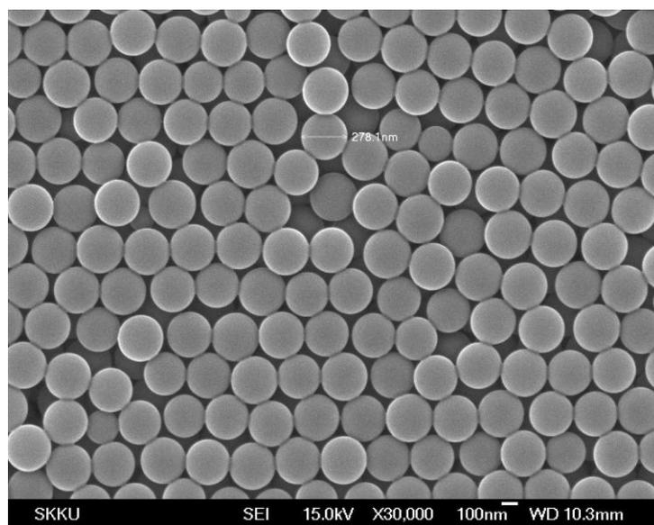
**Figure S2.** SEM image of PS nanobeads.
