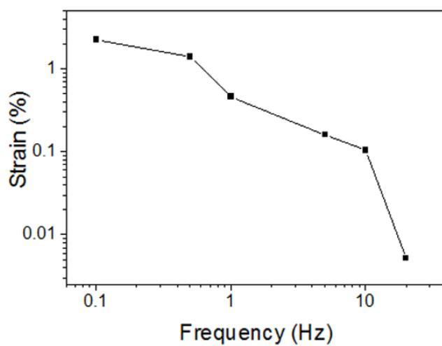
Figure S4. Actuation strain of sG paper as a function of frequency of the applied 10V square voltage.
