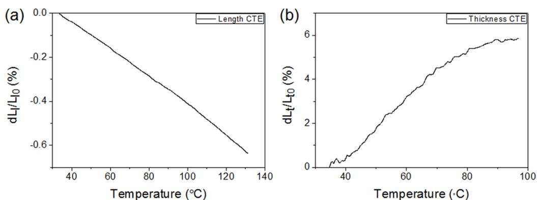
Figure S5. Thermal expansion curves of the sG paper along its length direction (a) and thickness direction (b) measured by TMA with a preload of 5mN.
