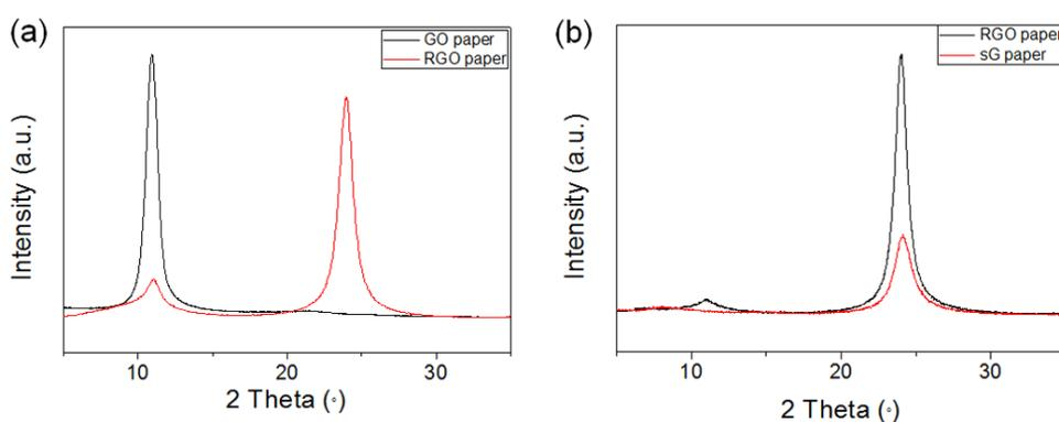
Figure S2. (a) XRD patterns of the GO paper and RGO paper. (b) XRD patterns of RGO paper and subsequently fabricated sG paper.
