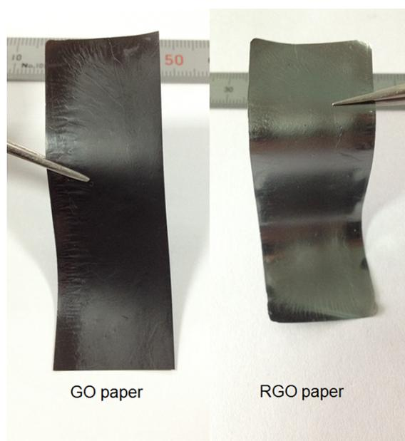
Figure S1. Optical images of GO paper (left) and RGO paper (right).
