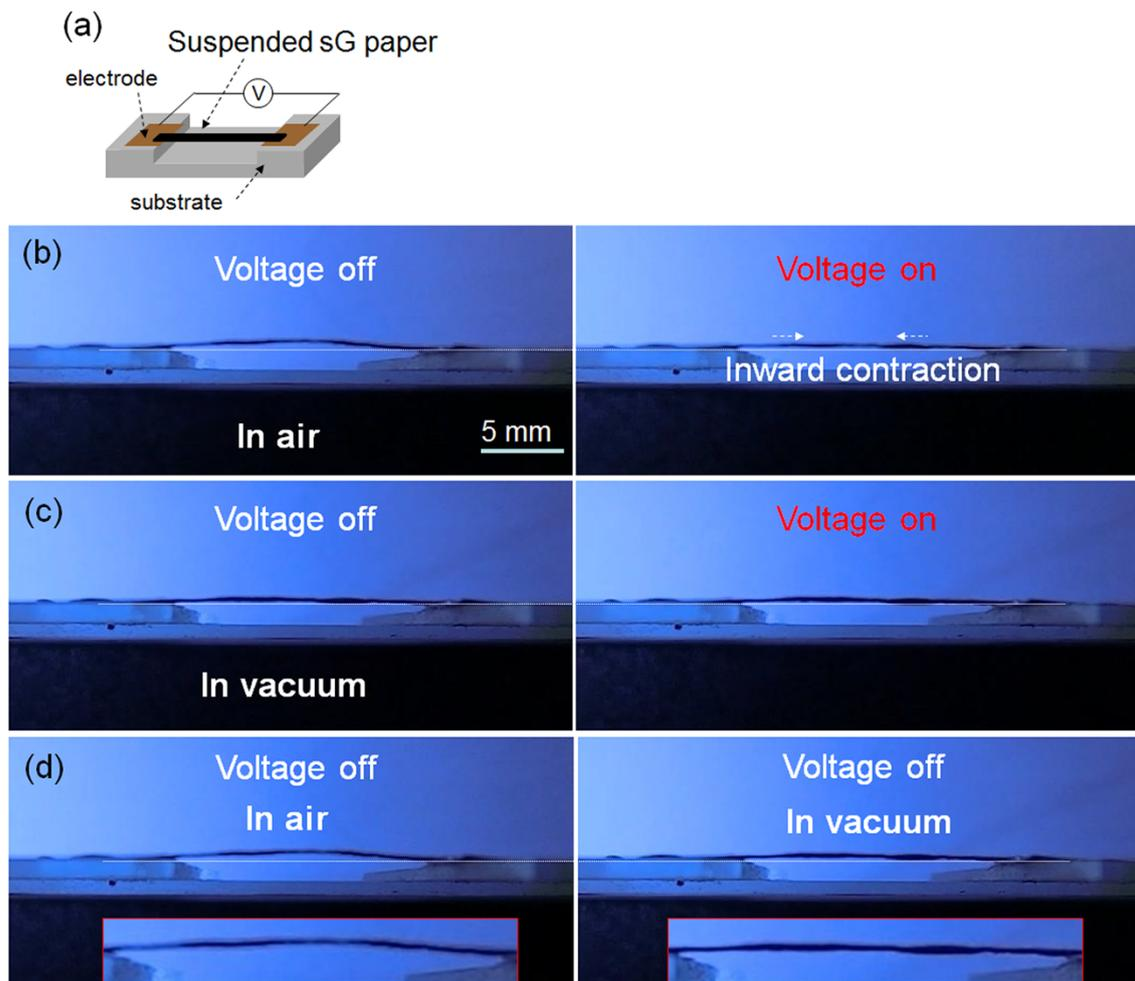
Figure S6. (a) Schematic illustration of the suspended sG paper strip upon electric stimulation. (b-c) Side view optical images of the suspended sG strip with the 0.1Hz 5V voltage off and on both in air (b) and in vacuum (c). Electric induced length contraction of the sG strip can be clearly observed in air.(d) Optical images of the suspended sG strip in air as well as in vacuum without voltage stimulation. The inset images in the red rectangles are the magnification of the suspended sG paper.
