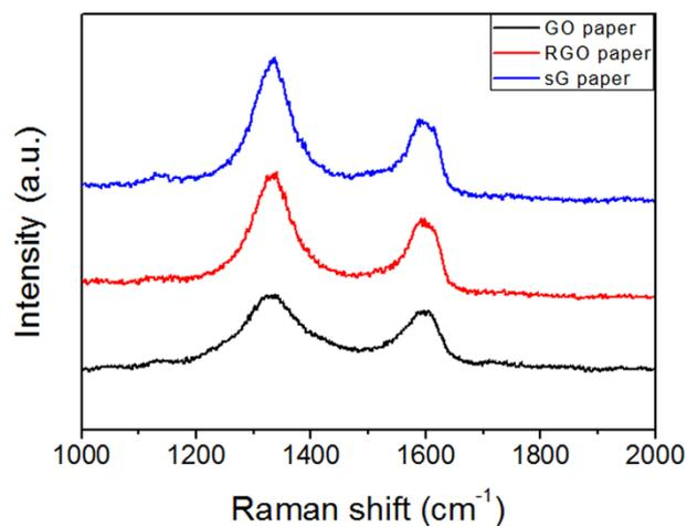
Figure S3. Raman spectra of the GO paper, RGO paper and sG paper.
