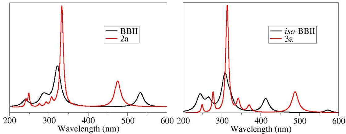
**Fig. S6** Calculated UV-vis spectra of BBII and 2a (left), *iso*-BBII and 3a (right).
