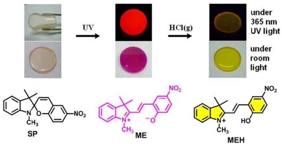
Figure S1. Color and fluorescence changes of a spiropyran-embedded PDMS film in response to UV and HCl(g).
