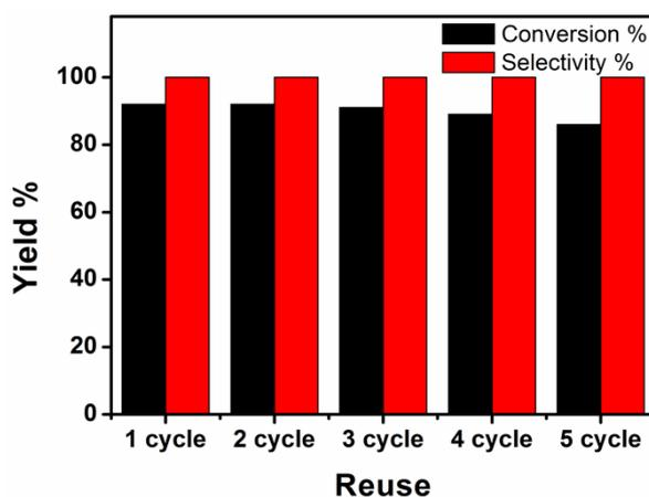
**Figure S7.** Reusability testing results of the NBG/CNTs (5:1) carboncatalyst. Reaction condition: acetonitrile (5 mL), substrate (1 mmol), catalyst (30 mg), O<sub>2</sub> balloon (1 atm), 3 h, 85°C.
