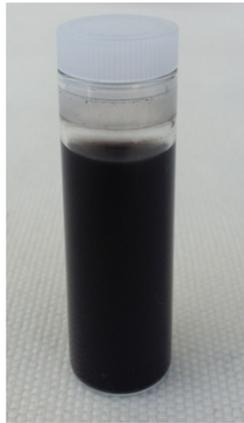
**Figure S3.** Photo of the NBG colloid solution after 24 h, (2 mg NBG was dispersed in 10 mL water), indicating the colloid is extremely stable.
