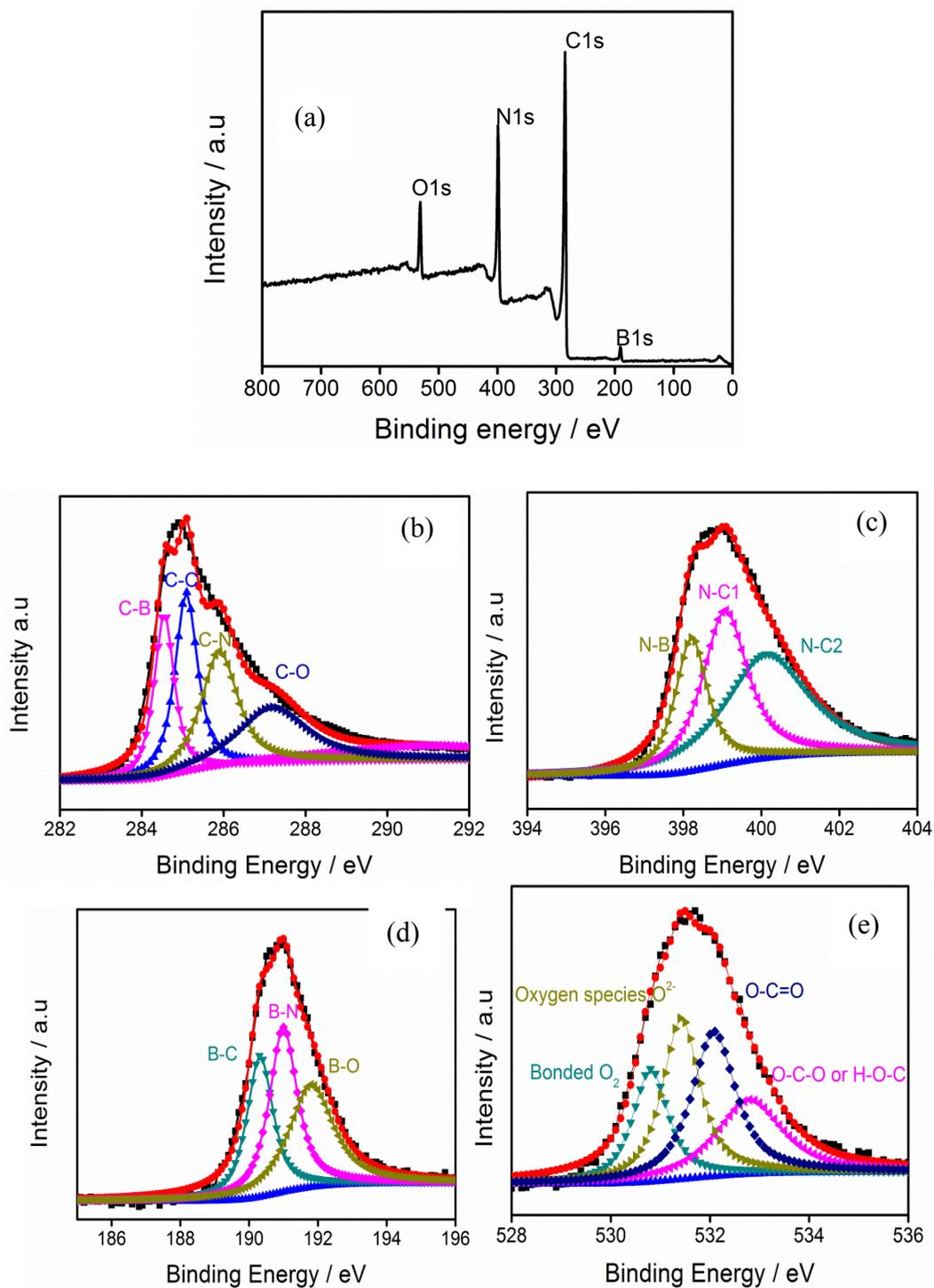
**Figure S1.** (a) The whole XPS spectra of NBG sample. (b) C1s spectra, (c) N1s spectra, (d) B1s spectra, and (e) O1s spectra of NBG.
