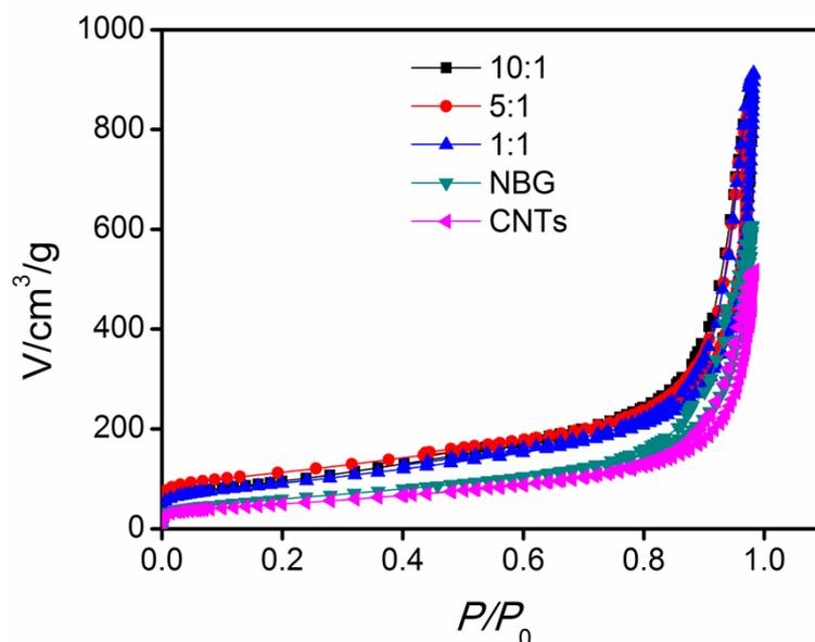
**Figure S5.** N<sub>2</sub> sorption isotherms of pure NBG, NBG/CNTs (10:1), NBG/CNTs (5:1), NBG/CNTs (1:1), and pure CNTs, respectively.
