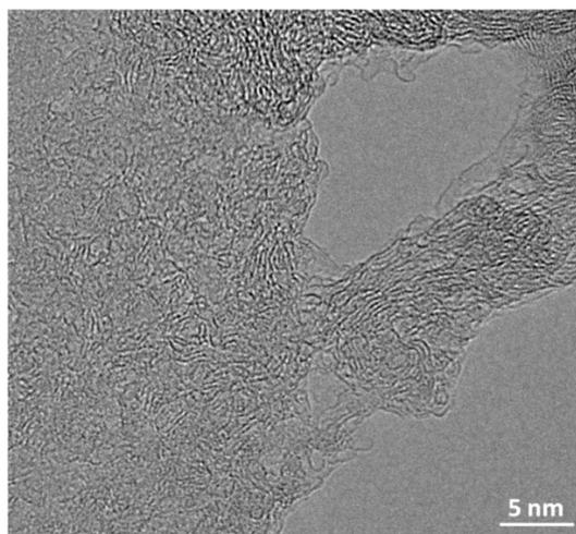
**Figure S4.** Holes were generated by the irradiation of the electron beam during HRTEM observation, indicating the super-thin carbon structure is formed.
