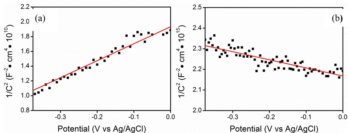
**Figure S6.** (a) Mott-Schottky plot of the pristine CNTs sample and (b) N, B-codoped graphene sample obtained in 1M NaOH solution using a three-electrode photoelectrochemical cell.
