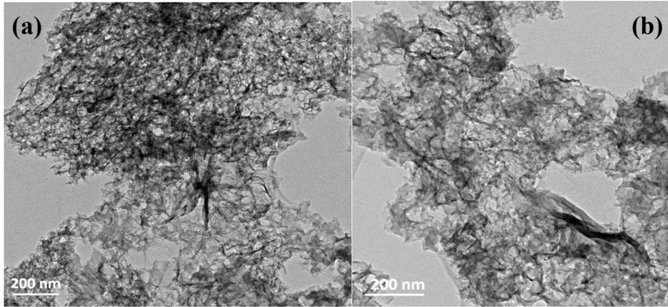
**Figure S2.** HRTEM images of NBG. Many nanopores can be clearly seen from the NBG planes.
