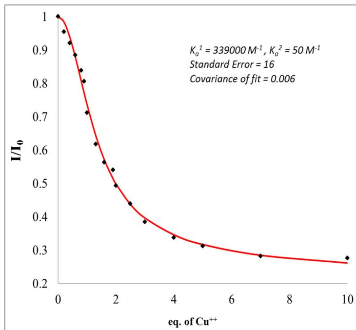
**Figure S2.** Fluorescence quenching response of BNP to the increments of Cu<sup>2+</sup> equivalent in solution. Association constants,  $K_a^1$  and  $K_a^2$ , were calculated by using MATLAB® m-files and fitted for 2:1 BNP: Cu<sup>2+</sup> binding isotherm (Thodarson, P., *Chem. Soc. Rev.* **2011**, *40*, 1305–1323). Experimental data points, (black markers) and fitting curve (red line) for such equilibrium are reported in figures here together with standard error and covariance of fit.
