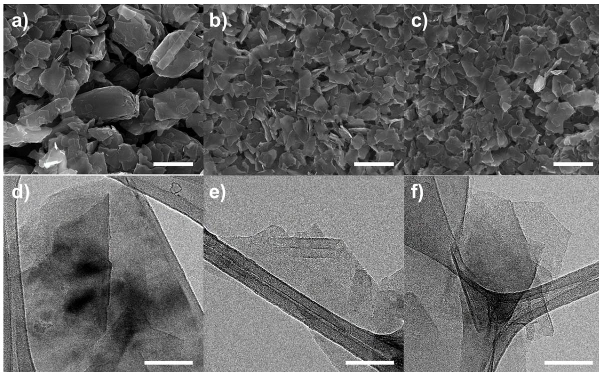
**Figure S1.** Low-magnification SEM image: a) pristine graphite, b) MAG, and c) MIG. Scale bars are 2  $\mu\text{m}$ . Low-magnification HR-TEM images: d) pristine graphite, e) MAG, and f) MIG. Scale bars are 100 nm.
