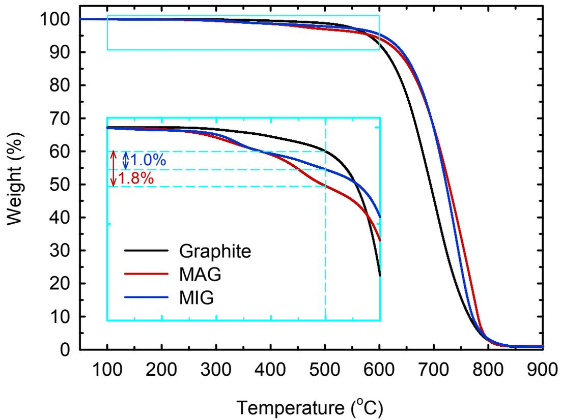
**Figure S2.** TGA thermograms obtained from the heating rate of 10 °C min<sup>-1</sup> in air.
